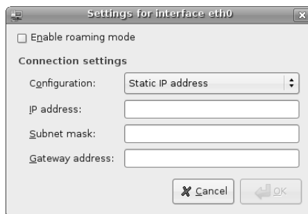
Figure 4-2: Manually inputting network IP settings
