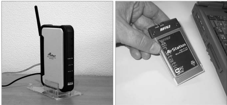
Figure 4-3: All you need for a WiFi setup—an access point and a network interface card
