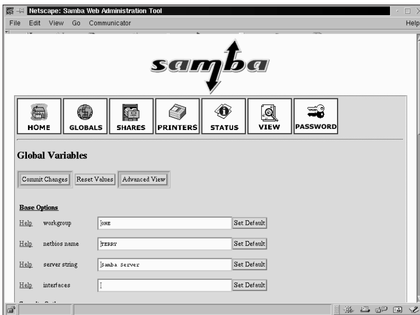
Figure 9-5: The global variables page makes it easy to configure the [globals] section of the smb.conf file.
