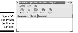
3. Click the New button in the main Printer Configuration tool window.
