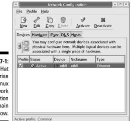
Figure 7-1: The Red Hat Enterprise Linux Network Configuration tool main window.
