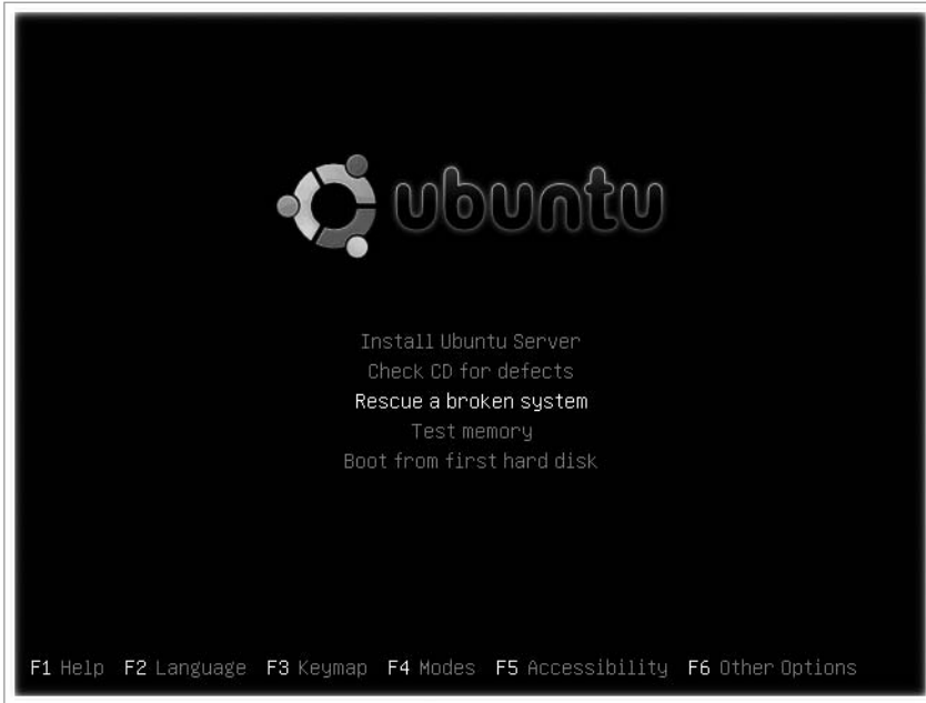
Figure 14-7. On the Ubuntu Server installation CD, you'll find an option to rescue a broken system.
