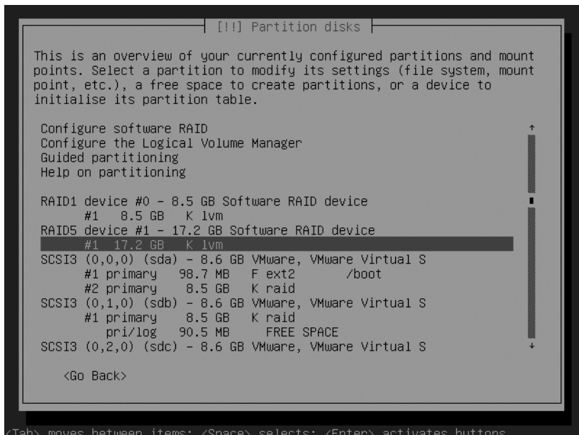
Figure 1-13. Before you start to create logical volumes, your Partition Disks interface should look similar to this.
