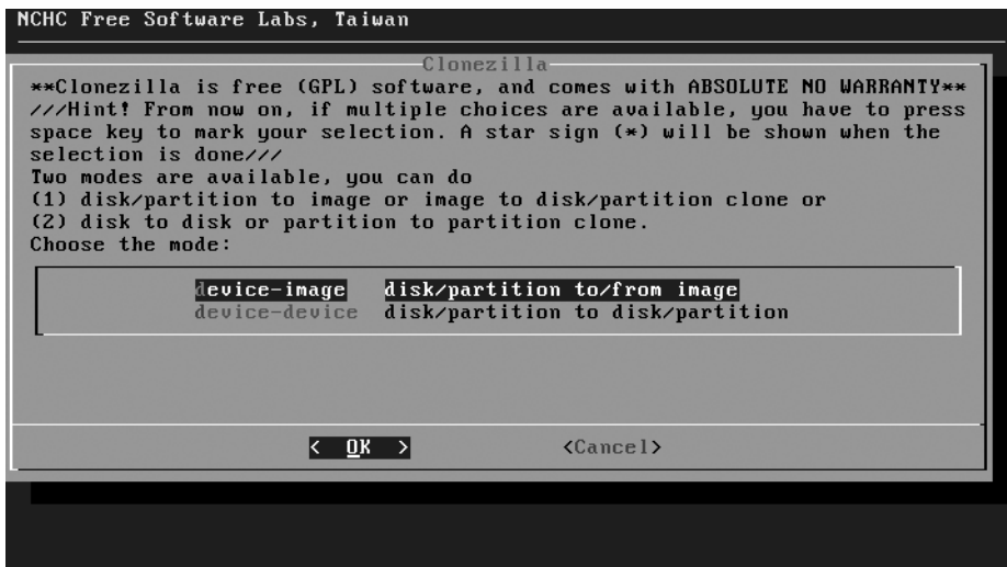
Figure 2-6. Use the device-image option to write the cloned disk to an image file on the Clonezilla server.
