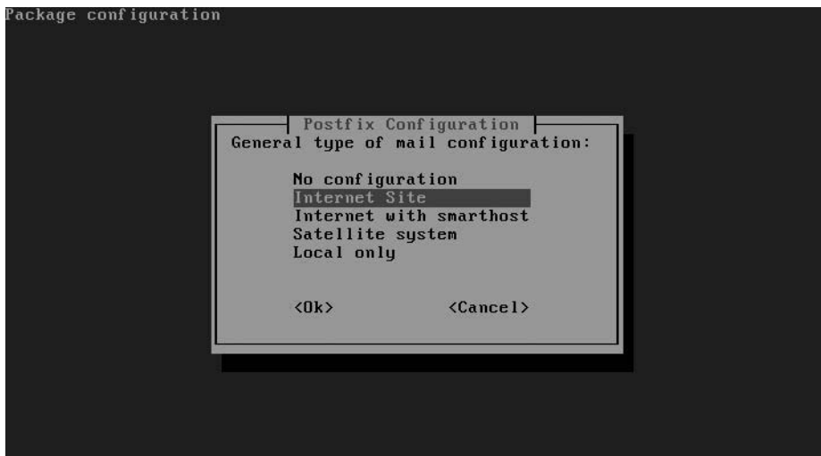
Figure 10-5. To make configuring Postfix easier, the configuration program asks you what kind of mail server you are configuring.
