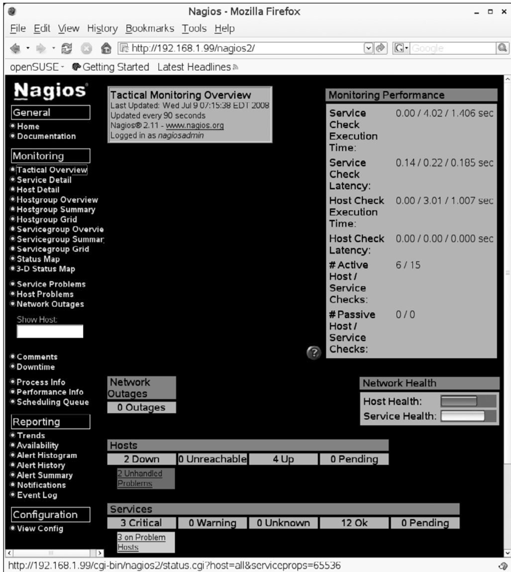
Figure 6-2. The Tactical Monitor Overview window shows you in one view what critical events have happened on your network recently.
