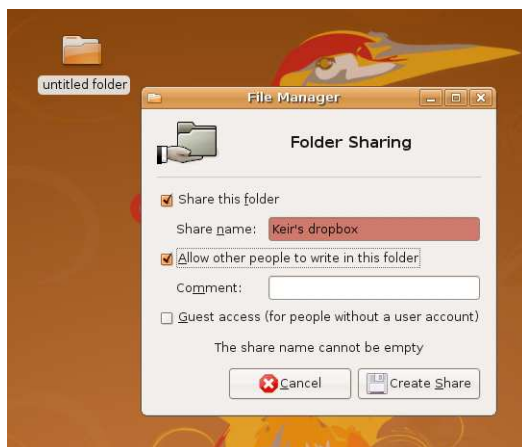
Figure 3.6: The sharing dialog box might report an error, but this is a bug (see Tip 28).
