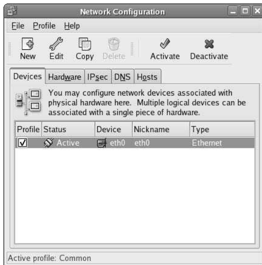
Figure 19-1: The system-config-network tool used by Fedora Core and Red Hat Enterprise Linux.
