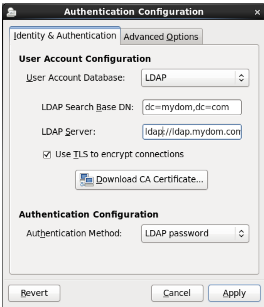
Figure 21.3 Authentication Configuration Using LDAP
