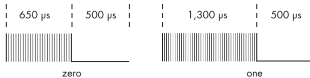
Figure 12-3: Modulated pulses in the Sony TV protocol
