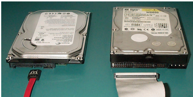
FIGURE 4.2 SATA (left) features much slimmer connecting cables than the older PATA (right).
