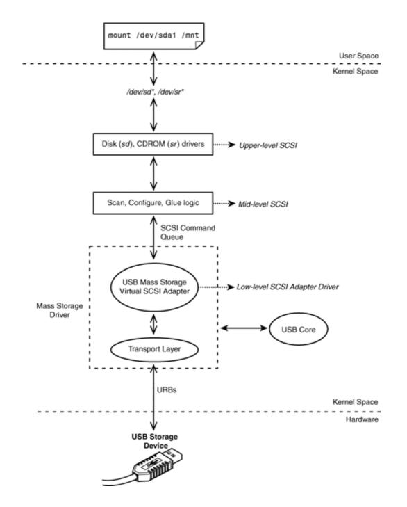
The mass storage driver registers itself as a virtual SCSI adapter. The virtual adapter communicates upstream via SCSI commands and downstream using URBs. A USB disk appears to higher layers as a SCSI device attached to this virtual adapter.
