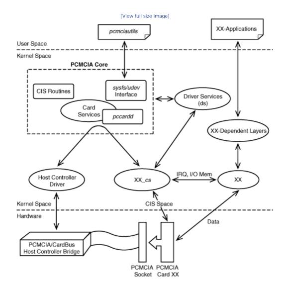
Figure 9.3. The Linux-PCMCIA subsystem.
