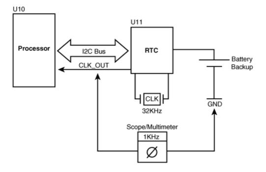
Figure 18.4. Debugging an I<sup>2</sup>C RTC on an embedded system.
