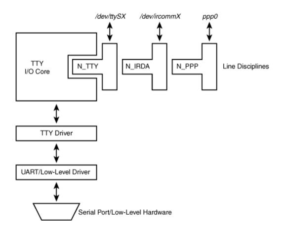
Figure 6.3. Serial layers mapped to kernel sources.
