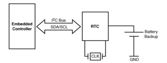
Figure 8.3. An I<sup>2</sup>C RTC on an embedded system.
