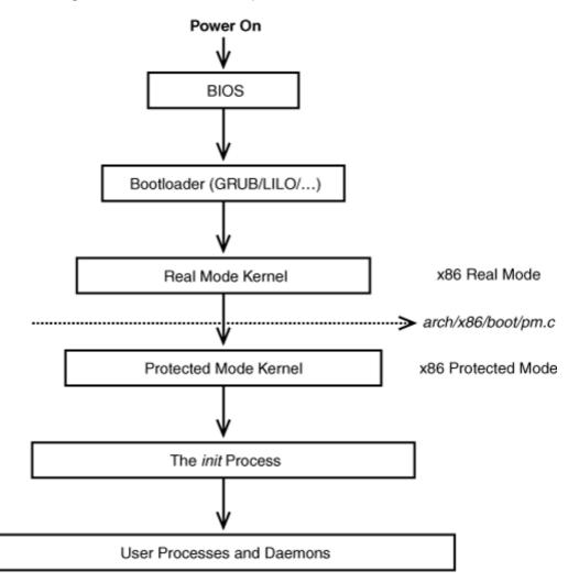
Figure 2.1. Linux boot sequence on x86-based hardware.
