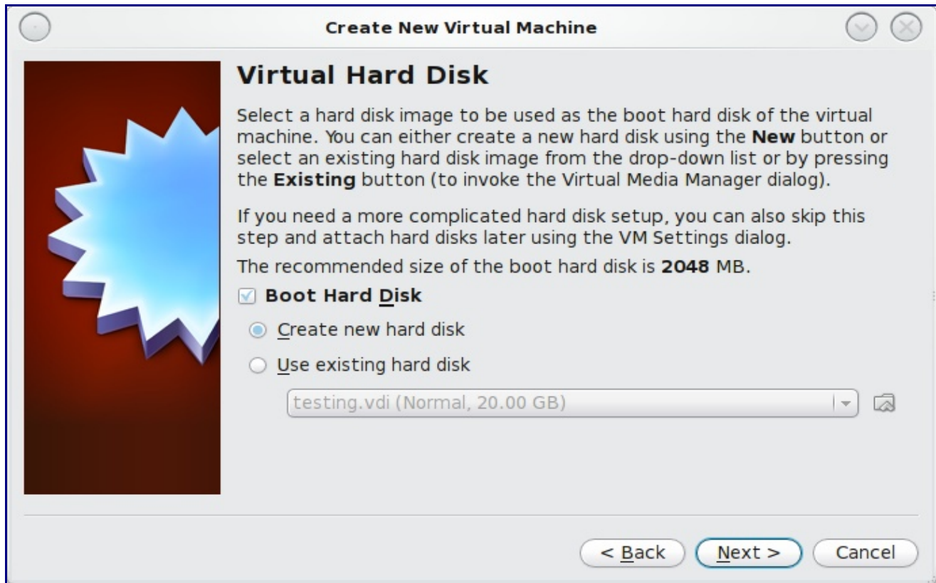
Figure 2.8.1c: Select Whether to Use an Existing or Create a New Virtual Disk
