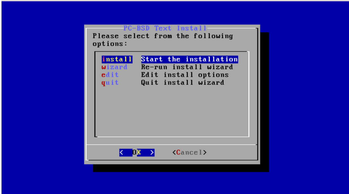
Figure 5.1f: Review Installation Options
