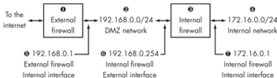
This sort of firewall setup is used whenever servers need different stages of protection. The **1** external firewall provides the outermost layer of protection. Any traffic coming in through the Internet hits this firewall first, and any traffic leaving the network goes through this firewall last. This firewall probably has fairly liberal traffic-management rules.
