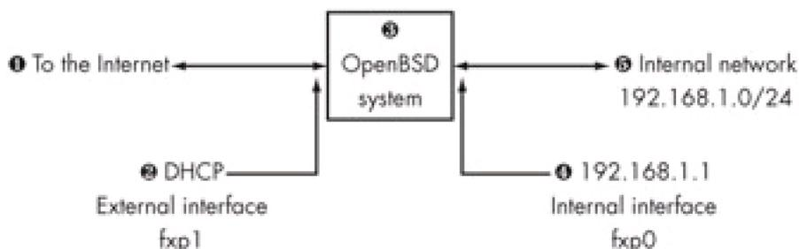
Here, we have an **3** OpenBSD machine attached to the **1** public Internet via a **2** DHCP connection. Our internal network is on the private IP addresses **5** 192.168.0.0/24, routing through the **4** default gateway of 192.168.1.1. We don't want anyone to come in from the outside world normally, but we will leave port 22 open so we can SSH to home from other locations.
