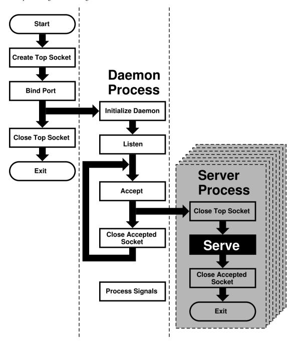
We moved the *serve* from the *daemon process* to its own *server process*. However, because each child process inherits all open files (and a socket is treated just like a file), the new process inherits not only the "accepted"
