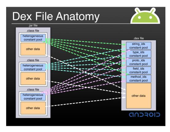
Figure 3.1: .dex file structure. Constant pools from classes get merged into one corresponded .dex file pool. From [17].
