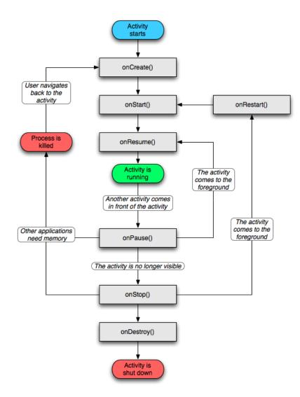
Figure 2.1: Life cycle graph of an *Activity*. The graph for a *Service* is similar. From [22, Application Fundamentals].
