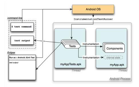
Figure 6.3: Instrumentation framework structure with it's different components onand off-site the device. From [22, Testing and Instrumentation].
