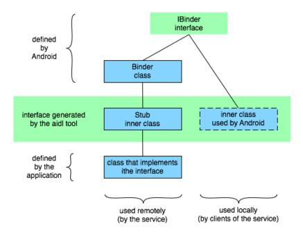
Figure 2.2: Android RPC class diagram showing the user space design of the mechanism. From [22, Application Fundamentals].
