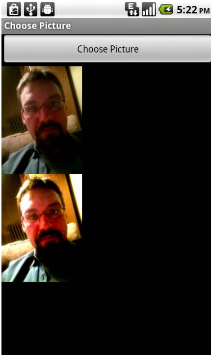
Figure 3–16. ColorMatrix with each color's intensity doubled but brightness decreased to affect contrast without changing brightness
