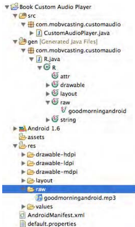
Figure 5–2. Custom audio player Eclipse Project layout showing audio file located in raw folder inside res folder.
