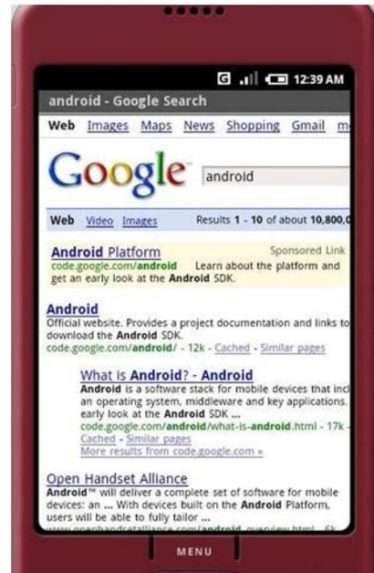
**Figure 1.2** Android’s built-in browser technology is based on WebKit’s browser engine.
