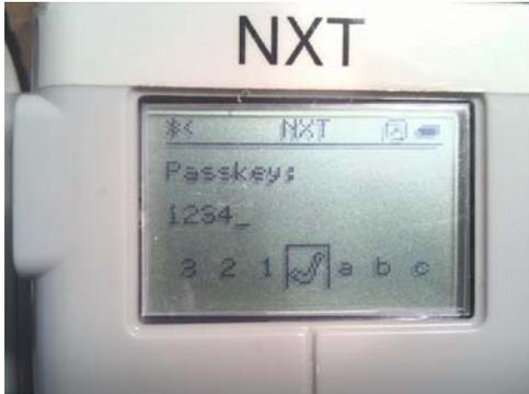
**Figure 14.3** LEGO controller prompts for a PIN
