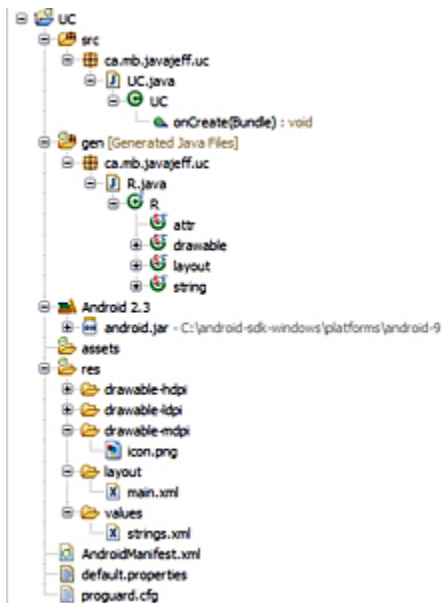
Figure 1-18. Additional + icons have been clicked to reveal more of UC's file organization.
