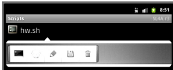
Figure A-4. The icon menu lets you run a script in a terminal window, run a script in the background, edit the script, rename the script, or delete the script.
