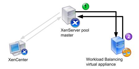
This illustration shows how (1) XenServer communicates with Workload Balancing using an account you created during Workload Balancing Configuration and (2) the Workload Balancing virtual appliance authenticates to XenServer using the credentials for the pool.
