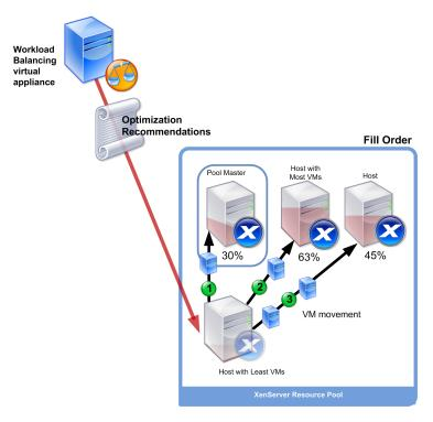
This illustration shows how, when consolidating VMs on hosts in Maximum Density mode, XenServer attempts to fill the pool master first, the most loaded host second, and the least loaded host third.
