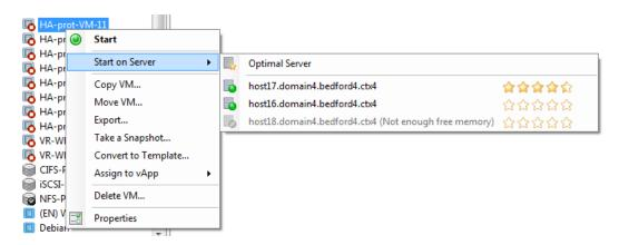
This illustration shows a screen capture of the Start On Server feature. More stars appear beside host17 since this is the optimal host on which to start the VM. host16 does not have any stars beside it, which indicates that host is not recommended. However, since host16 is enabled the user can select it. host18 is greyed out due to insufficient memory, so the user cannot select it.
