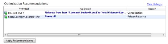
This illustration shows a screen capture of the Optimization Recommendations list, which appears on the WLB tab. The Operation column displays the behavior change suggested for that optimization recommendation. The Reason column displays the purpose of the recommendation. This screen capture shows an optimization recommendation for a virtual machine, HA-prot-VM-7, and a host, host17.domain4.bedford4.ctx4.
