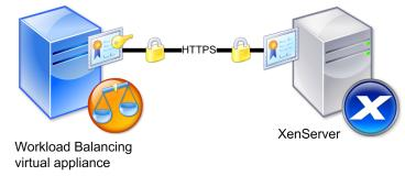
This illustration shows how XenServer verifies that a specific certificate is present before it lets the Workload Balancing virtual appliance establish a connection to it over SSL. In this case, the real certificate (the certificate with the private key) is on the Workload Balancing server and the certificate that was used to sign it, is on the XenServer pool master.
