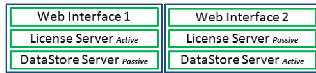
Figure 23 - Hardened Services Module
