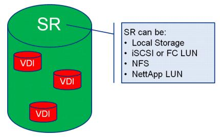
A key object in XenServer storage is a Storage Repository (SR). This is the physical on-disk structure or format imposed on the available physical storage by XenServer. XenServer allocates Virtual Disk Images (VDI) on an SR, which is what a VM sees as a physical disk.
