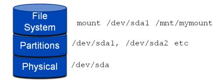
Because the storage access is through the Control Domain, it is worth revising what we know about Linux and how it views disk storage. In Linux, typically the physical disk itself is split into partitions. Remember that all devices in Linux are accessed through device files.
