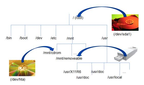
The Linux file system gives you a unified view of all storage and has a single root directory, indicated by a forward slash (/). Within the root directory is a hierarchy of files and directories. Parts of the file system can reside on different physical media, such as hard disks, flash disks, and CD-ROMs. If you are familiar with MS-DOS or Windows, note that you will not find drive letters in Linux. All disk drives and CD-ROM drives are part of a single file system hierarchy.
