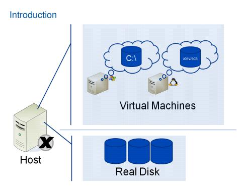
In the virtual world of a XenServer, the virtual machines (VMs) behave like real machines with locally attached disks. In reality, the XenServer host has allocated a chunk of real disk space and, through the hypervisor and Control Domain (Domain 0), has made them available as a disk resource to the VMs.
