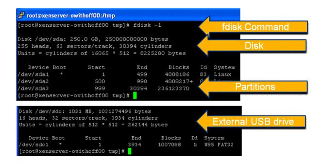
How does Linux let us know which disks it has detected? The **fdisk** command is the partition table manipulator for Linux, but it can be destructive when used improperly. You can, however, use **fdisk** –I to check which disks and partitions on those disks Linux has detected. Remember that you can read the manual pages for Linux commands using the **man** command. For example, **man fdisk**.
