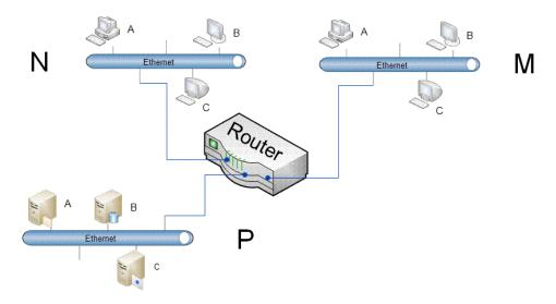
In this example, if node NA wants to send a TCP/IP packet to node PB, what needs to happen?
