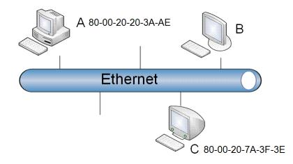
Ethernet defines a frame (not a packet) which is the carrier of the data payload from the upper layers.
