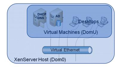
This is a simple picture of how XenServer networking works. Each virtual machine has a virtual NIC, which is connected to a virtual network, which is controlled by the XenServer host: Domain zero.
