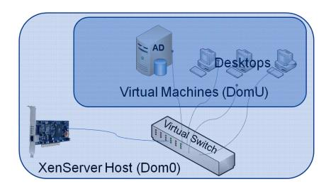
In reality, XenServer networking is accomplished by connecting the VIFs and optionally 1-PIF to a virtual switch or bridge. If you remember, a switch learns the MAC addresses of the nodes connected to each of its ports, thereby reducing the amount of traffic on its other ports. It's the same with a bridge.
