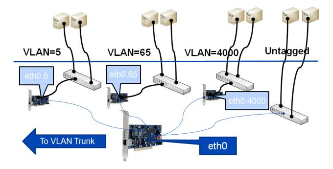
In this example there are 8 virtual machines as guests on a single XenServer host. Also on this host are 3 VLANs, with tags 5, 65 and 4000. There are also a couple of machines that have a regular non-vlan (untagged) external network, so their bridge is wired directly to the PIF.
