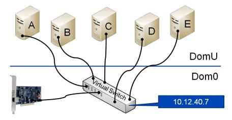
Adding access to the physical NIC on the host turns our *Internal Network* into an *External Network*. The virtual machines communicate as previously described, but now we have a special case – the real ethernet NIC. What happens when we need to transmit a frame from node A, for example, to a node outside of the host?
