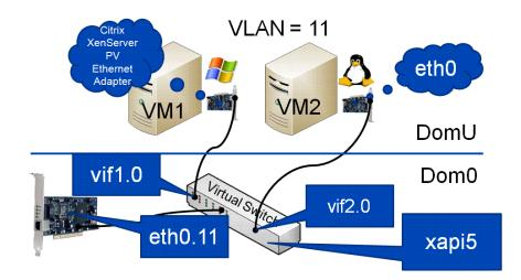
In the case of creating a VLAN, every distinct VLAN will get its own bridge. Also, the (pseudo) PIF will have a dot separated name to include the vlan tag number and, when on the real network, the bridge name will start with "xapi". Apart from that, everything else will be the same as normal external network. It's not possible to create an internal VLAN network.
