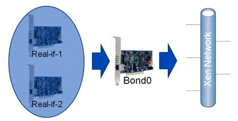
NIC bonds can improve XenServer Host resiliency by using two physical NICs as if they were one. If one NIC within the bond fails the host's network traffic will automatically be routed over the second NIC. In XenServer 4.1, NIC bonds work in an active/passive mode, with only one physical NIC ever in use.
