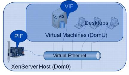
In the Unix world, the NICs, real or virtual, are called interfaces. XenServer calls a real interface a Physical Interface or PIF and each virtual interface in a virtual machine is a VIF.
