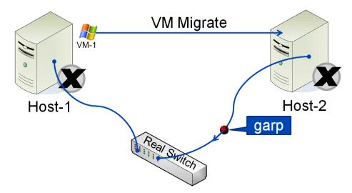
But in this example setup, the external real switch device is expecting the MAC address of the VM to be on one port, while it's actually just migrated to another port. In this case, the last step of the migration is for the destination host to update any external devices with a gratuitous ARP packet. A "garp", is nothing more than a regular ARP request, but with the MAC and IP address already filled-in. This serves as an update to any external devices' arp cache, and there would be no response.
