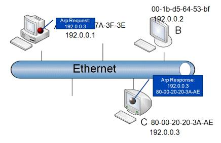
Layer 3 of the 7-layer OSI defines a network addressing scheme, most commonly the Internet Protocol (IPv4). Here both nodes A and C have been given unique IP addresses. Although not obvious here, we haven't just replaced one addressing scheme with another. IP can route packets from one node in one Ethernet segment to another node in another segment across the world.
