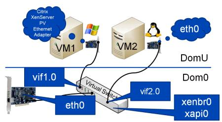
Each virtual machine has a unique ID, and in the above example the Windows VM has an ID of 1, and the Linux VM has an ID of 2.
