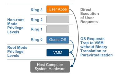
paravirtualization. The guest state is stored in Virtual Machine Control Structures (VT-x) or Virtual Machine Control Blocks (AMD-V).
