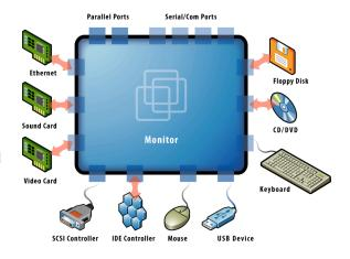
Figure 9 – Device and I/O virtualization
