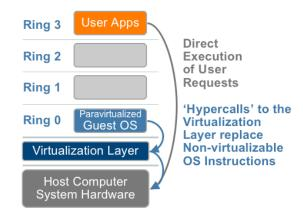
Figure 6 – The Paravirtualization approach to x86 Virtualization
