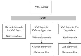
Figure 11 – Transparent paravirtualization with the Virtual Machine Interface (VMI)
