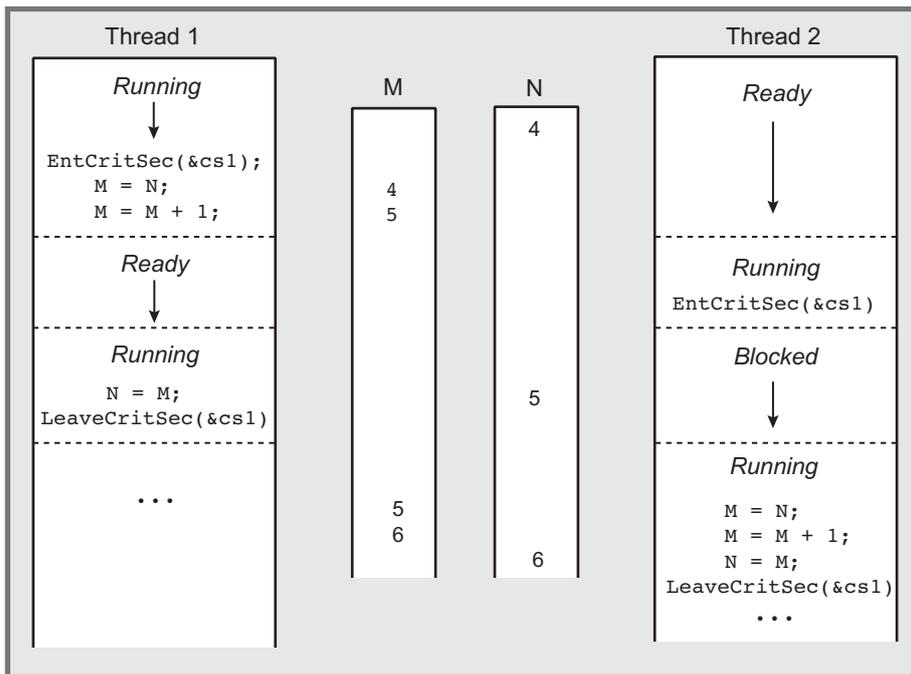
**Figure 8–3** Synchronized Threads Sharing Memory
