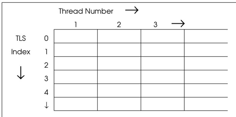
**Figure 7-3** Thread Local Storage within a Process
