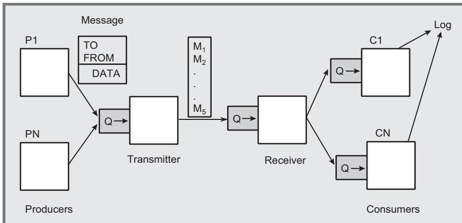
**Figure 10–1** Multistage Pipeline
