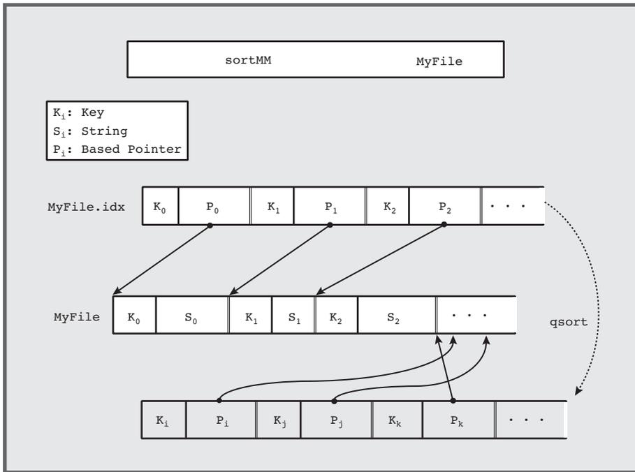
**Figure 5-5** Sorting with a Memory-Mapped Index File
