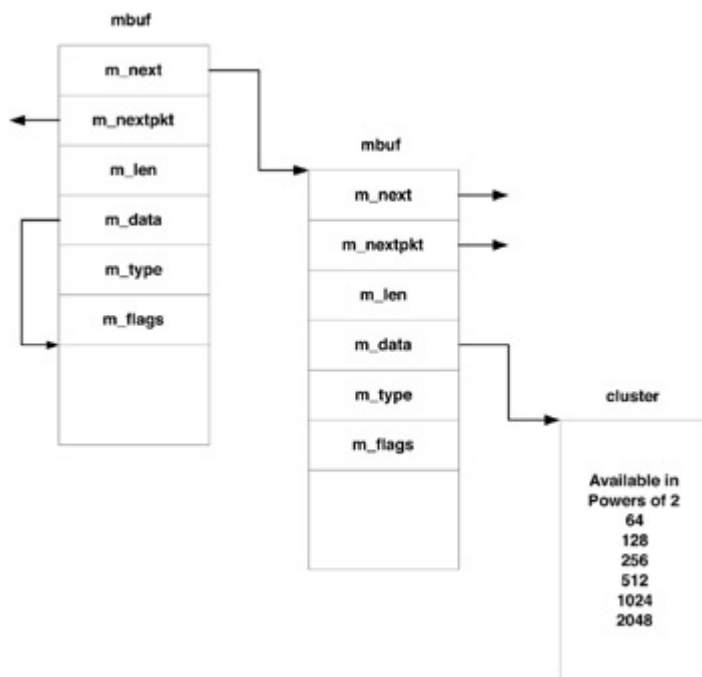
Figure 7.3: Berkeley mbuf structure.
