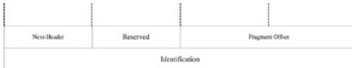
Figure 11.2: The fragmentation header.
