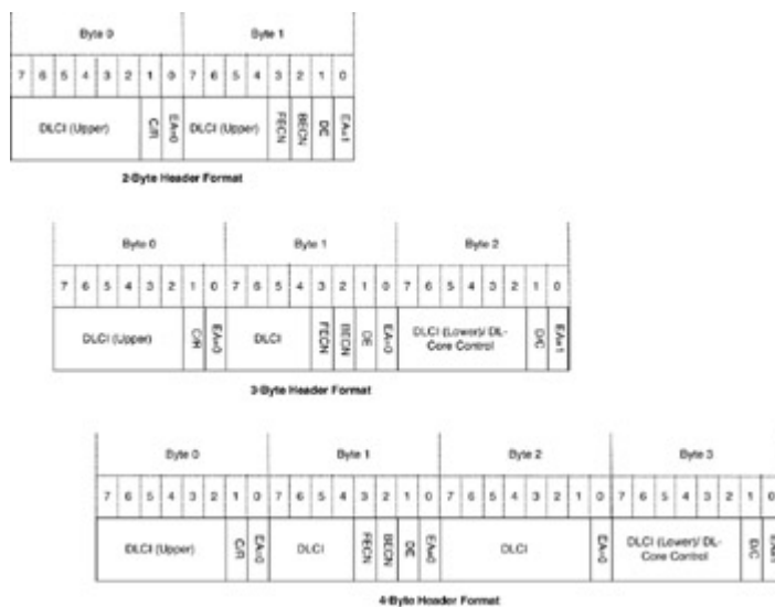
Figure 2.5: Frame Relay header formats.
