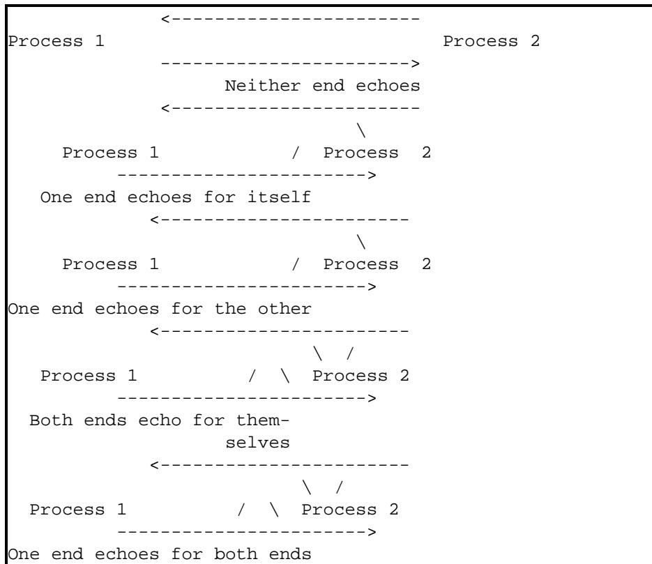
This option provides the capability to decide whether either end will echo for the other. It does not, however, provide any control over whether an end echoes for itself; this decision must be left to the sole discretion of the systems at each end (although they may use information regarding the state of “remote” echoing negotiations in making this decision).
