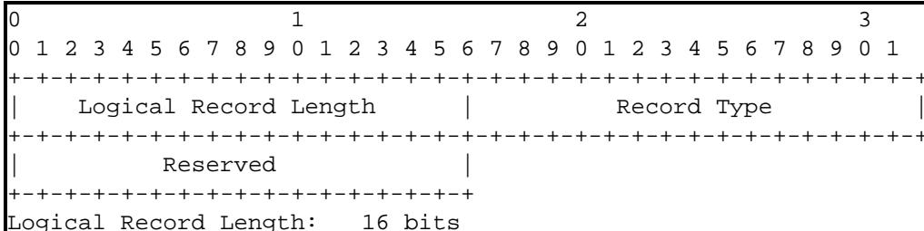
This field indicates the length, in octets, of this logical record including the header length. The length is calculated *before* doubling any IAC characters in the data stream. The length does not include the <IAC><EOR> that is appended to the end of the data stream to mark the end of this logical record. The length is specified with the most significant octet first. For example, a length of 36 (decimals) would be specified as '0024'X.
