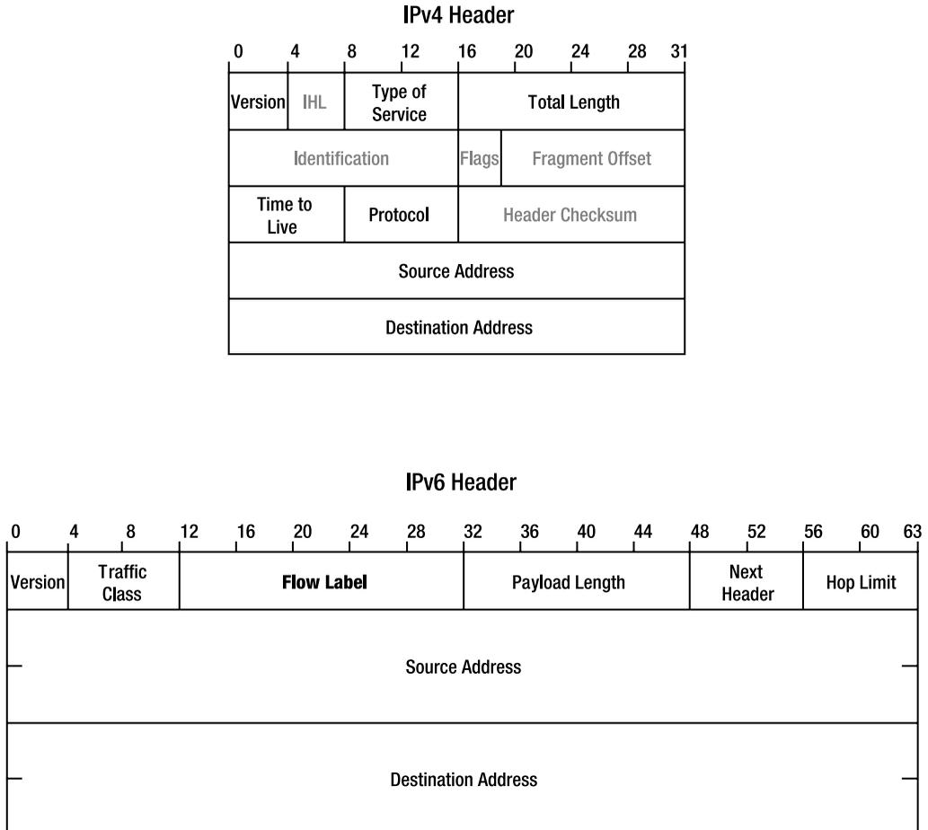
**Figure 8-1.** *The IPv4 and IPv6 headers*
