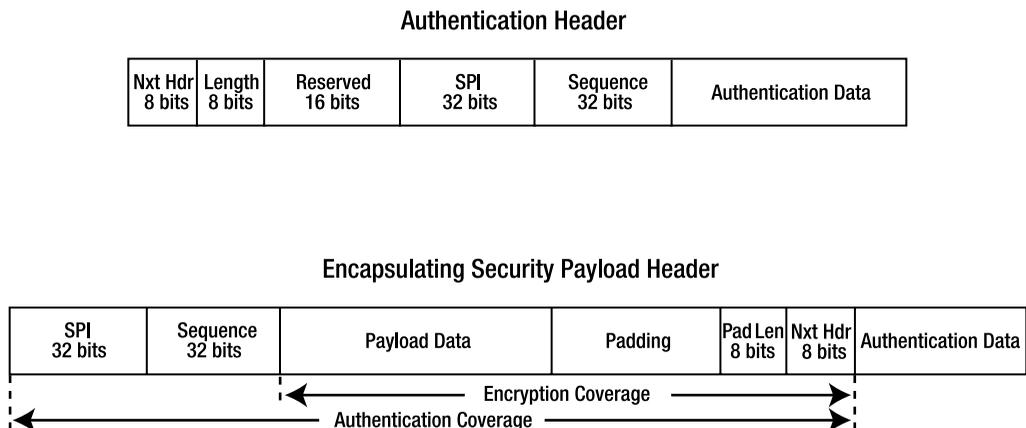
**Figure 9-3.** The AH and ESP header formats
