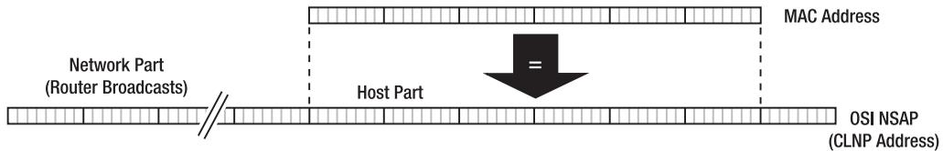
**Figure 1-5.** *The variable length CLNP address and the Ethernet MAC address*
