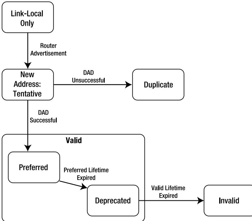
**Figure 8-2.** *The life cycle of an IPv6 address*
