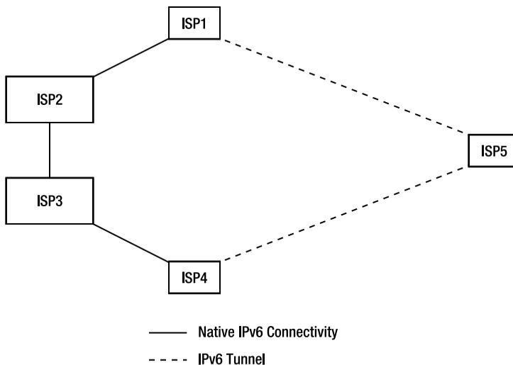
**Figure 4-5.** *Native versus tunneled connectivity in IPv6*
