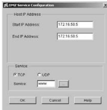
Figure 15.24 shows Advanced Firewall DMZ Service Configuration dialog box with the first service in place. As previously mentioned, you can click Add to configure as many more services as required. By the way, since it is not unusual to have more than one service on a server, the SDM allows you to configure more than one service. You simply configure each one individually.
