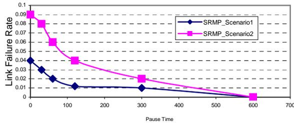
Figure 5.15 SRMP Link Failure Rate (Both Multicast Scenario)
