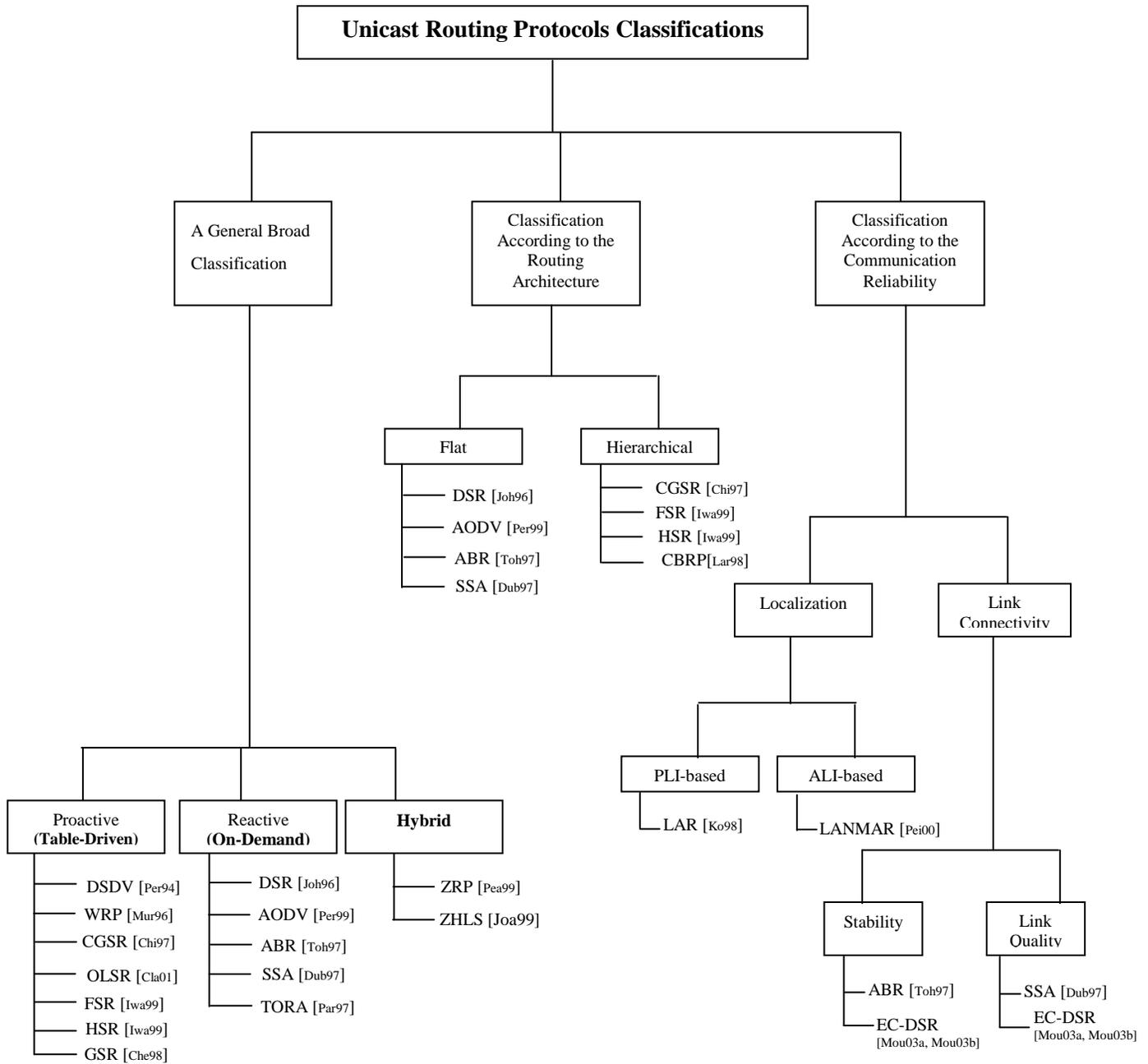
Figure 2.1 Ad hoc Routing Protocols Different Classifications
