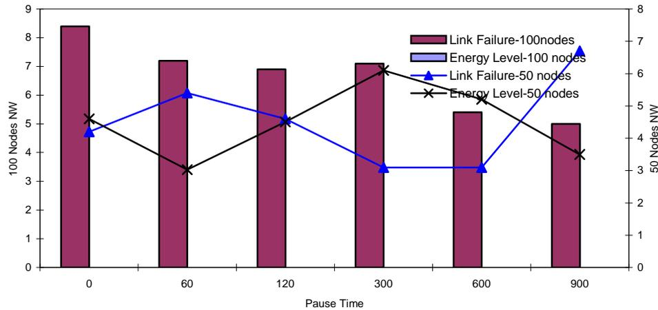
Figure 4.19 PM Energy Level Vs Link Failure
