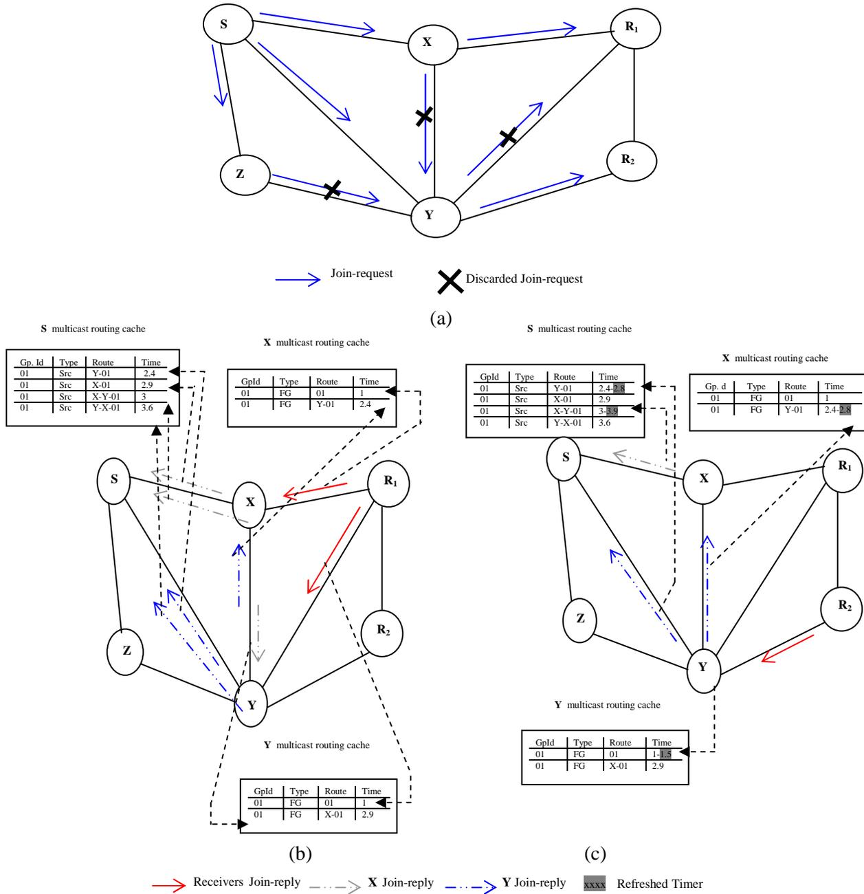
Figure 5.6 : A Small Network Running SRMP: (a) Join-request generation by S, (b) Join-reply generation by R<sub>1</sub> to S, and (c): Join-reply generation by R<sub>2</sub> to S
