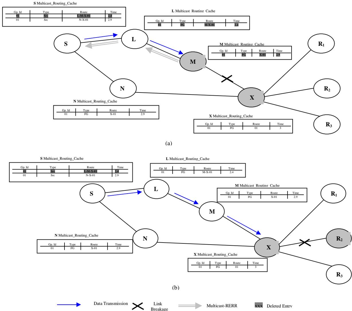
Figure 5.10 Link Failure Examples: (a) Link breakage between two FG Nodes, (b) Breakage Between an FG Node and a Multicast Receive
