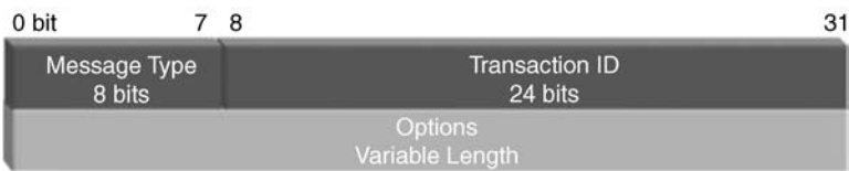
Figure 5.3. DHCPv6 packet format (68).
