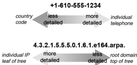
Figure 10.2. Telephone number mapping to domain structure.
