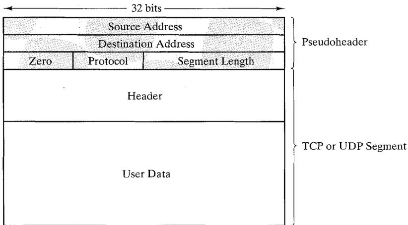
**FIGURE 17.15** Scope of checksum for TCP and UDP.
