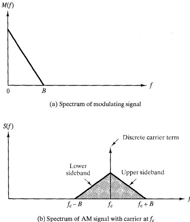
FIGURE 4.19 Spectrum of an AM signal.
