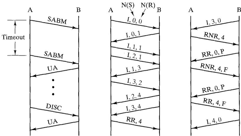
(a) Link setup and disconnect (b) Two-way data exchange (c) Busy condition
