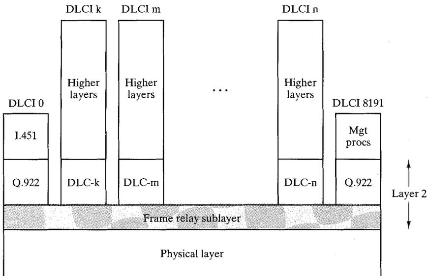
**FIGURE 10.8** Multiplexing at the frame relay sublayer.
