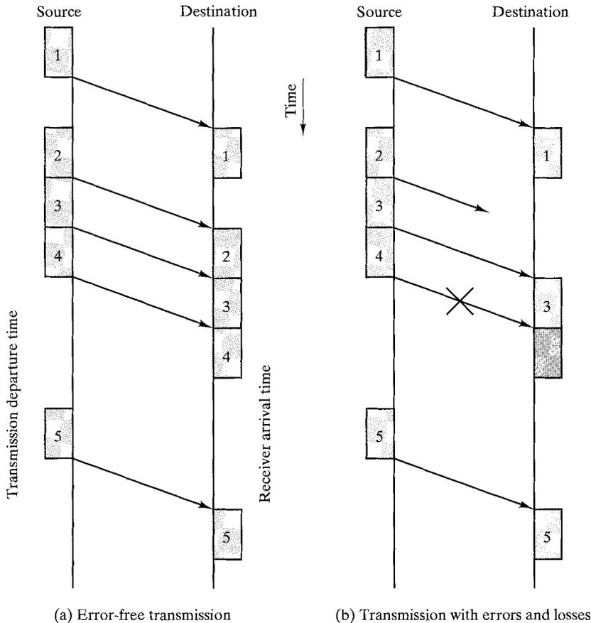
FIGURE 6.1 Model of frame transmission.
