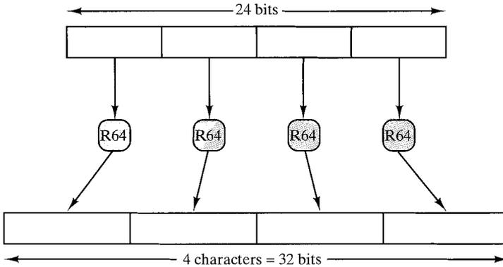
**FIGURE 19.11** Printable encoding of binary data into radix-64 format.
