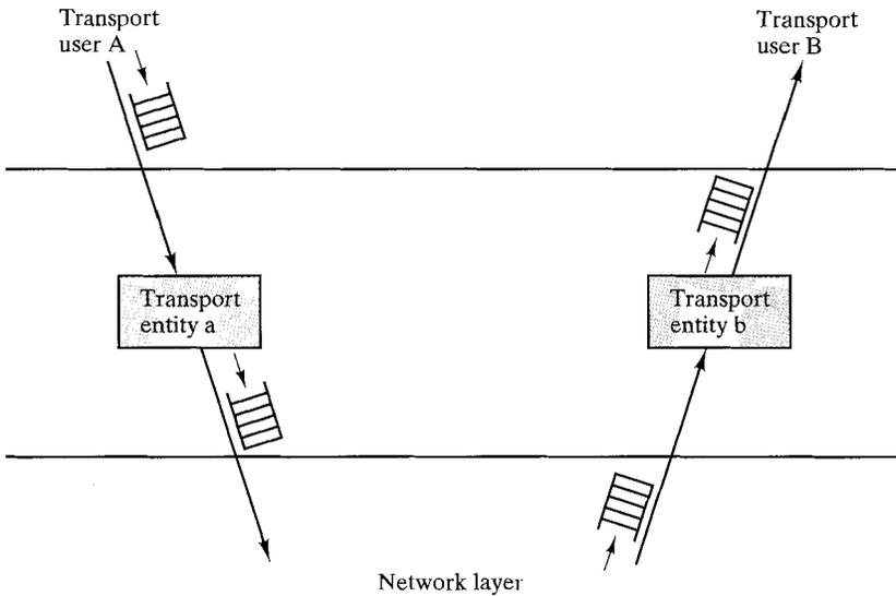
FIGURE 17.3 Queuing representation of connection-oriented data transfer.
