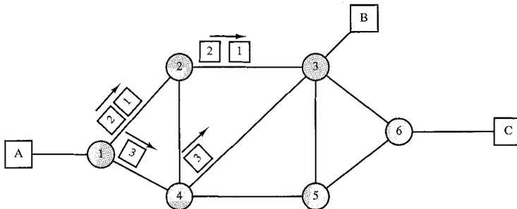
(d) Internal datagram. Each packet is treated independently by the network. Packets are labeled with a destination address and may arrive at the destination node out of sequence.
