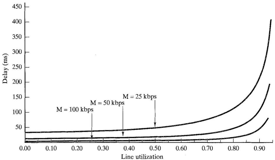
(b) Mean delay versus utilization
