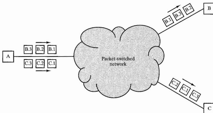
(b) External diagram. Each packet is transmitted independently. Packets are labeled with a destination address and may arrive out of sequence.
