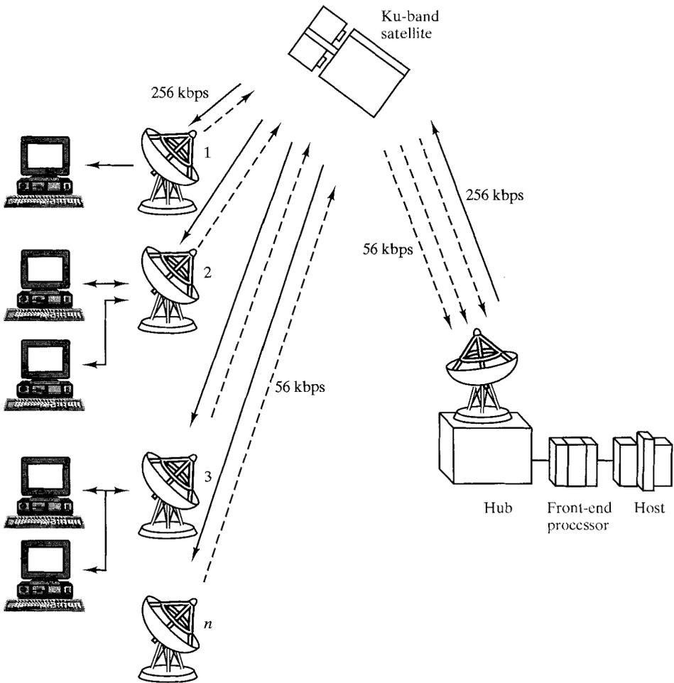
FIGURE 3.5 VSAT configuration.
