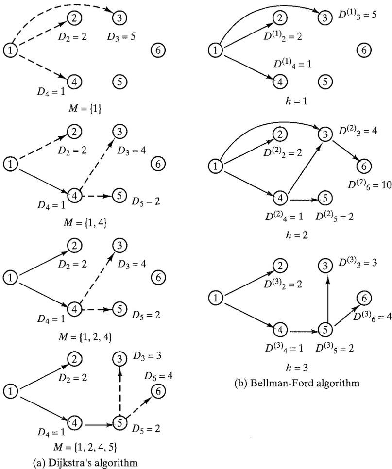
**FIGURE 9.23** Examples of least-cost routing algorithms (based on Table 9.4).
