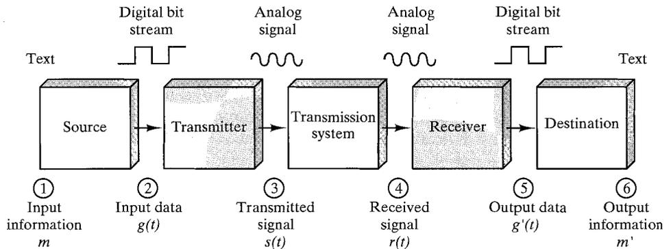
**FIGURE 1.2** Simplified data communications model.
