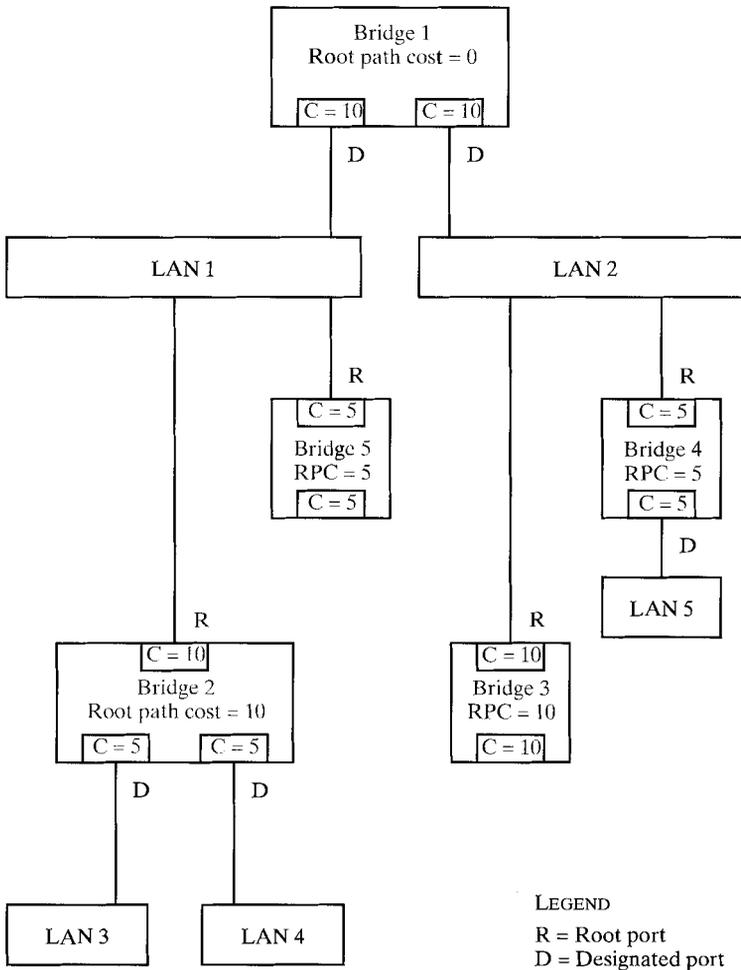
FIGURE 14.11 Spanning tree for configuration of Figure 14.10.
