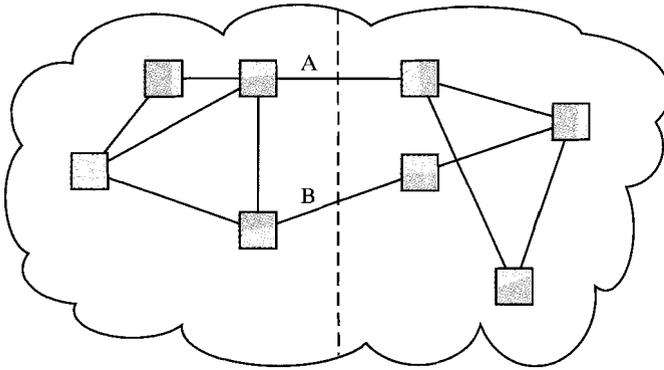
**FIGURE 9.11** Packet-switching network subject to oscillations.
