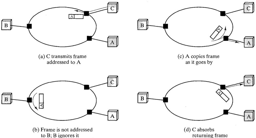
**FIGURE 12.6** Frame transmission on a ring LAN.
