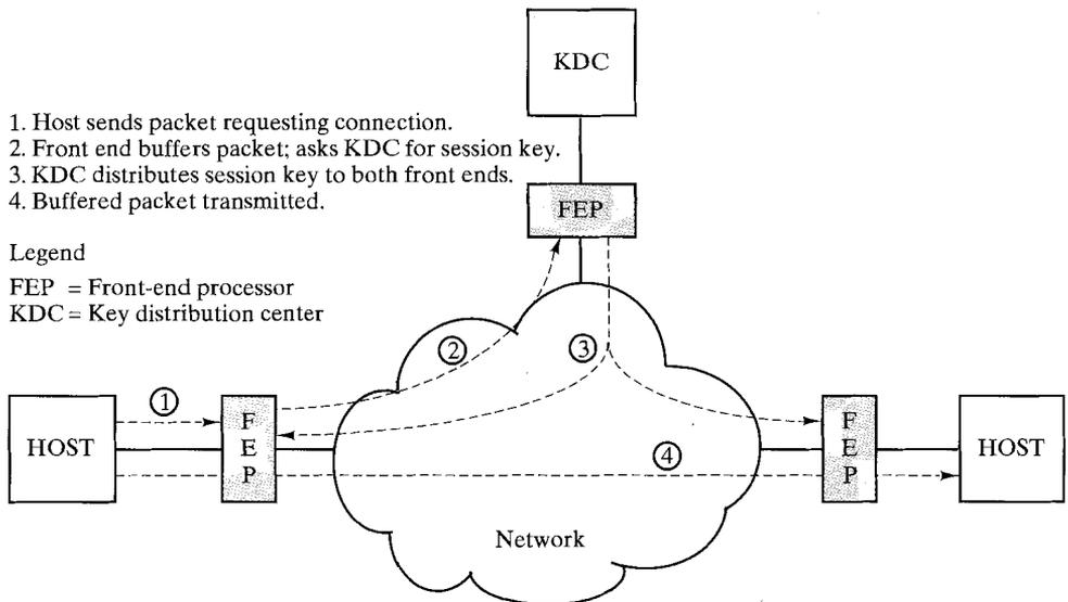
FIGURE 18.8 Automatic key distribution for connection-oriented protocol.
