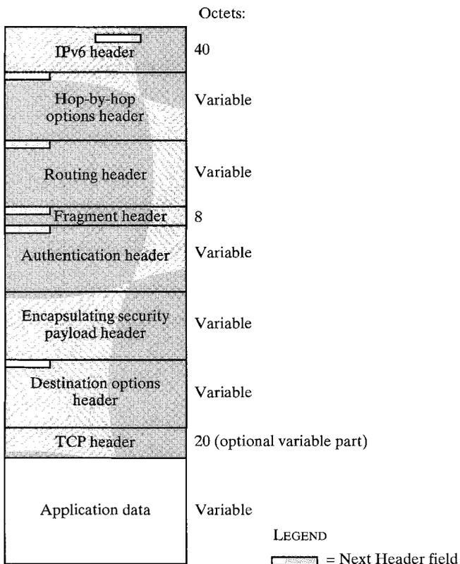
FIGURE 16.15 IPv6 packet with all extension headers.
