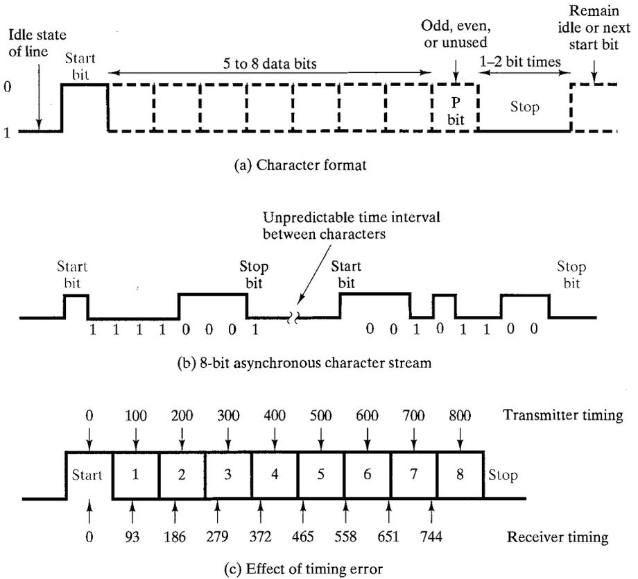
FIGURE 5.1 Asynchronous transmission.
