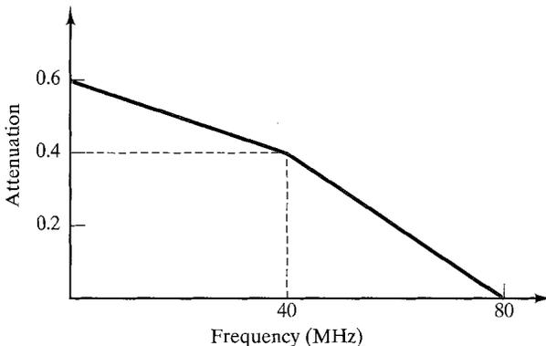
FIGURE 3.6 Filter characteristics of a twisted-pair line.
