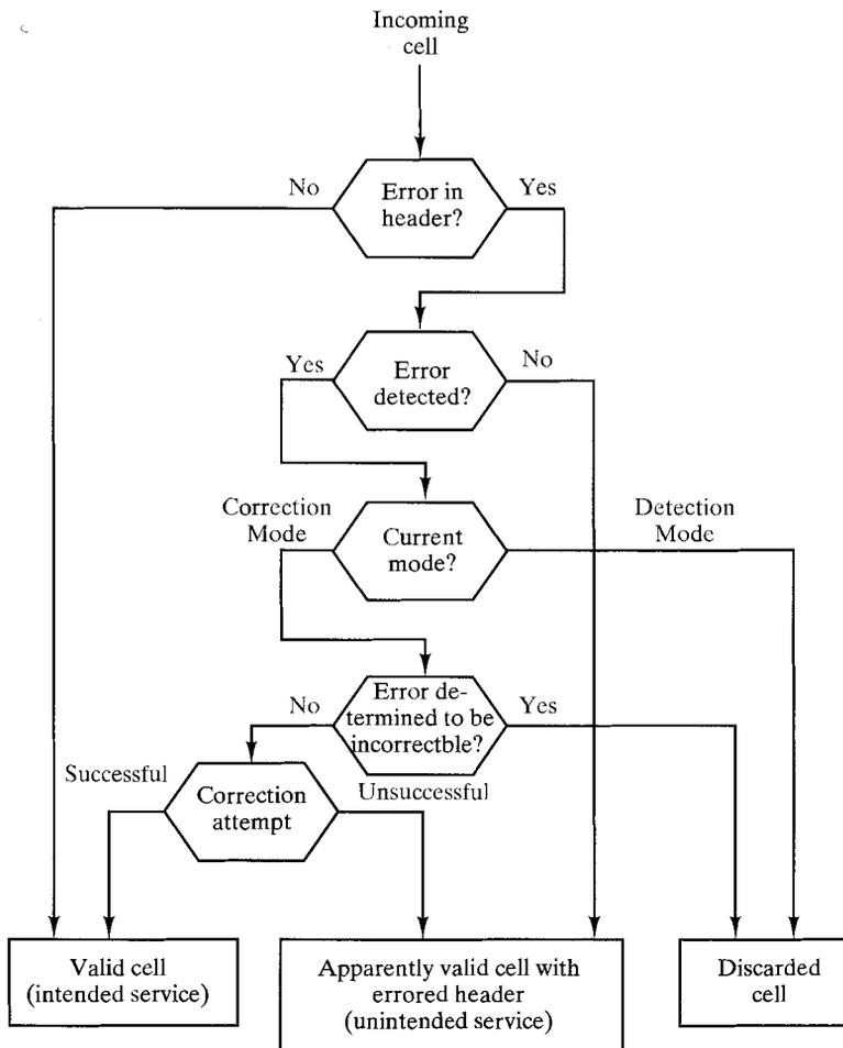
FIGURE 11.6 Effect of error in cell header.
