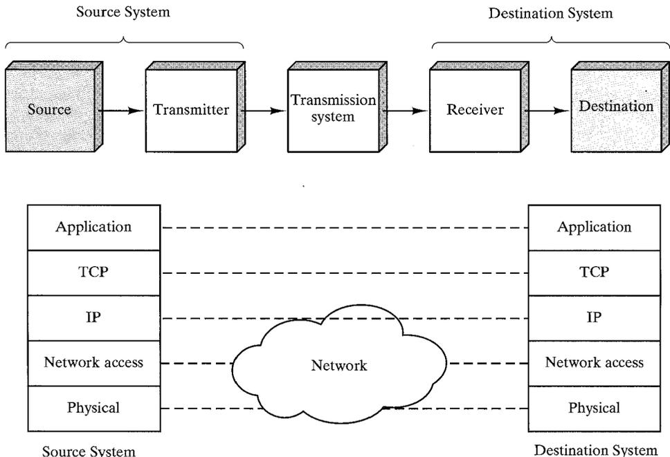
FIGURE 1.9 Protocol architecture model.
