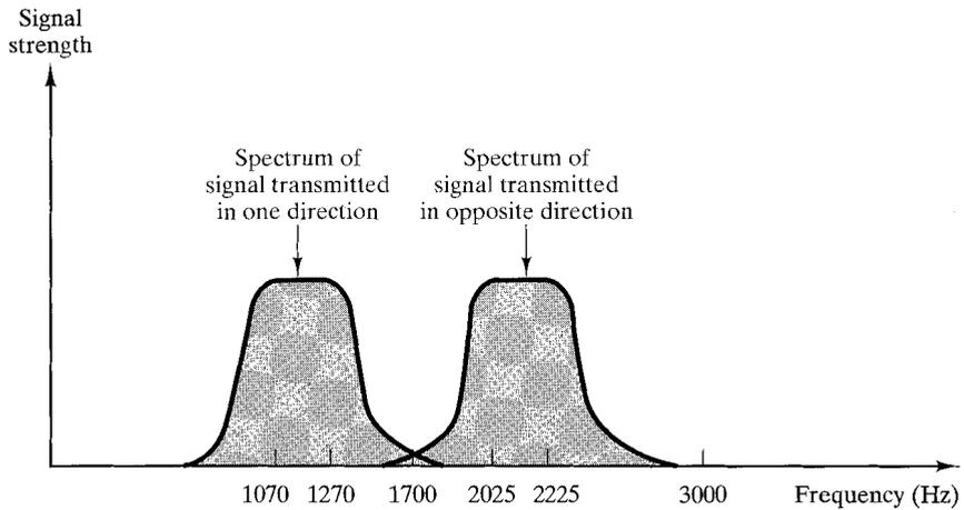
FIGURE 4.8 Full-duplex FSK transmission on a voice-grade line.
