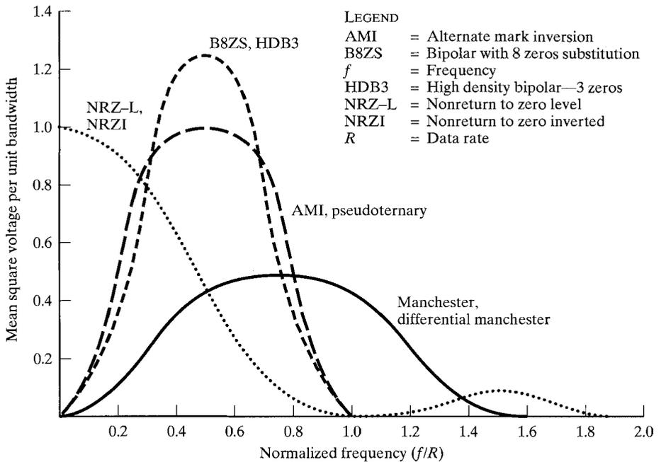
**FIGURE 4.3** Spectral density of various signal encoding schemes.
