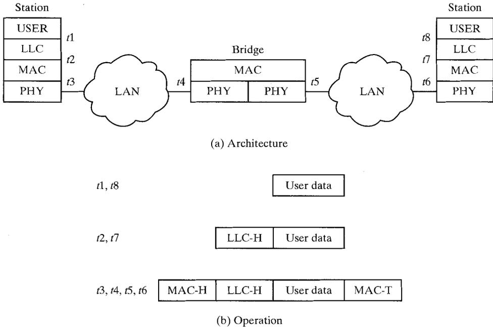
**FIGURE 14.2** Connection of two LANs by a bridge.
