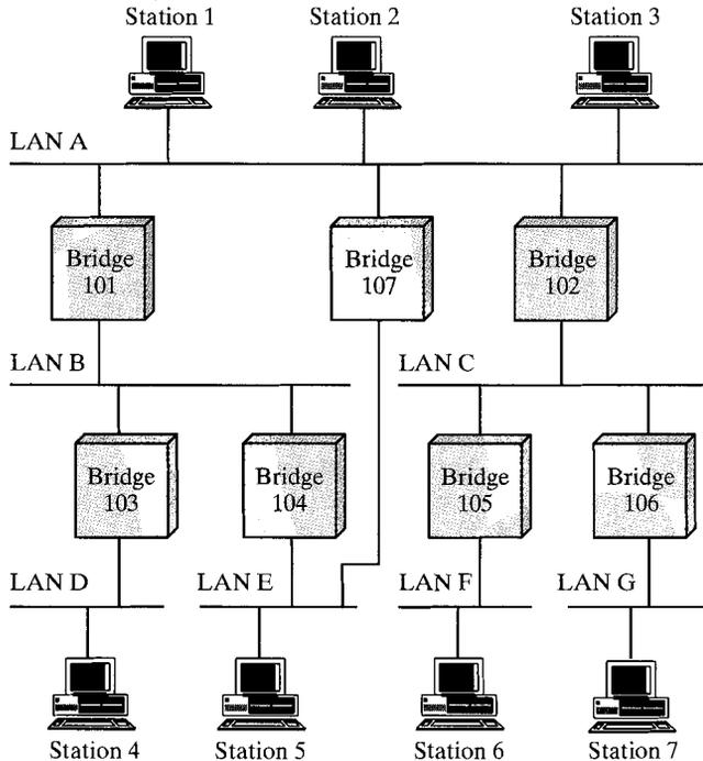
**FIGURE 14.6** Configuration of bridges and LANs, with alternate routes.
