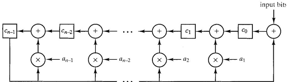
FIGURE 6.7 General CRC architecture to implement divisor  $1 + a_1X + a_2X^2 + \dots + a_{n-1}X^{n-1} + X^n$ .
