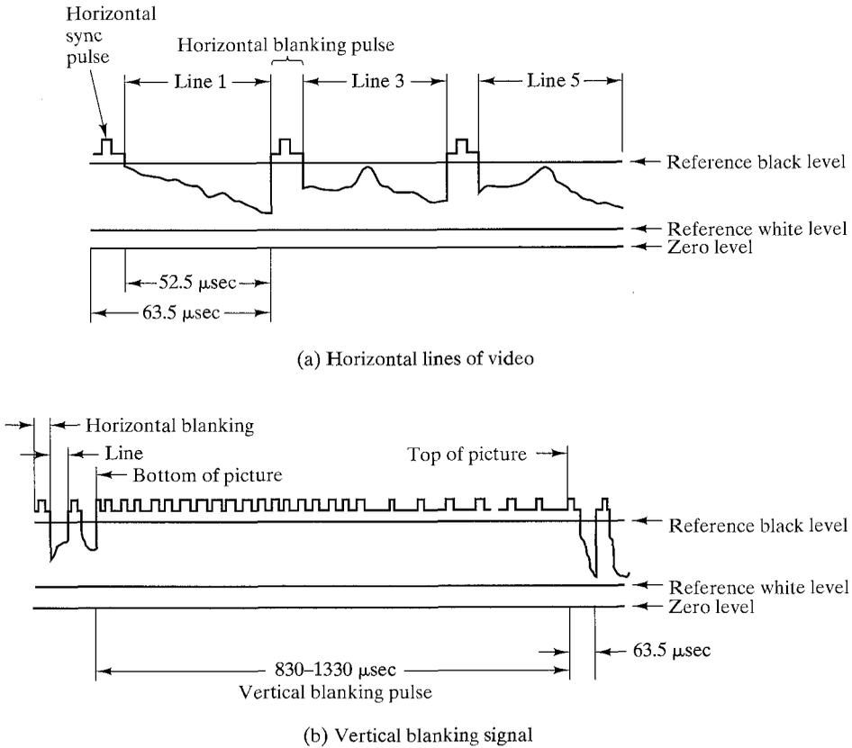
FIGURE 2.12 Video signal (different scales for a and b).
