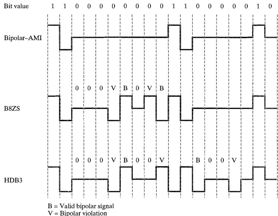
FIGURE 4.6 Encoding rules for B8ZS and HDB3.
