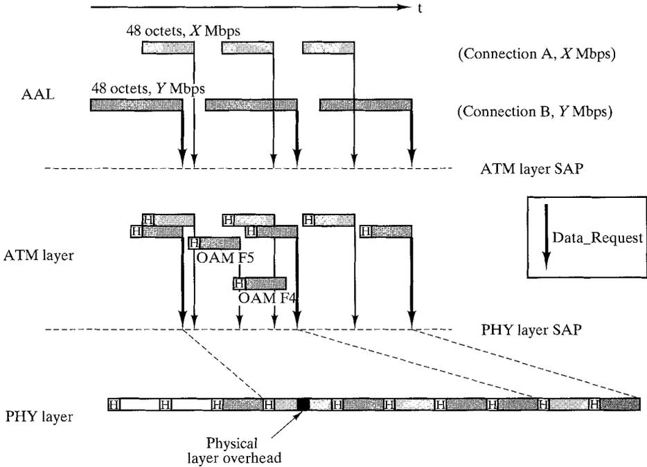
FIGURE 11.17 Origins of cell delay variation (I.371).
