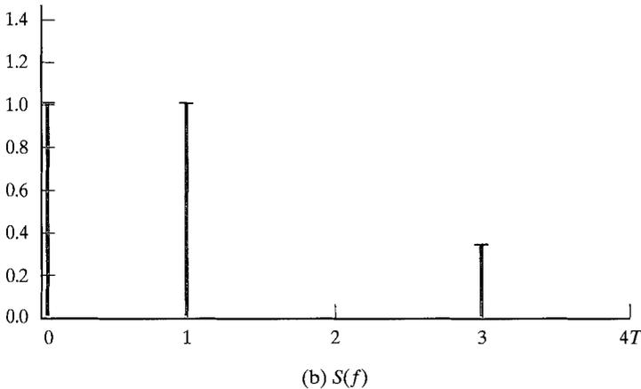
FIGURE 2.7 Signal with dc component.
