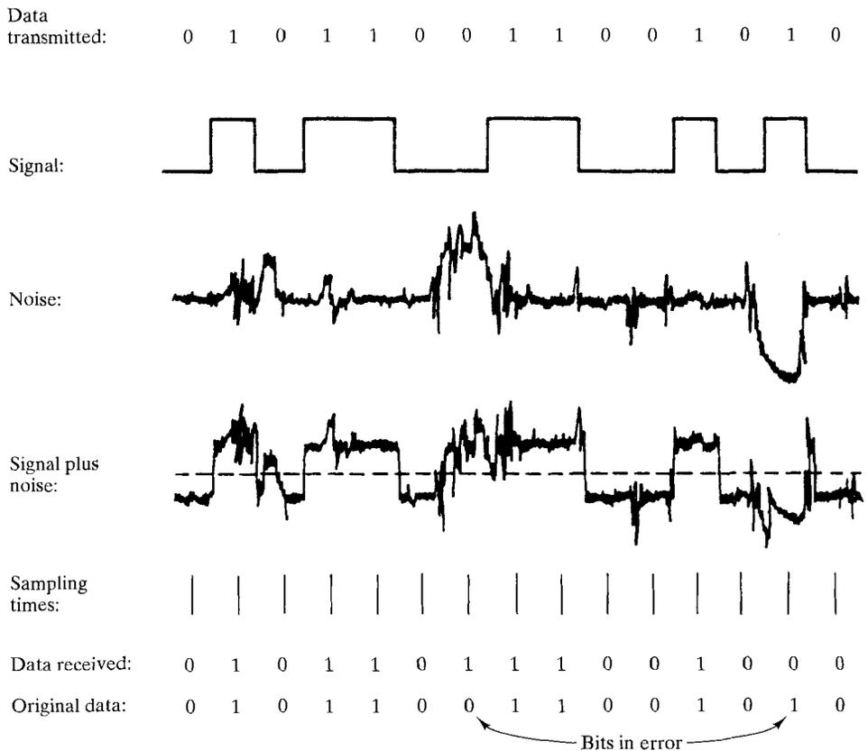
**FIGURE 2.15** Effect of noise on a digital signal.
