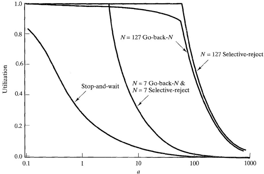
FIGURE 6.17 Line utilization for various error-control techniques ( $P = 10^{-3}$ ).
