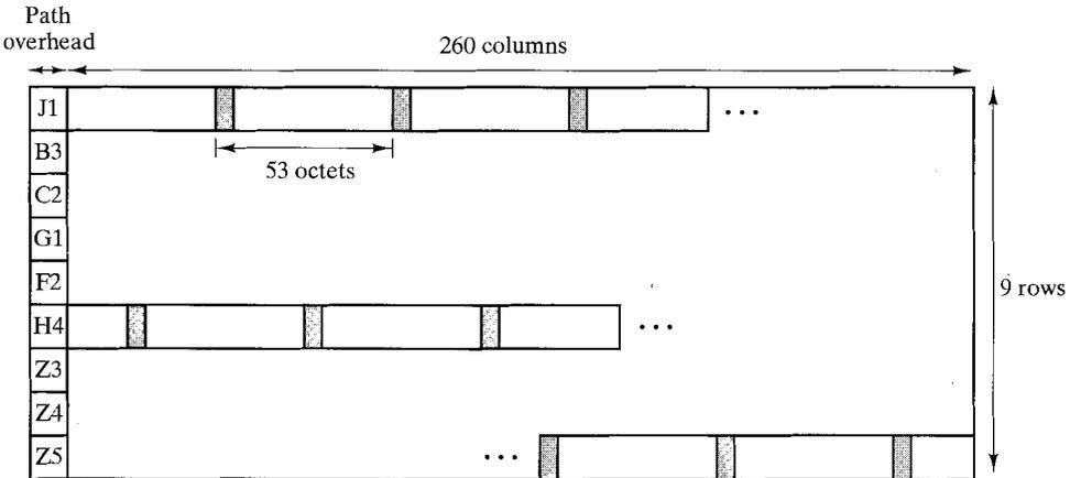
FIGURE 11.11 STM-1 payload for SDH-based ATM cell transmission.
