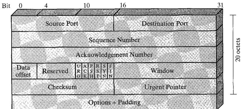
**FIGURE 17.14** TCP header.
