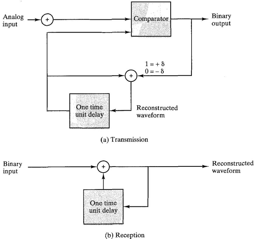
**FIGURE 4.17** Delta modulation.
