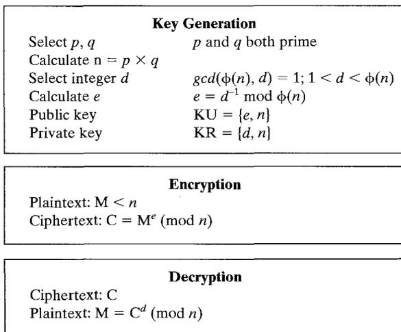
**FIGURE 18.18** The RSA algorithm.
