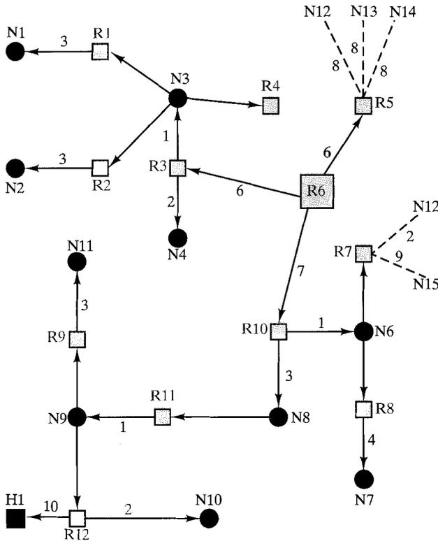
FIGURE 16.14 The SPF tree for router R6.
