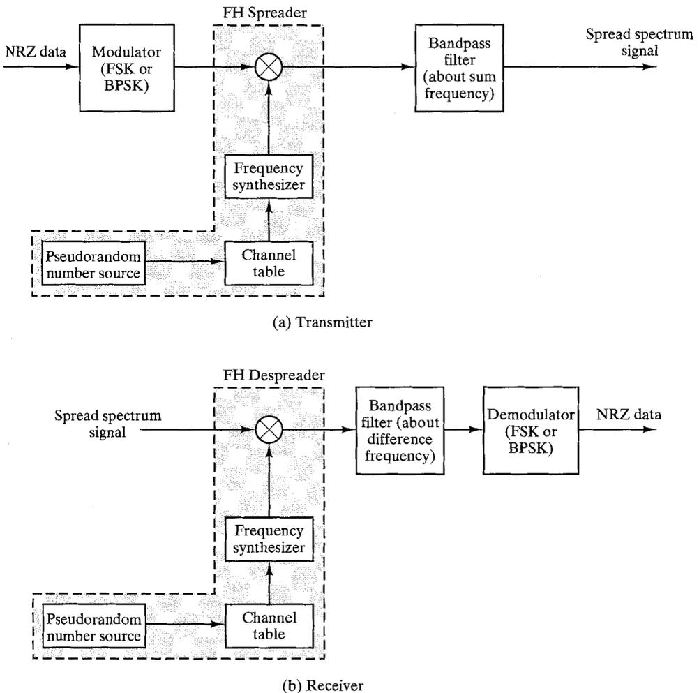
FIGURE 4.22 Frequency-hopping spread spectrum system.
