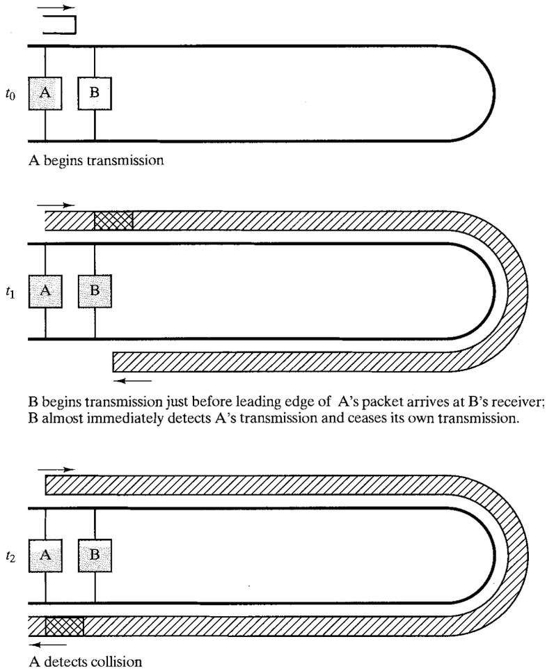
**FIGURE 13.2** Broadband collision detection timing.
