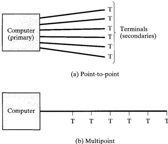
FIGURE 5.3 Traditional computer/terminal configurations.
