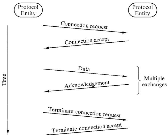
**FIGURE 15.3** The phases of a connection-oriented data transfer.
