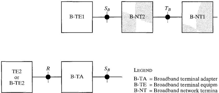
FIGURE A.13 B-ISDN reference configurations.
