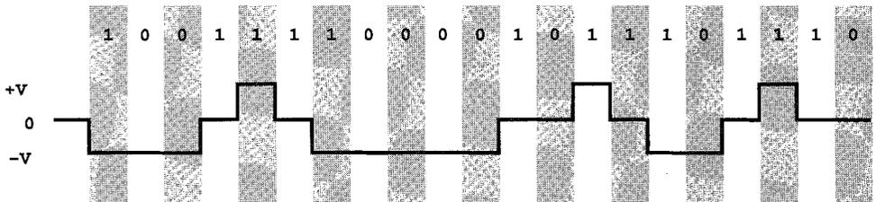
FIGURE 13.23 Example of MLT-3 encoding.
