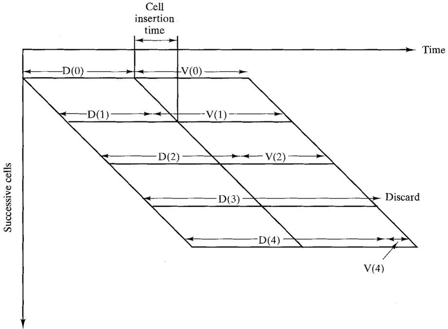
**FIGURE 11.16** Time reassembly of CBR cells.
