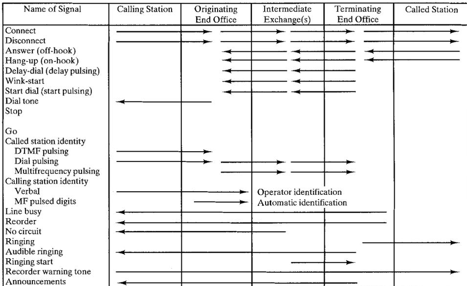
Note: A broken line indicates repetition of a signal at each office, whereas a solid line indicates direct transmittal through intermediate offices.
