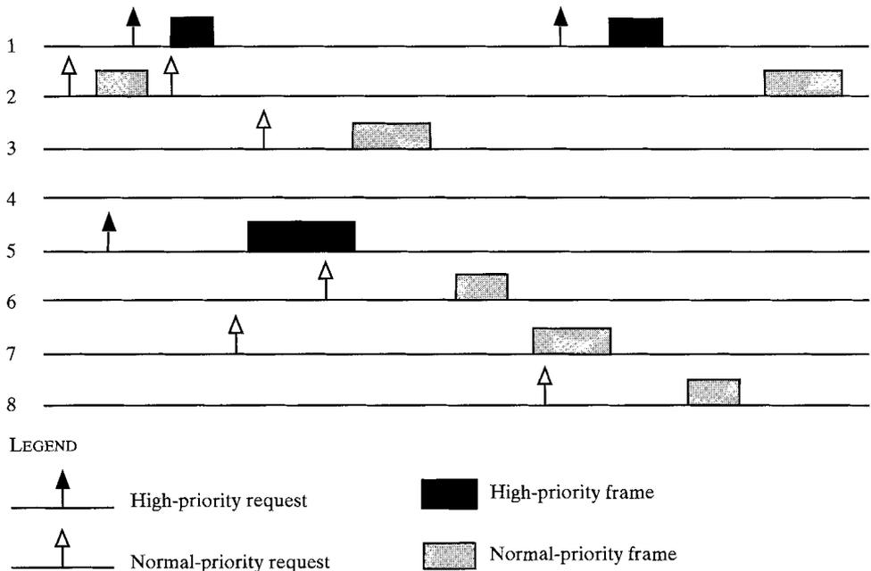
**FIGURE 13.11** Example frame sequence in a single-repeater network.
