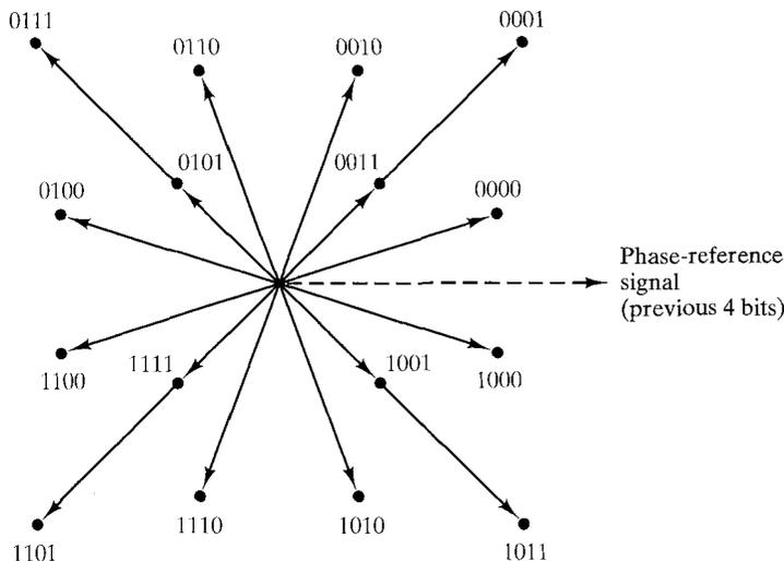
FIGURE 4.9 Phase angles for 9600 bit-per-second transmission.
