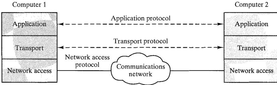
FIGURE 1.6 Protocols in a simplified architecture.
