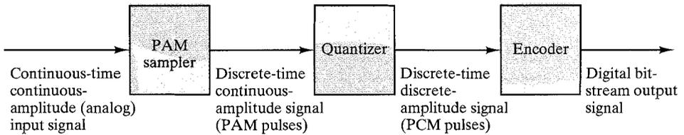
**FIGURE 4.13** Analog-to-digital conversion.
