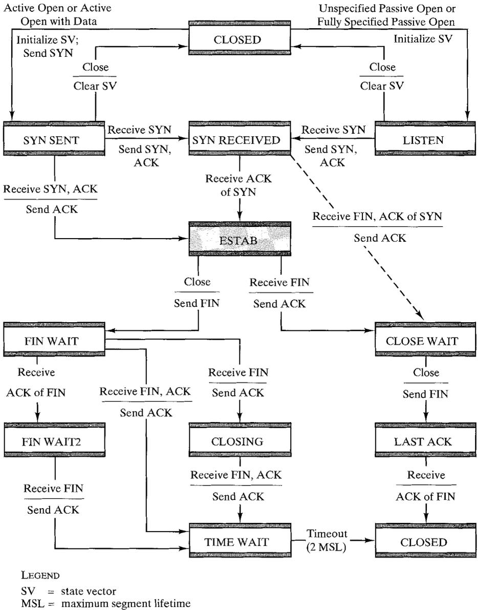
FIGURE 17.12 TCP entity state diagram.
