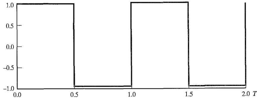
(c)  $\sum 1/k \sin(2\pi k f_1 t)$ **FIGURE 2.8** Frequency components of a square wave ( $T = 1/f_1$ ).
