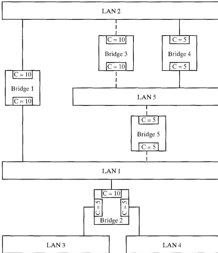
**FIGURE 14.10** Example configuration for spanning tree algorithm.
