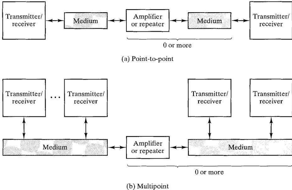
**FIGURE 2.1** Guided transmission configurations.
