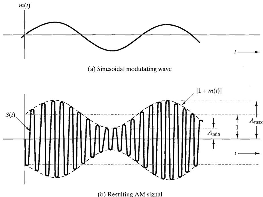
FIGURE 4.18 Amplitude modulation.
