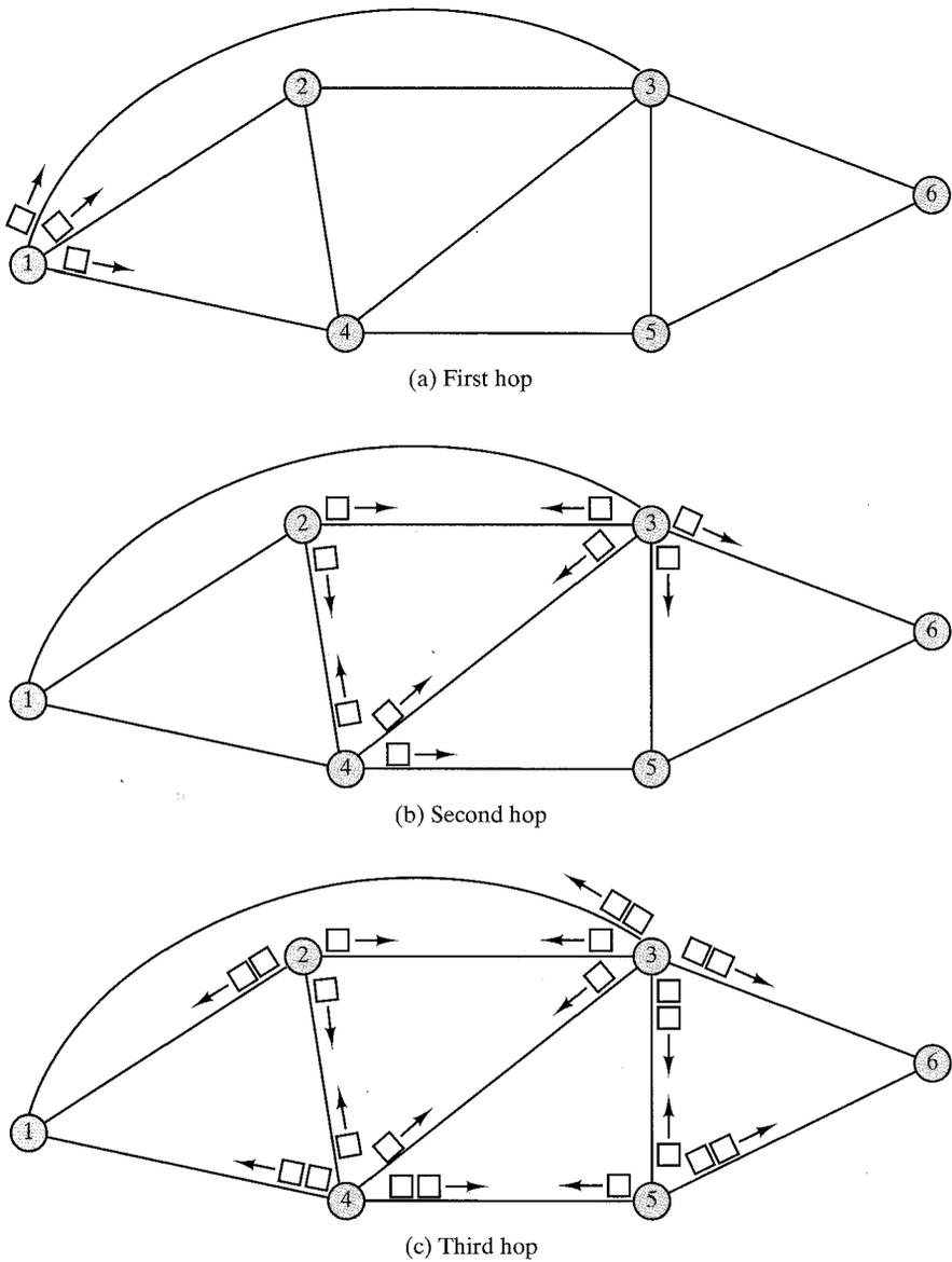
**FIGURE 9.7** Flooding example (hop count = 3).
