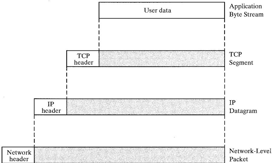
**FIGURE 15.11** Protocol data units in the TCP/IP architecture.
