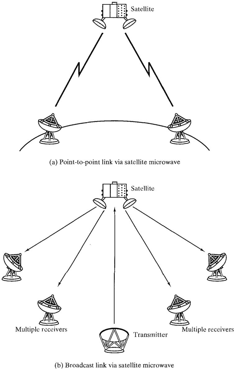
**FIGURE 3.4** Satellite communications configurations.
