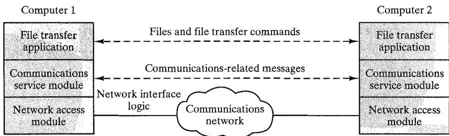
**FIGURE 1.4** A simplified architecture for file transfer.
