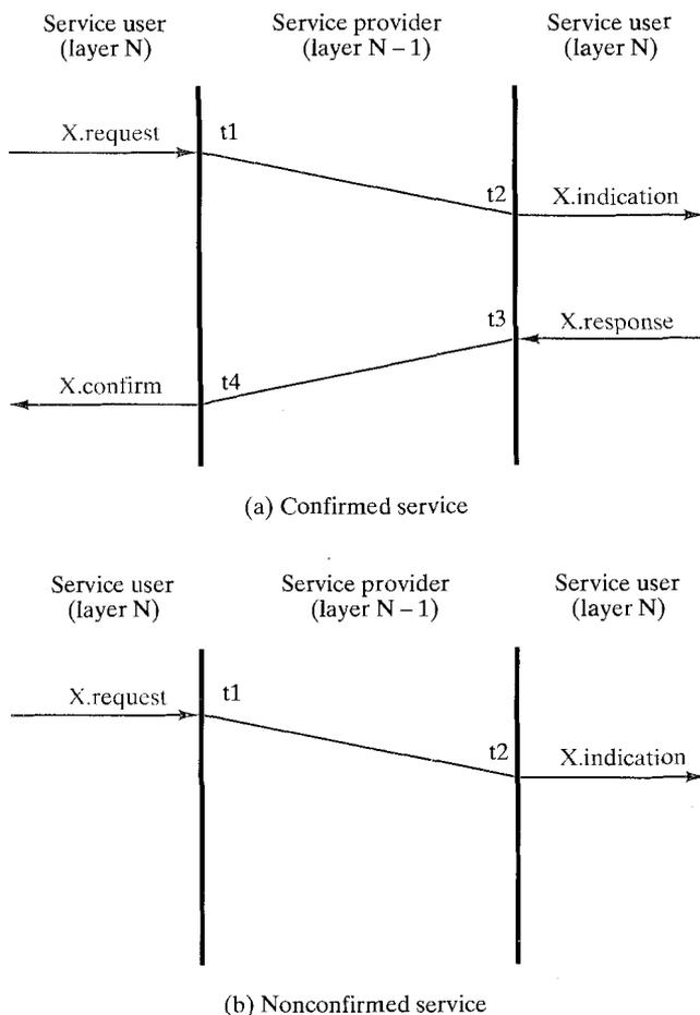
**FIGURE 15.9** Time sequence diagrams for service primitives.
