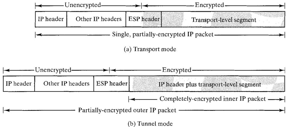
**FIGURE 18.22** Secure IPv4 datagram or IPv6 packet.
