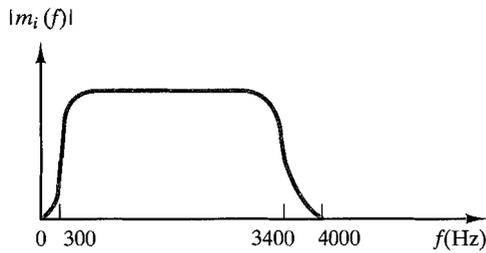
(a) Spectrum of  $m_i(t)$ , positive  $f$
