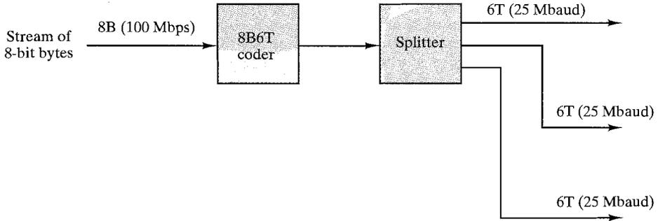
**FIGURE 13.24** 8B6T transmission scheme.
