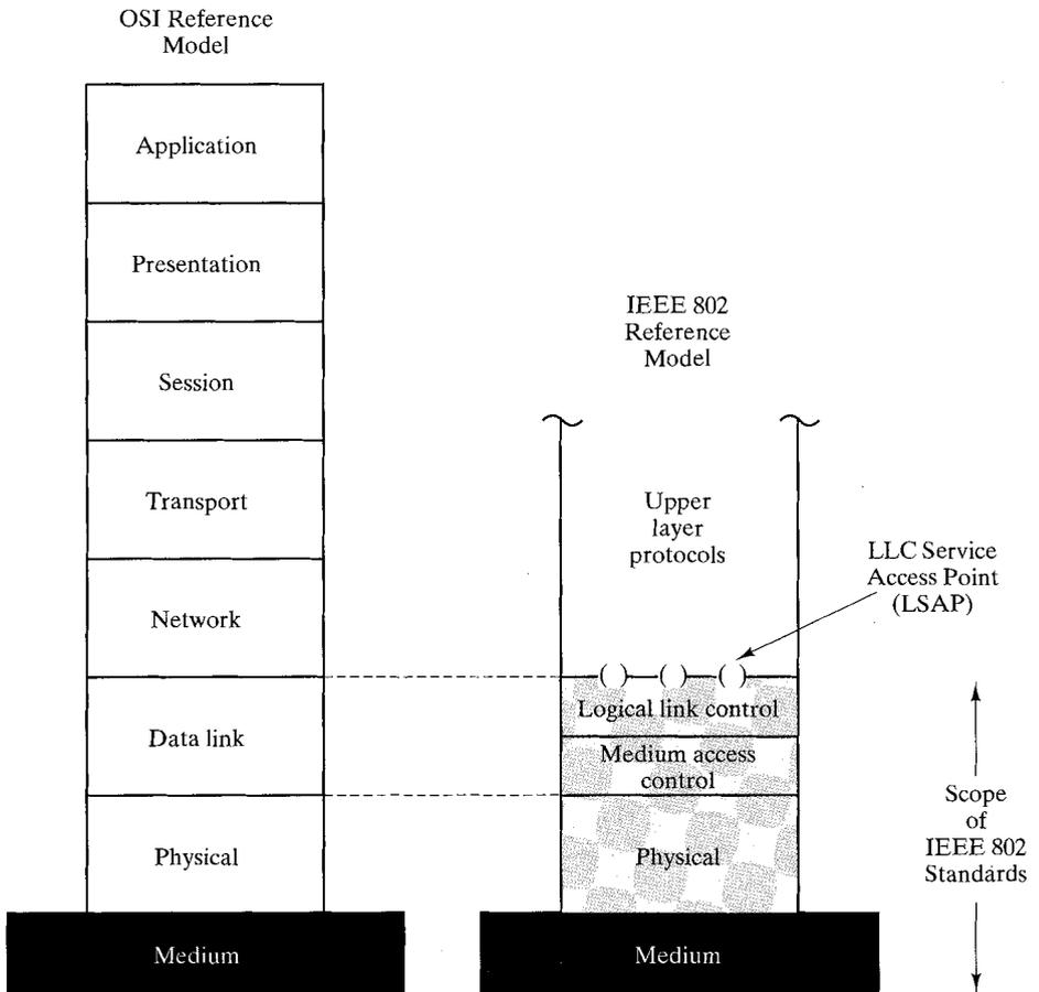
**FIGURE 12.1** IEEE 802 protocol layers compared to OSI model.
