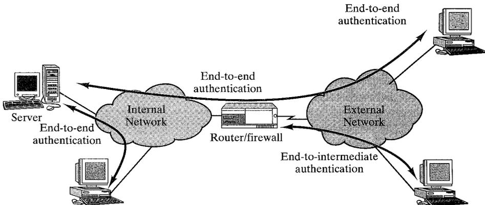
FIGURE 18.21 End-to-end versus end-to-intermediate authentication [DOTY95].
