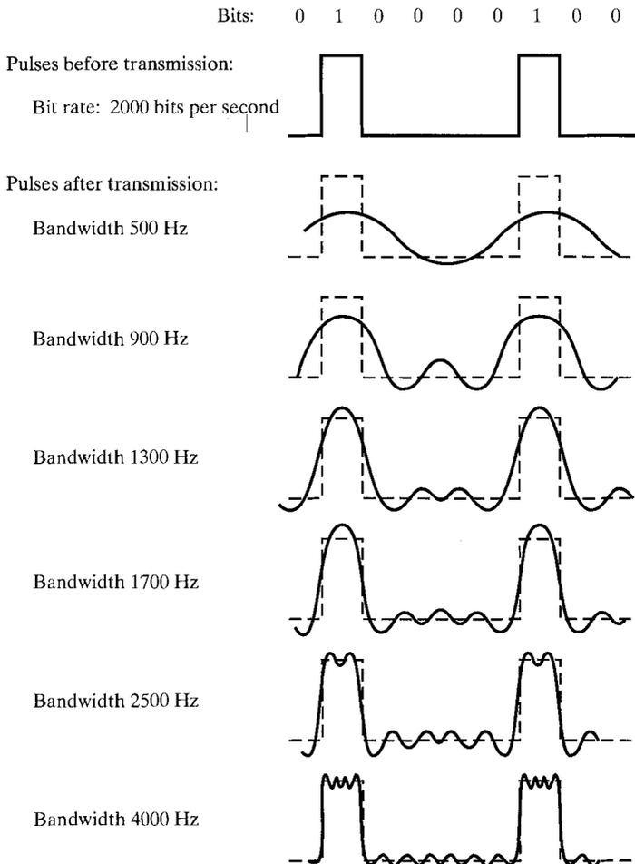
**FIGURE 2.9** Effect of bandwidth on a digital signal.
