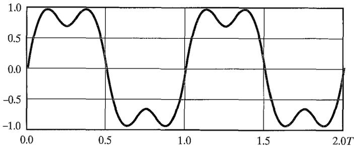
(c)  $\sin(2\pi f_1 t) + \frac{1}{3} \sin(2\pi(3f_1)t)$ **FIGURE 2.5** Addition of frequency components ( $T = 1/f_1$ ).
