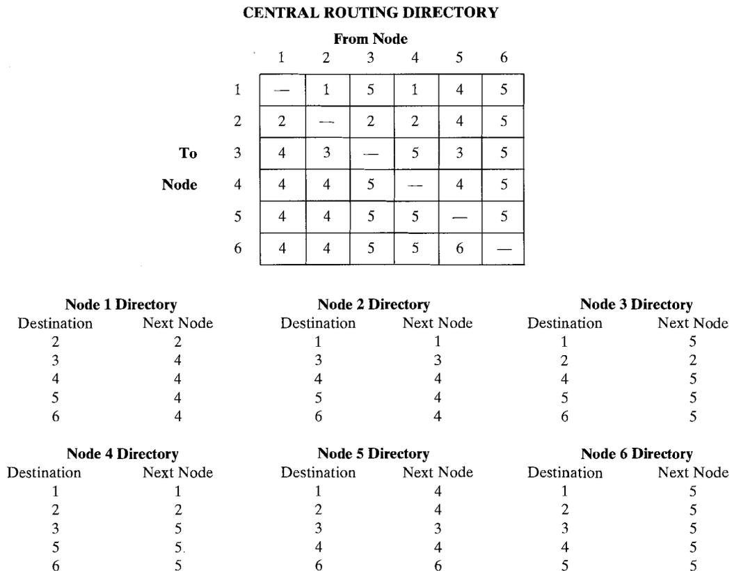
**FIGURE 9.6** Fixed routing (using Figure 9.5).
