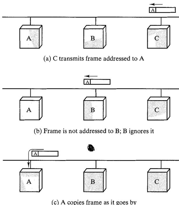
**FIGURE 12.5** Frame transmission on a bus LAN.
