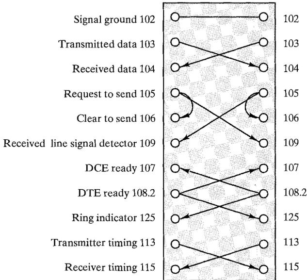
FIGURE 5.8 Example of a null modem.
