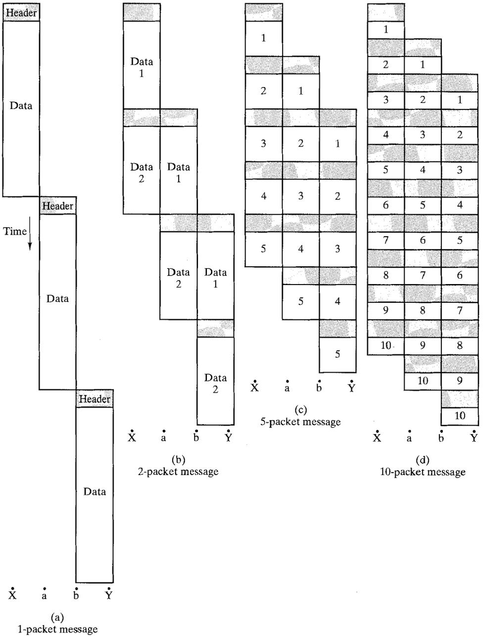
**FIGURE 9.2** Effect of packet size on transmission time.
