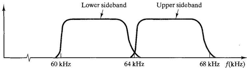
(b) Spectrum of  $S_{sc1}(t)$  for  $f_{sc1} = 64$  kHz
