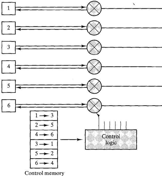
**FIGURE 8.8** Control of a TDM bus switch.
