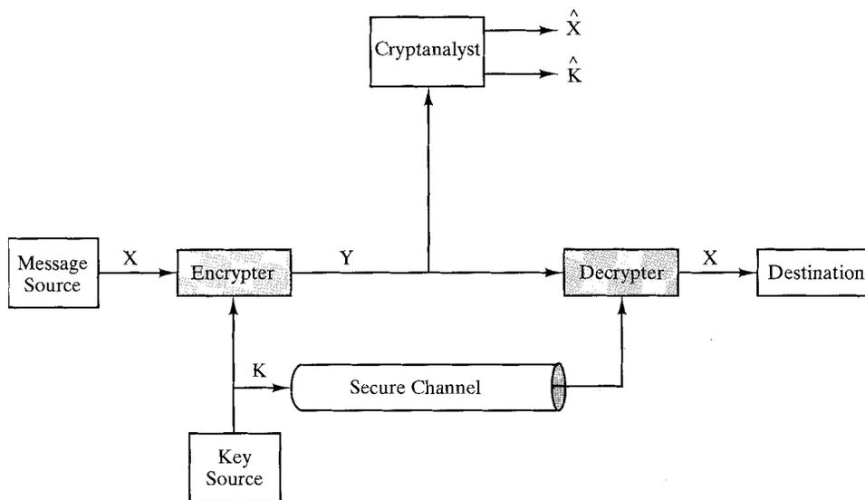
FIGURE 18.3 Model of conventional cryptosystem.
