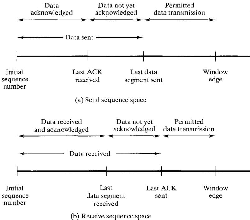
**FIGURE 17.6** Sending and receiving flow control perspectives.
