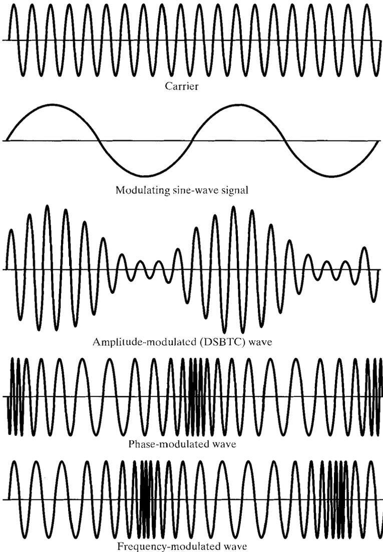
**FIGURE 4.20** Amplitude, phase, and frequency modulation of a sine-wave carrier by a sine-wave signal.
