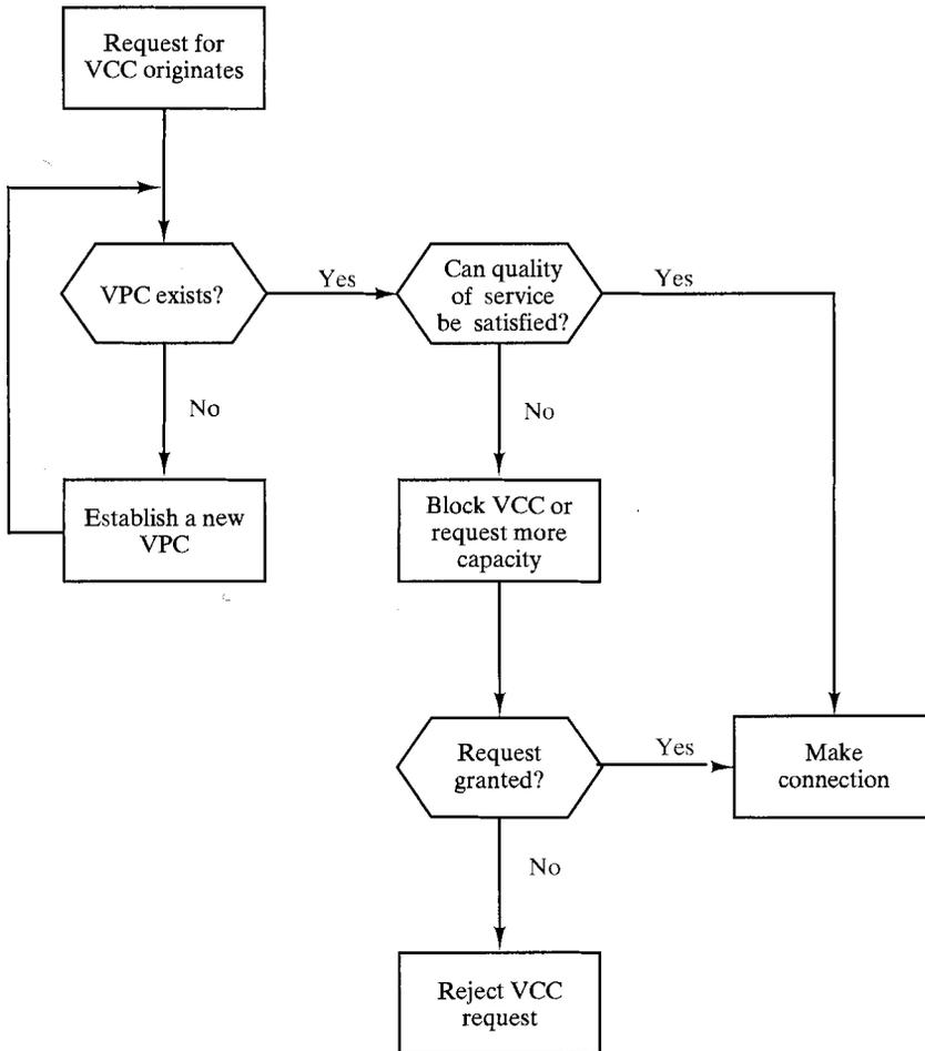
FIGURE 11.3 Call establishment using virtual paths.
