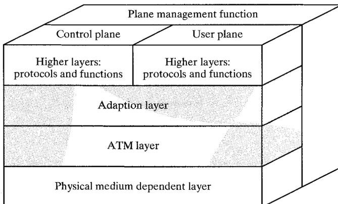
**FIGURE A.14** B-ISDN protocol model for ATM.
