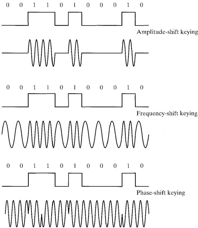
**FIGURE 4.7** Modulation of analog signals for digital data.
