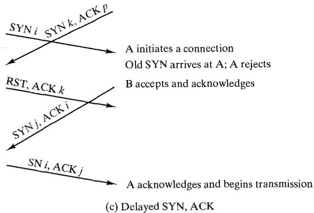
**FIGURE 17.13** Examples of three-way handshake.
