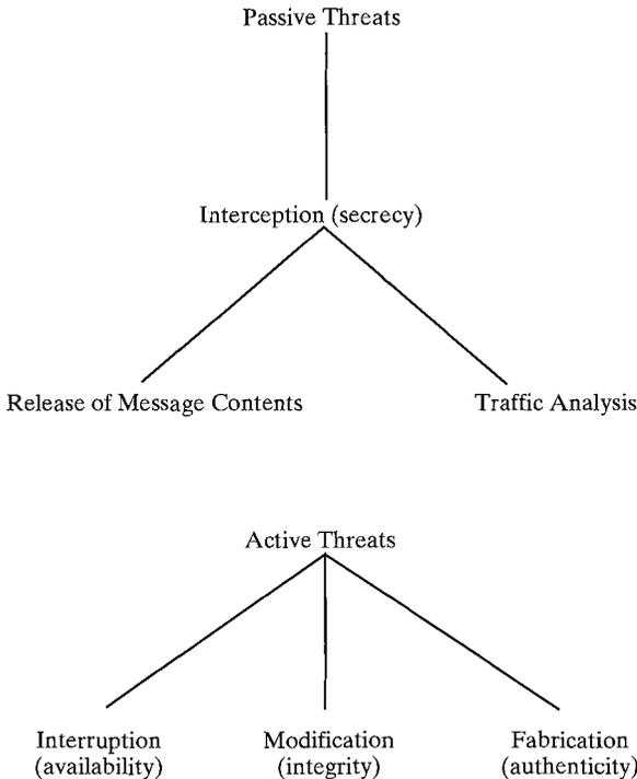
**FIGURE 18.2** Active and passive network security threats.
