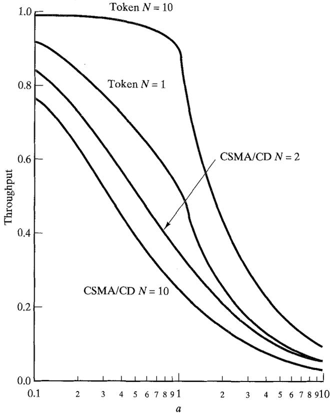
**FIGURE 13.28** Throughput as a function of  $a$  for token passing and CSMA/CD.
