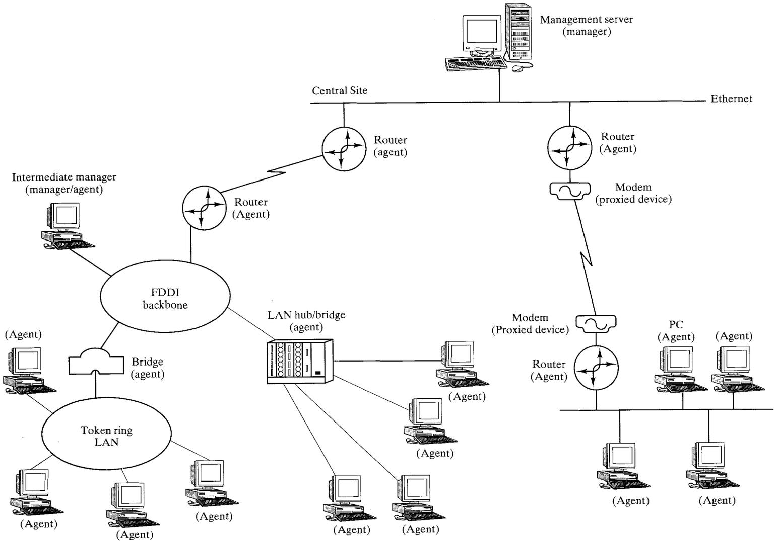
**FIGURE 19.5** Example distributed network management configuration.
