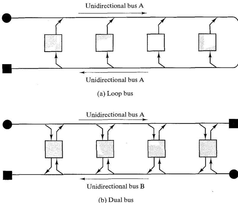
FIGURE 12.11 Optical fiber bus configurations.
