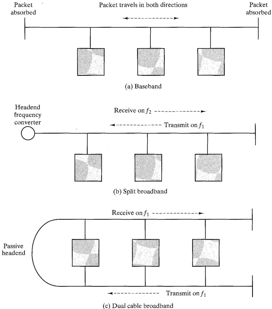
**FIGURE 12.8** Baseband and broadband transmission techniques.
