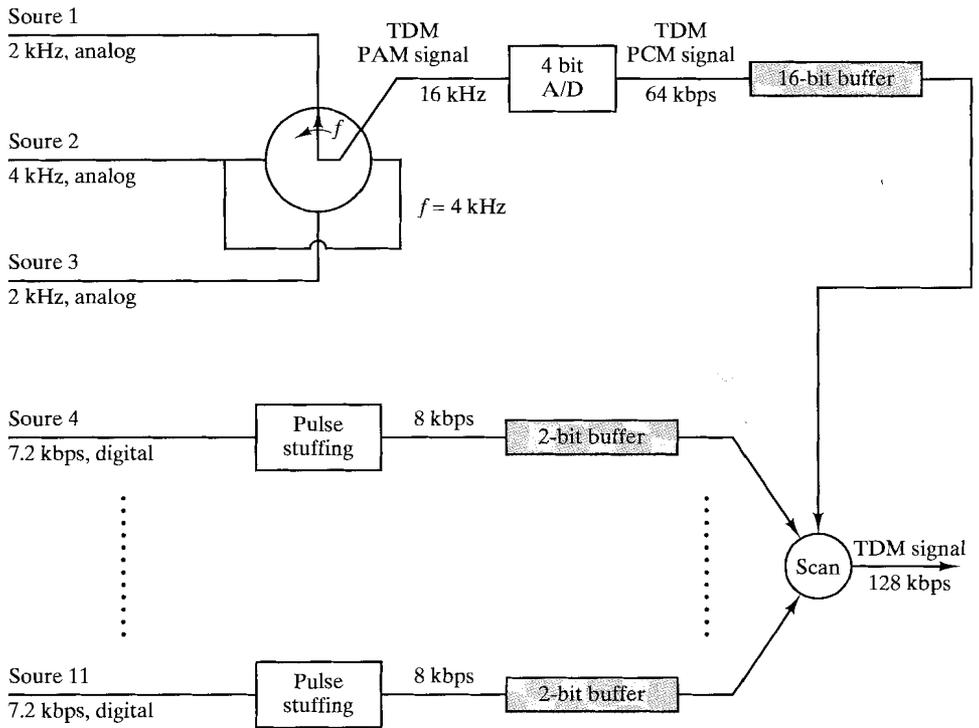
FIGURE 7.8 TDM of analog and digital sources.
