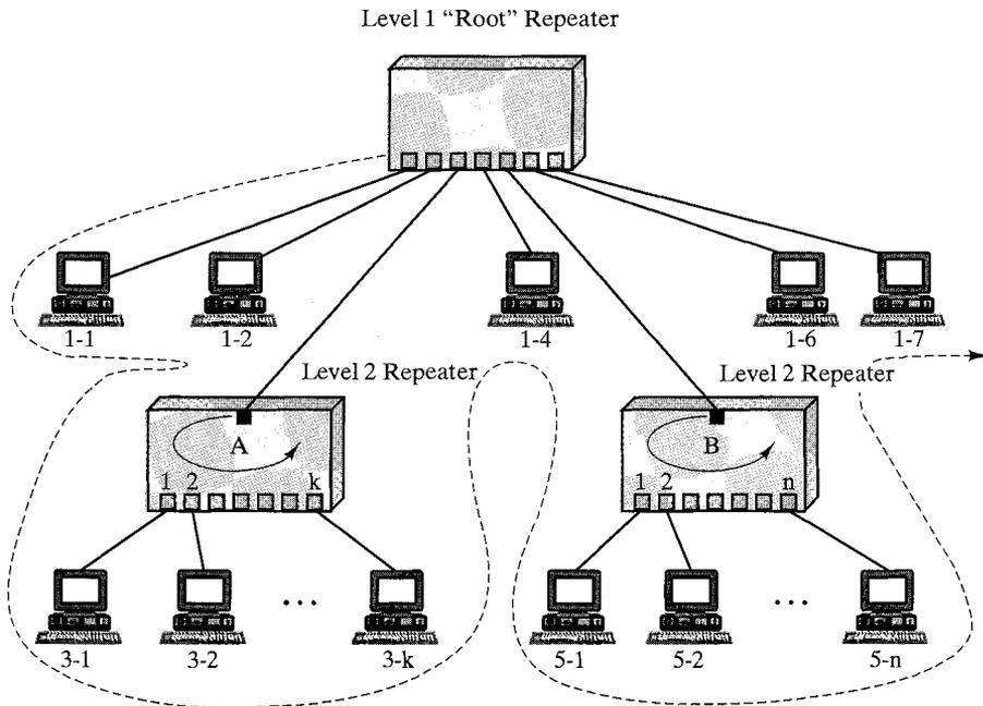
FIGURE 13.12 Port ordering in a two-level IEEE 802.12 network.
