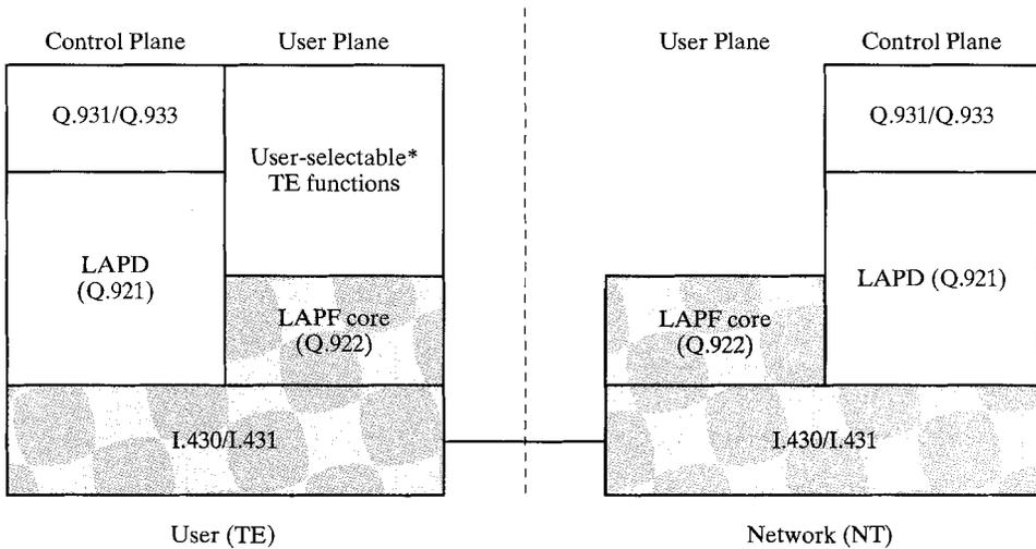
\* Additional functions to support flow and error control may be provided. LAPF control is one protocol that may be used.
