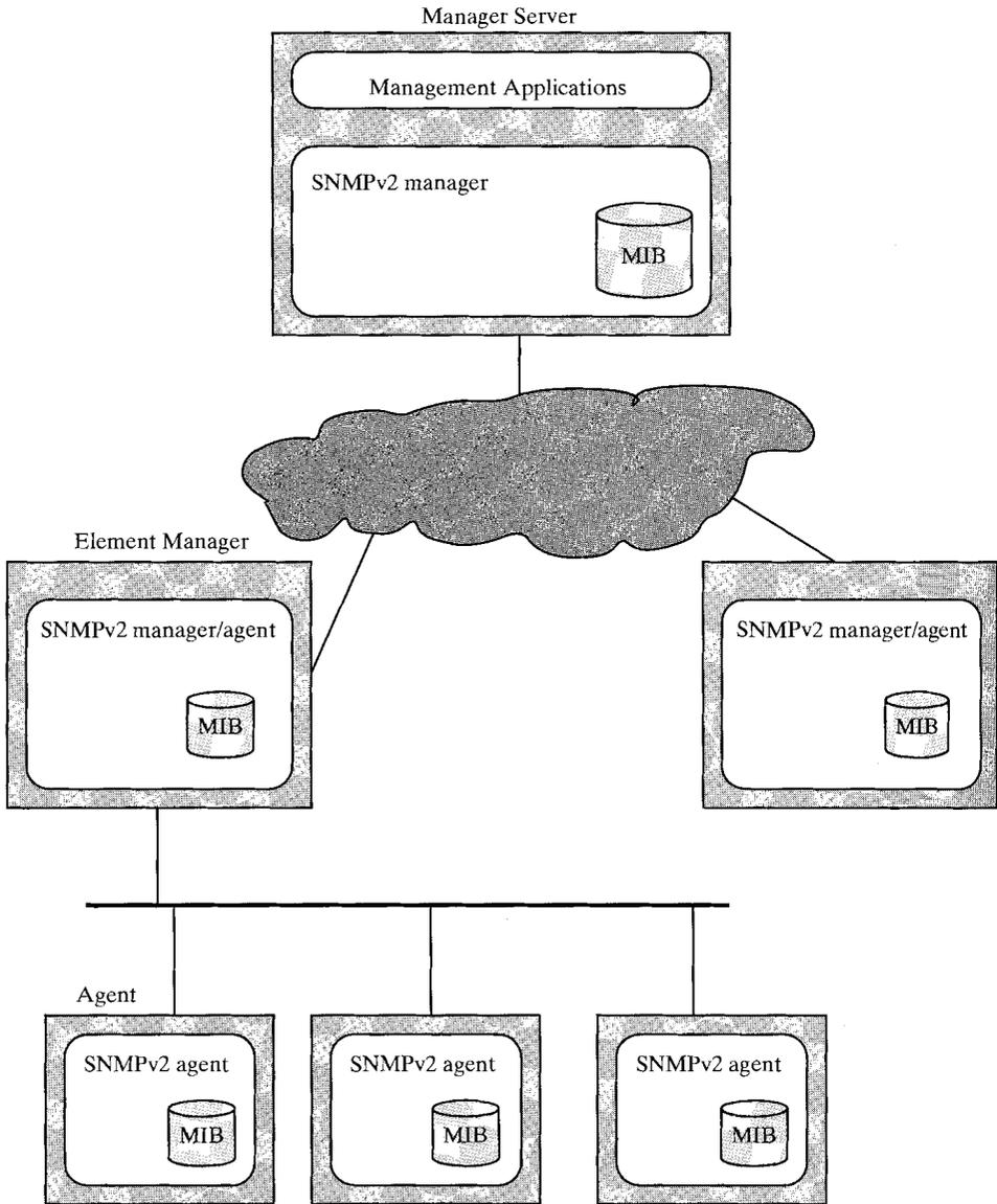
**FIGURE 19.6** SNMPv2-managed configuration.
