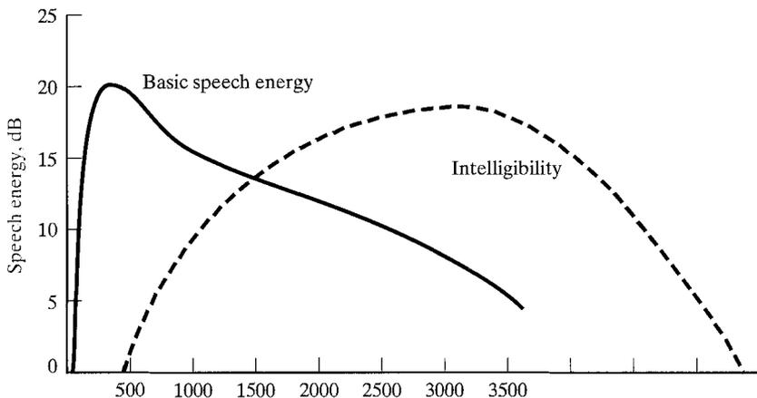
**FIGURE 2.10** Acoustic spectrum for speech. *SOURCE: [FREE89]*
