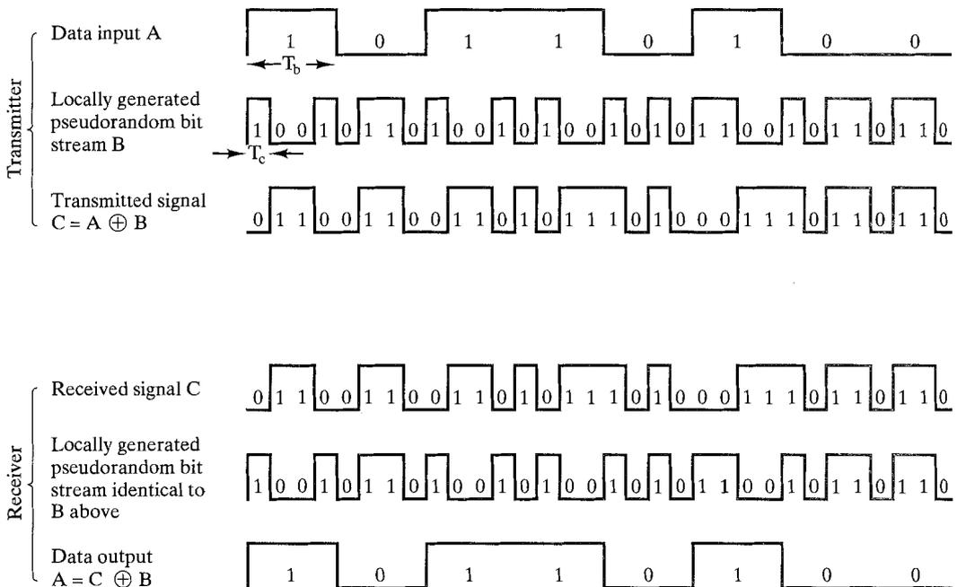
FIGURE 4.23 Example of direct sequence spread spectrum.
