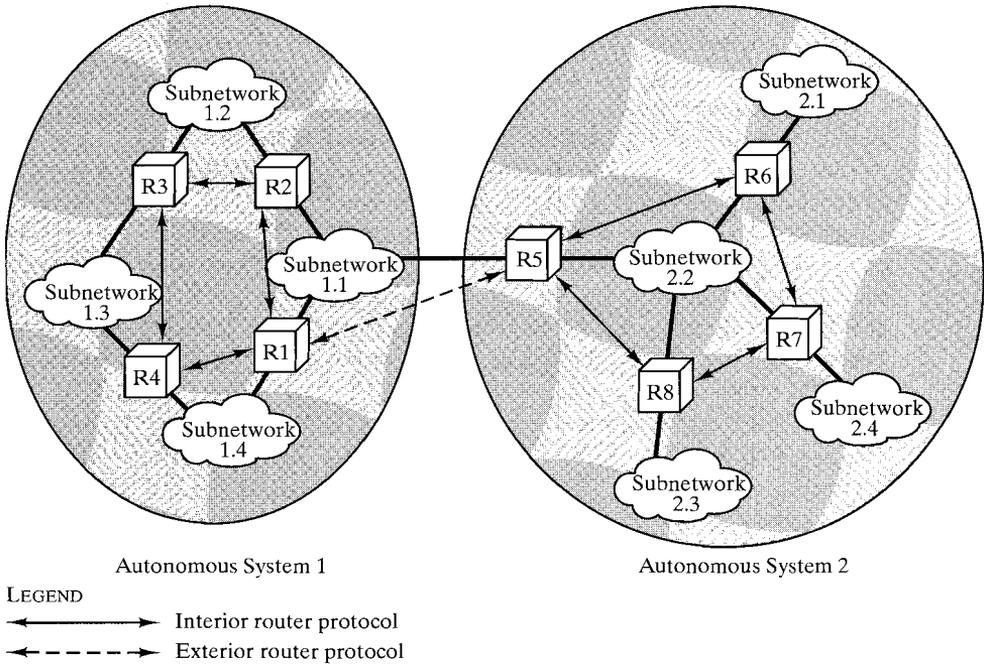
**FIGURE 16.10** Application of exterior and interior routing protocols.
