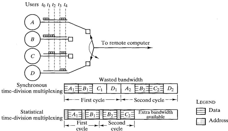
FIGURE 7.14 Synchronous TDM contrasted with statistical TDM.
