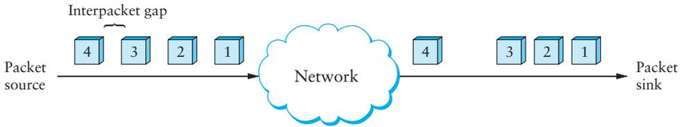
**Figure 1.24 Network-induced jitter.**
