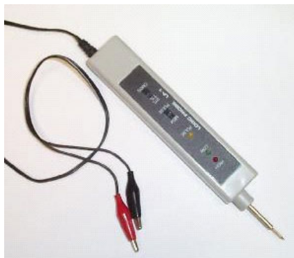
Figure 10. An example of a digital logic probe
