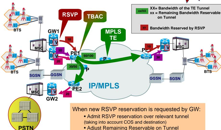
RSVP signalling encapsulated in TE Tunnel
