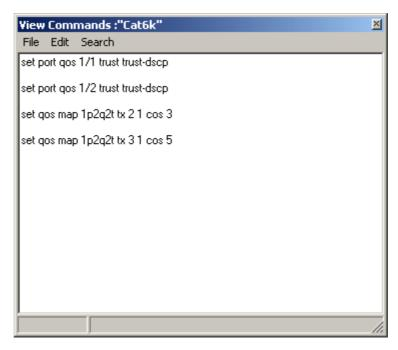
Figure 2-25 Previewing the CLI for Catalyst 6000 Access-to-Distribution Uplinks
