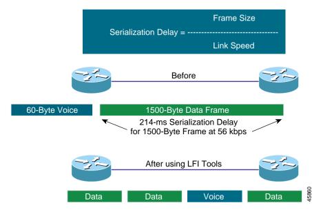
Figure 5-2 Using LFI Tools to Reduce Frame Delay
