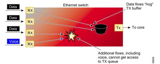
Figure 3-2 Loss of Voice Quality When Transmit Buffer Is Full
