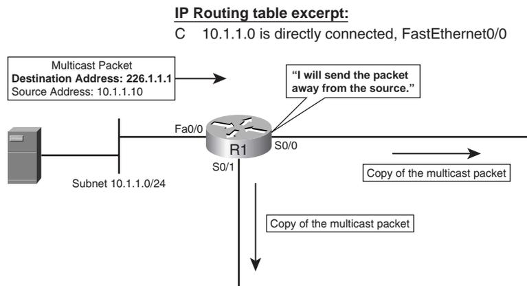
Figure 20-2 shows the dense-mode logic on R1, with R1 *flooding* copies of the packet out all interfaces except the one on which the packet was received. Although Figure 20-2 shows only one router, other routers can receive these multicasts and repeat the same process. All subnets will receive a copy of the original multicast packet.
