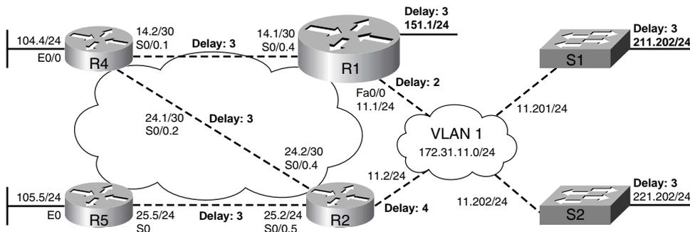
**NOTE** The routers have disabled the use of bandwidth in the EIGRP metric calculation, so all metrics in Example 9-4 are multiples of 256.
