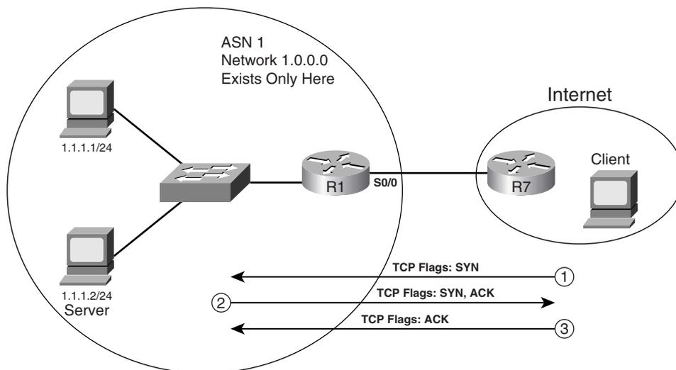
Cisco IOS ACLs cannot directly match the TCP SYN flag. However, an ACE can use the **established** keyword, which matches TCP segments that have the ACK flag set. The **established** keyword essentially matches all TCP segments except the very first TCP segment in a new connection. Example 21-11 shows the configuration that would be used on R1 to deny new connection requests from the Internet into the network on the left.
