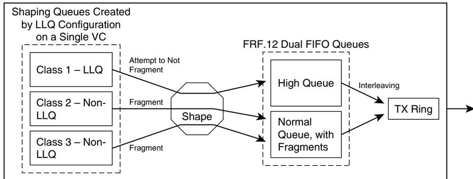
**NOTE** All packets can be fragmented, but Cisco rightfully suggests choosing a fragment size so that the packets typically placed into the LLQ PQ will not be fragmented. Only packets from the shaping LLQ are placed into the Dual FIFO interface high queue, and only those packets are interleaved.
