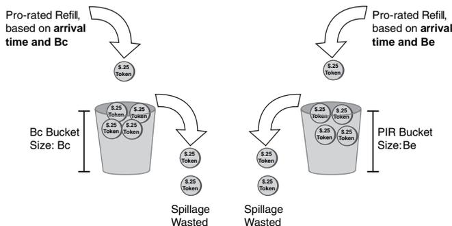
The refilling of the two buckets based on two different rates is very important. For example, imagine you set a CIR of 128 kbps (16 kilobytes/second), and a PIR of 256 kbps (32 kbps). If 0.1 second passed before the next packet arrived, then the CIR bucket would be replenished with 1600 tokens (1/10 of 1 second’s worth of tokens, in bytes), while the PIR bucket would be replenished with 3200 tokens. So, there are more tokens to use in the PIR bucket, as compared to the CIR bucket.
