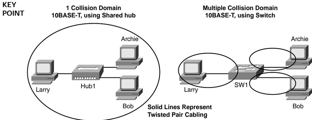
Switches have the same cabling and signal regeneration benefits as hubs, but switches do a lot more—including sometimes reducing or even eliminating collisions by buffering frames. When switches receive multiple frames on different switch ports, they store the frames in memory buffers to prevent collisions.
