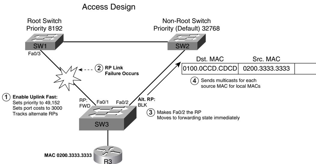
Upon enabling UplinkFast globally in a switch, the switch takes three actions:
