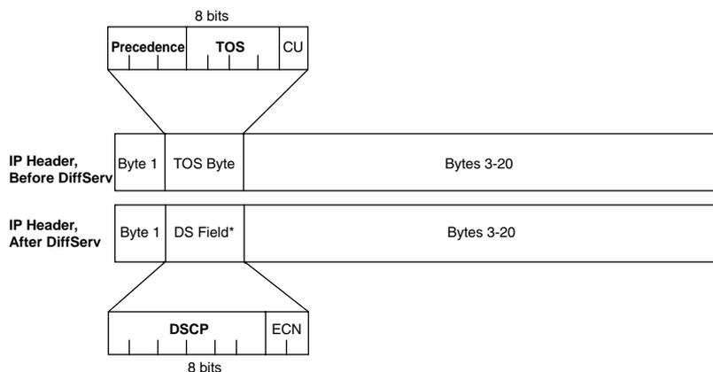
C&M tools often mark DSCP or IPP because the IP packet remains intact as it is forwarded throughout an IP network. The other possible marking fields reside inside Layer 2 headers, which means the headers are discarded when forwarded by a Layer 3 process. Thus, the latter cannot be used to carry QoS markings beyond the current hop.
