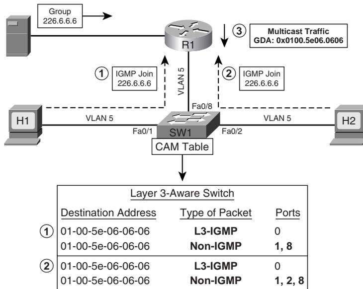
The following three steps, referenced in Figure 19-20, describe the sequence of events when H1 and H2 send IGMP Join messages:
