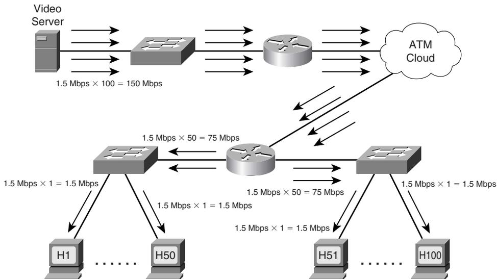
Figure 19-3 *Broadcast Wastes Bandwidth and Increases Processing Load on CPU*
