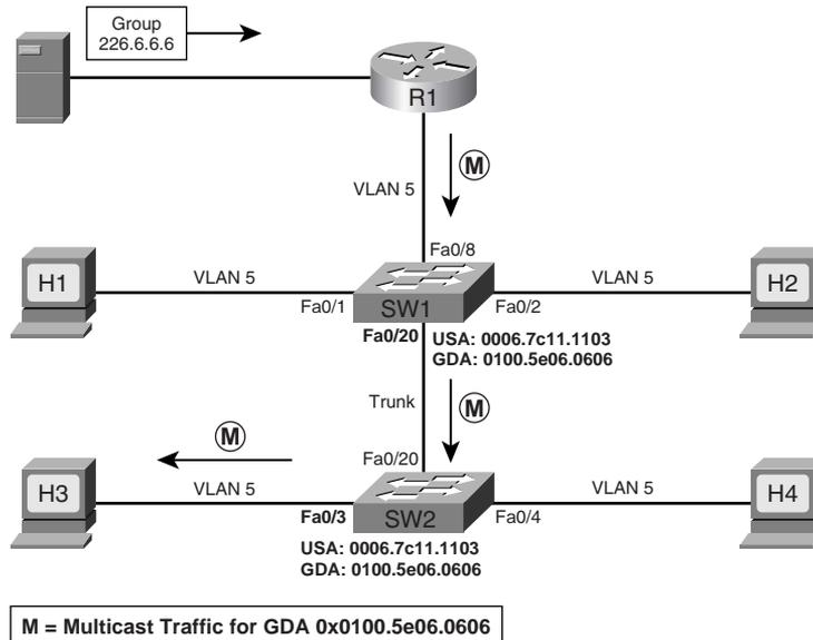
When R1 forwards multicast traffic with GDA 0x0100.5e06.0606 to SW1, as shown in Figure 19-18, SW1 searches its CAM table and notices that this traffic should be forwarded only on port fa0/20. Therefore, only SW2 receives the group traffic. Similarly, SW2 searches its CAM table and forwards the group traffic only on its port fa0/3, and only H3 receives the group traffic.
