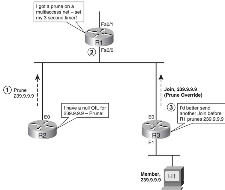
This process is called *Prune Override* because R3 overrides the Prune sent by R2. The Prune Override is actually a Join message, sent by R3 in this case. The message itself is no different from a normal Join. As long as R1 receives a Join message from R3 before its 3-second timer expires, R3 continues to receive traffic without interruption.
