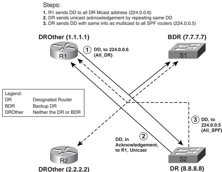
Routers that are not the DR (including the BDR) send DDs to the DR by sending them to multicast address 224.0.0.6, the All OSPF DR Routers multicast address. The DR then acknowledges the DDs with a unicast DD (Step 2 in Figure 10-2). The DR then floods a new DD packet to all OSPF routers (multicast address 224.0.0.5).
