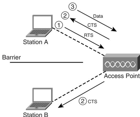
The RTS/CTS function is a handshaking process that minimizes the occurrence of collisions when hidden nodes are operating on the network. In addition, protection mechanisms can use RTS/CTS to avoid collisions between 802.11b and 802.11g radio cards. If hidden nodes are not causing significant retransmissions or hidden nodes are not present, then RTS/CTS is generally not necessary (unless protection mechanisms are in use).
