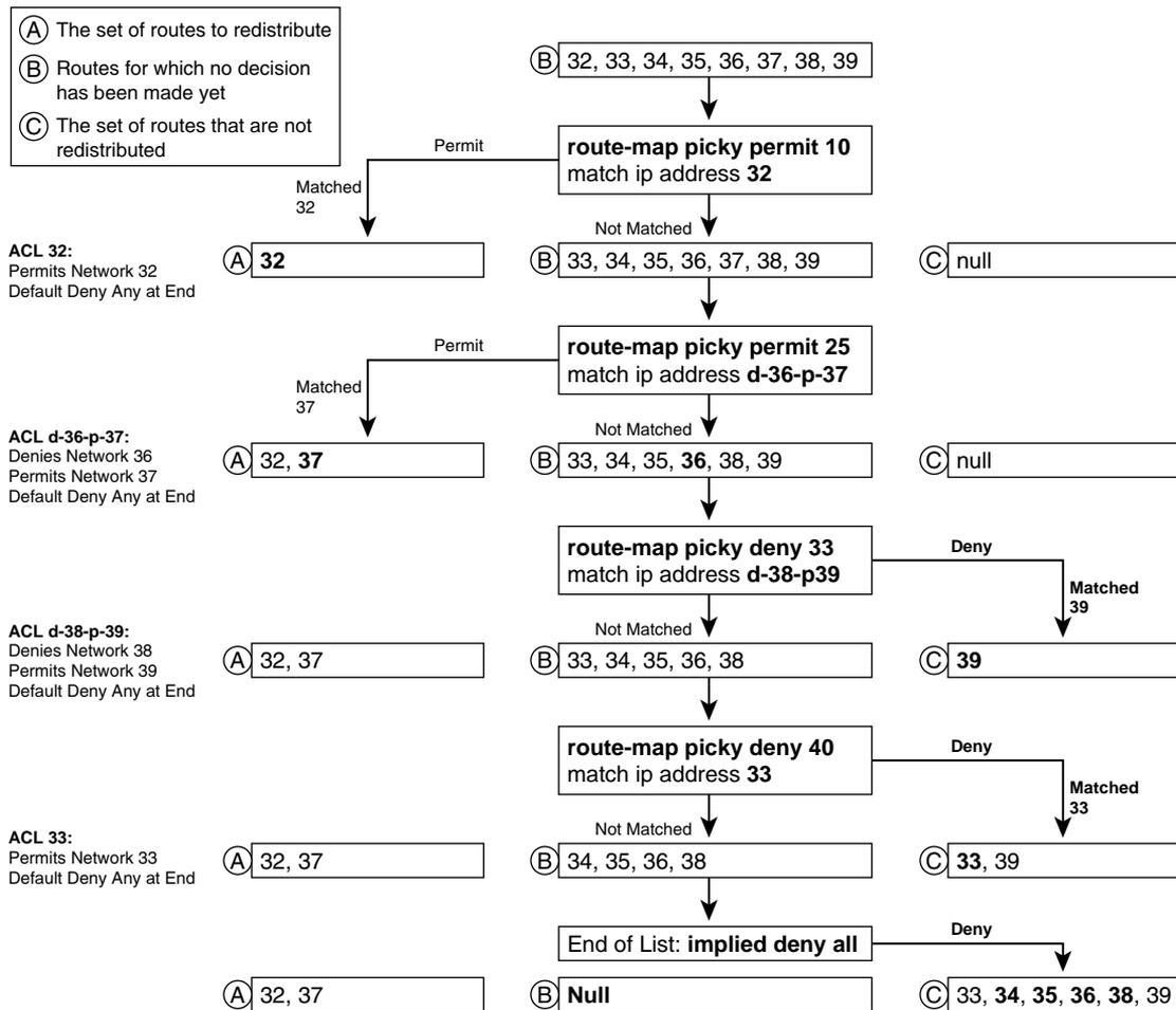
First, a few clarifications about the meaning of Figure 11-1 are in order. The top of the figure begins with the set of connected networks (32 through 39), labeled with a “B,” which is the set of routes still being considered for redistribution. Moving down the figure, four separate **route-map** commands sit inside this single route map. Each **route-map** clause (the clause includes the underlying **match** and **set** commands) in turn moves routes from the list of possible routes (“B”)
