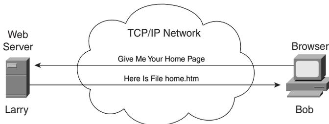
Figure 24-4 shows an example of same-layer interaction. The HTTP protocol is a TCP/IP application layer protocol. The HTTP software on each computer in the figure sits at the same
