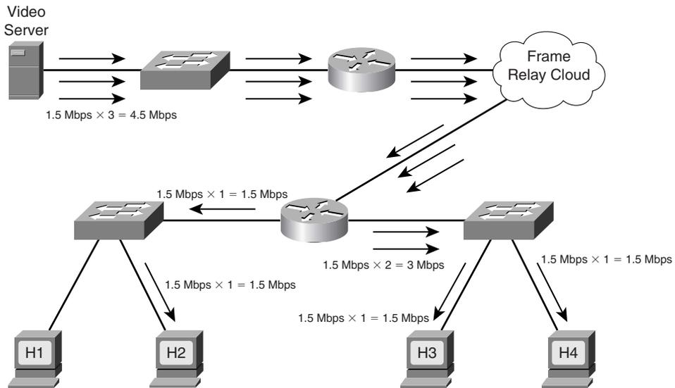
The unicast method requires that the video application send one copy of each packet to every group member's unicast address. To support full-motion, full-screen viewing, the video stream requires about 1.5 Mbps of bandwidth for each receiver. If only a few receivers exist, as shown in Figure 19-1, this method works fine but still requires  $n * 1.5 \text{ Mbps}$  of bandwidth, where  $n$  is the number of receiving hosts.
