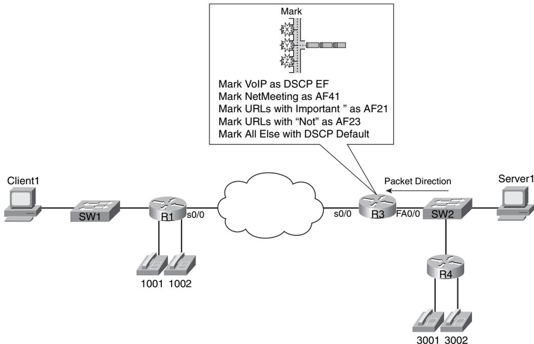
The following criteria define the requirements for marking the various types of traffic for Example 14-3:
