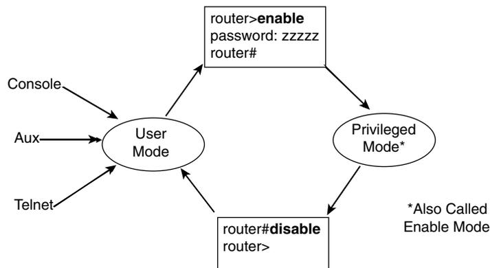
Figure 21-1 shows three methods to reach user mode on a router. The figure also applies to Cisco IOS-based switches, except that Cisco switches do not have auxiliary ports.
