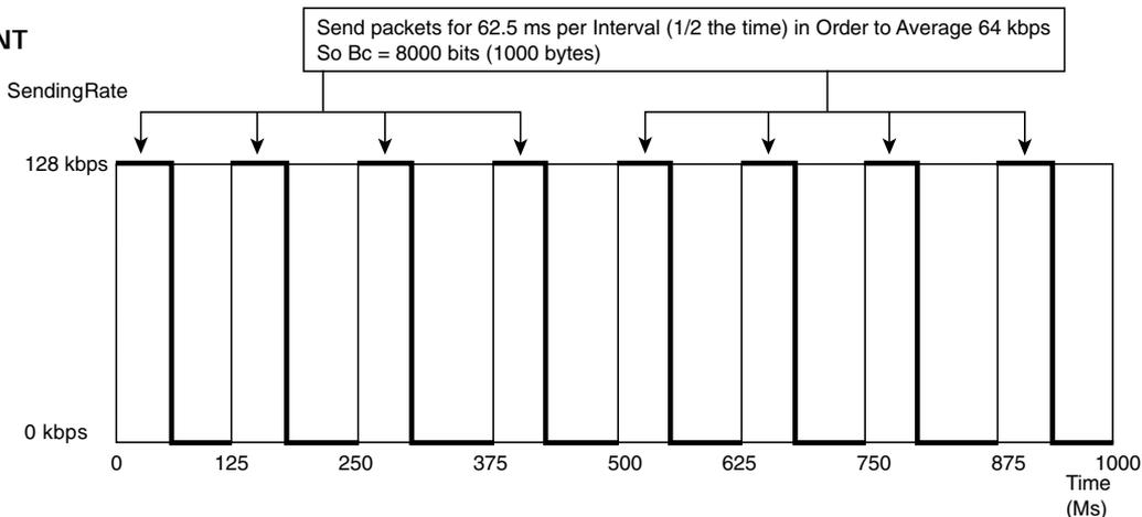
The number of bits that can be sent in each  $T_c$  is called the *committed burst* ( $B_c$ ). In Figure 16-1, an 8000-bit  $B_c$  can be sent in every 125-ms  $T_c$  to achieve a 64-kbps average rate. In other words, with a  $T_c$  of 125 ms, there will be eight  $T_c$  intervals per second. If  $B_c$  bits (8000) are sent each  $T_c$ , then eight sets of 8000 bits will be sent each second, resulting in a rate of 64,000 bps.
