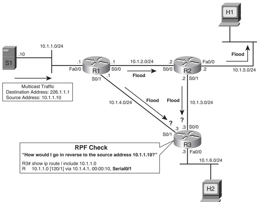
A multicast router does not forward any multicast packet unless the packet passes the RPF check. In Figure 20-3, R3 has to decide whether it should accept the multicast packets coming from R1 and R2. R3 makes this decision by performing the RPF check, described in detail as follows:
