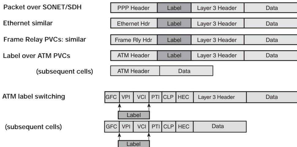
The San Jose router in the example shown in Figure C-10 inserts the MPLS label in front of the IP packet just received, encapsulates the labeled packet in a PPP frame with a PPP Protocol field value of 8281 hex, and forwards the Layer 2 frame toward the San Francisco router.
