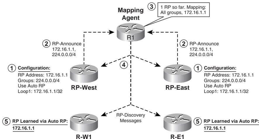
Figure 20-22 shows a design using two RPs (RP-East and RP-West) along with Auto-RP. The steps shown in the figure are as follows:
