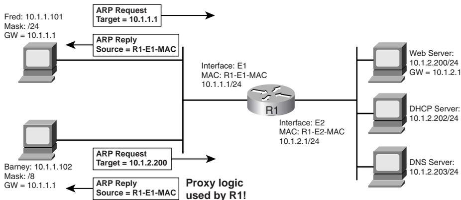
Fred follows a normal ARP process, broadcasting an ARP request, with R1's E1 IP address as the target. The ARP message has a *Target* field of all 0s for the MAC address that needs to be learned, and a target IP address of the IP address whose MAC address it is searching, namely 10.1.1.1 in this case. The ARP reply lists the MAC address associated with the IP address, in this case, the MAC address of R1's E1 interface.
