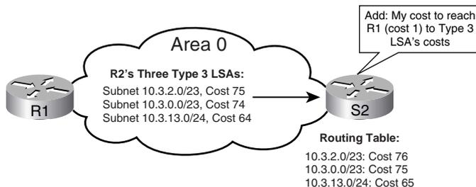
Example 10-5 focuses on the three subnets inside area 3, looking at the type 3 summary LSAs created for those subnets by ABR R1. Note that the example shows commands on S2; S2 has identical area 0 LSDB entries as compared with R1.
