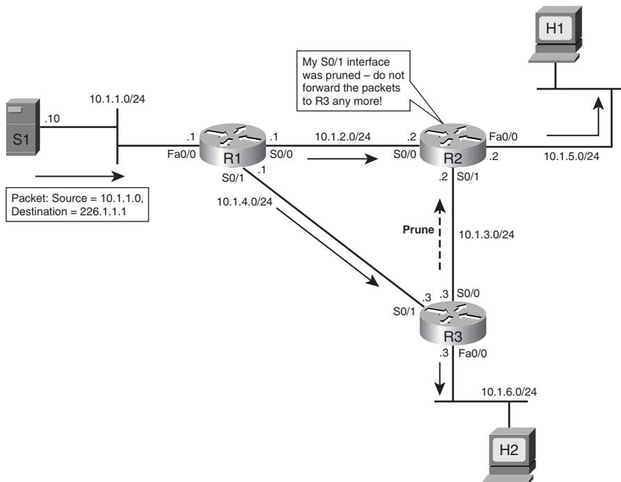
As a result of the Prune message from R3 to R2, R2 will prune its s0/1 interface from the SPT for (10.1.1.10,226.1.1.1). Example 20-2 shows the multicast route table entry for R2 in Figure 20-6, with the line that shows the pruned state highlighted.
