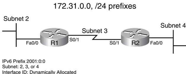
The routers use *dual stacks* (both IPv4 and IPv6 addresses are assigned to the interfaces) for this network. Hosts with dual stacks (running both IPv4 and IPv6) would be able to send IPv4 or IPv6 packets, and the routers could accommodate either. This relatively simple example of IPv6 uses global addresses and a minimal OSPF configuration. Example 4-3 shows the configuration and a working **ping**.
