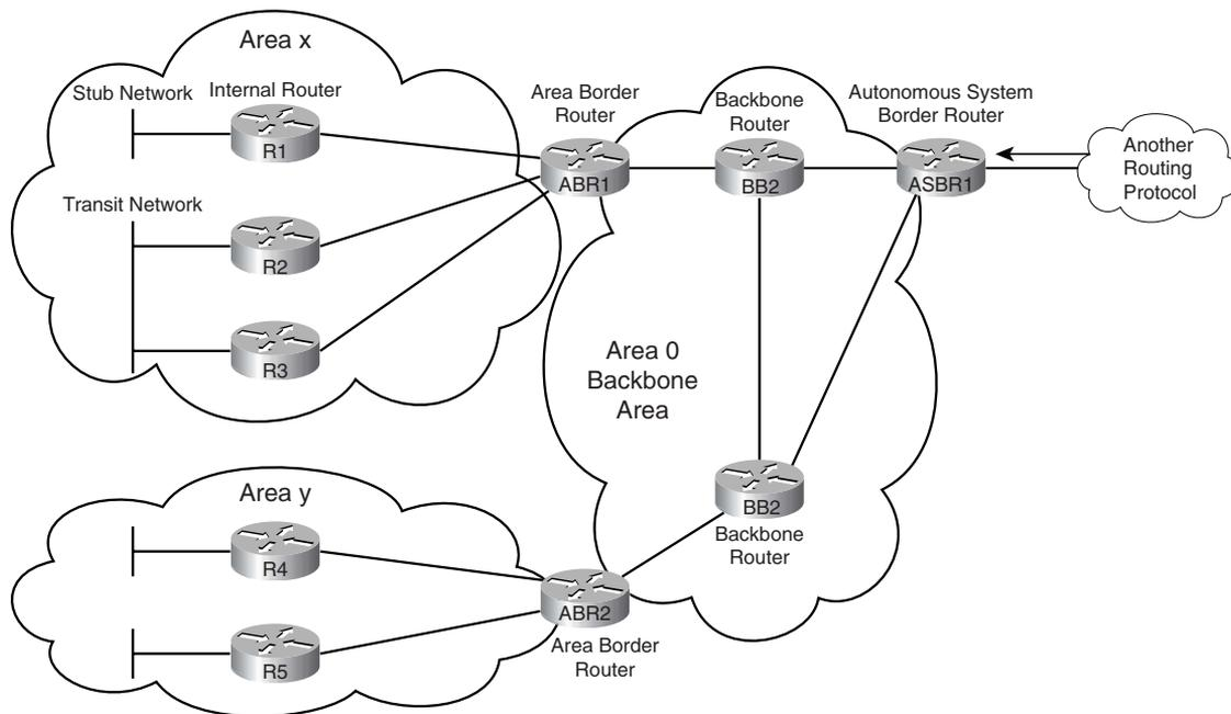
Networks can use a single OSPF area, but using OSPF areas helps speed convergence and reduce overhead in an OSPF network. Using areas provides the following benefits:
