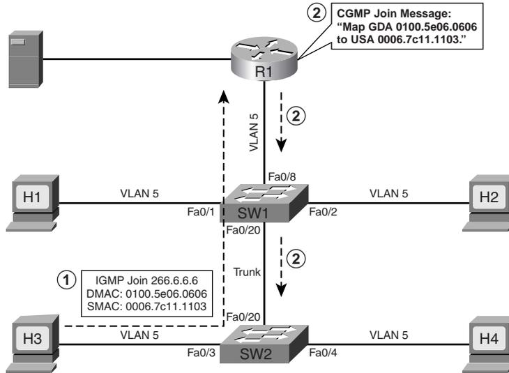
SW1 and SW2 search their CAM table entries and find that a host with the USA 0x0006.7c11.1103 is located on their port number fa0/20 and fa0/3, respectively. Figure 19-18 shows that SW1 and SW2 have mapped the GDA 0x0100.5e06.0606 to their port numbers fa0/20 and fa0/3, respectively.
