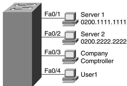
**Example 21-8** *Using Port Security to Define Correct MAC Addresses Connected to Particular Interfaces*
