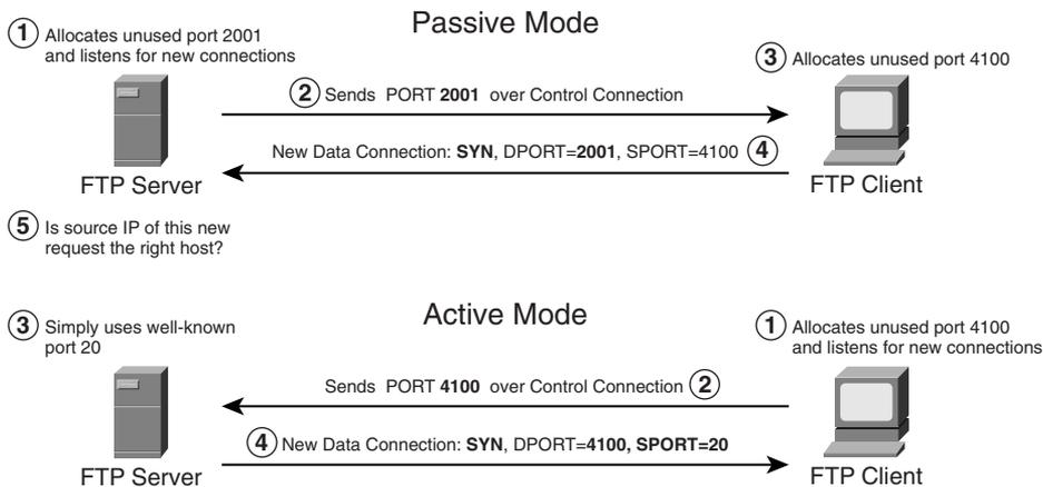
The bottom half of Figure 6-5 shows an active FTP data connection establishment:
