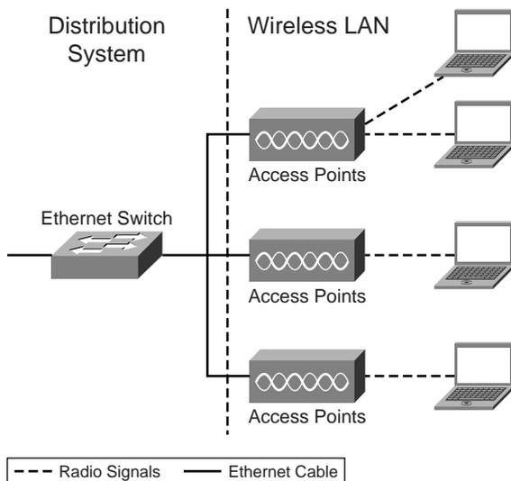
Each access point in the infrastructure wireless LAN creates a radio cell, with a coverage area that depends on the following variables:
