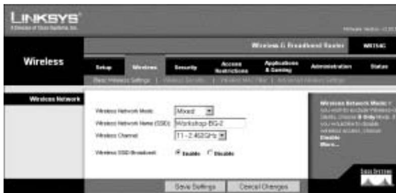
Figure 22-6 Advanced Setup Screen of a Linksys WRT55AG Dual-Band Access Point
