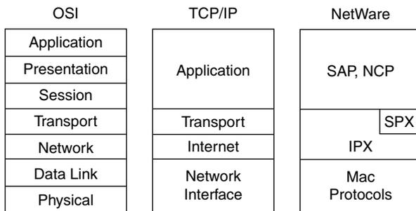
Because the OSI reference model does have a well-defined set of functions associated with each of its seven layers, you can examine any other networking protocol or specification, and make some determination as to whether it most closely matches OSI Layer 1, 2, or 3, and so on. For instance, the TCP/IP Internetwork layer (IP) closely equates to the OSI network layer, hence the use of the terms *network layer protocol* and *Layer 3 protocol* when referring to IP.
