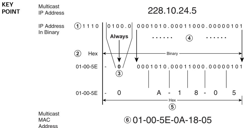
To understand the mechanics of this process, use the following six steps, which are referenced by number in Figure 19-6:
