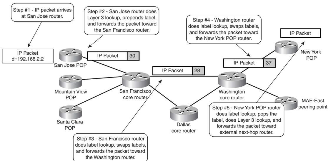
The San Jose POP router receives an IP packet with the destination address of 192.168.2.2 and performs a traditional Layer 3 lookup through the IP forwarding table (also called *Forwarding Information Base [FIB]*).
