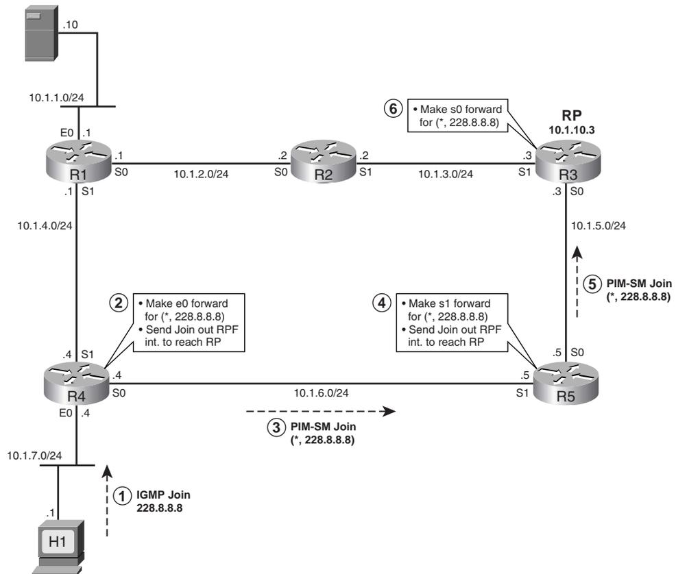
Figure 20-14 shows how H1 causes a shared tree (\*,228.8.8.8) to be created, as described in the following steps:
