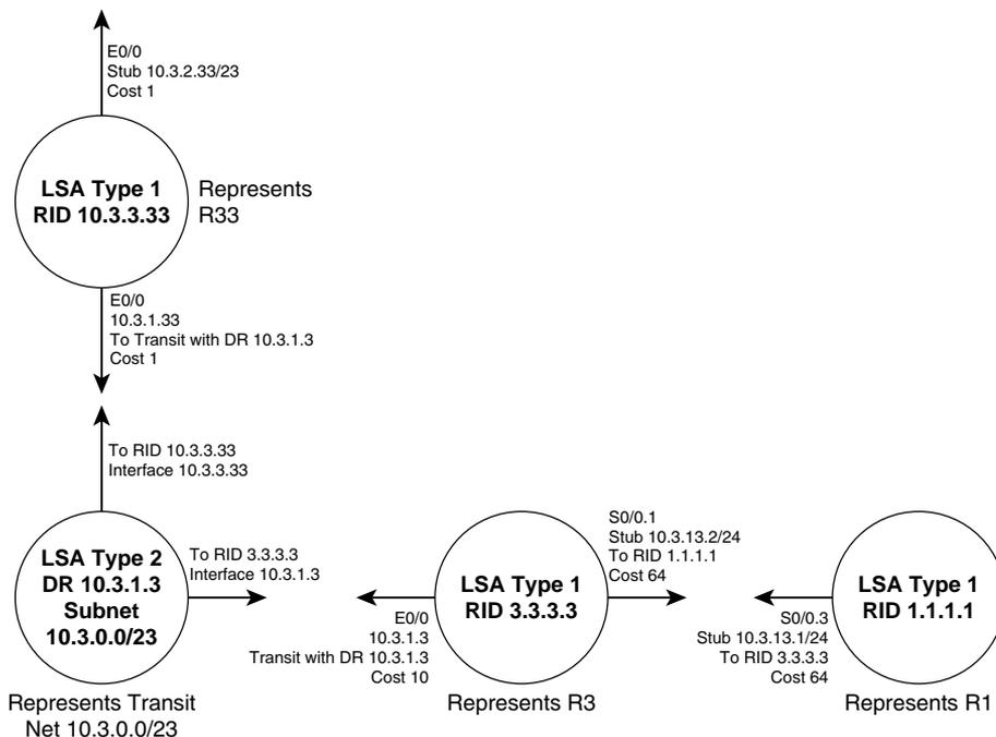
For subnets without a DR, the type 1 LSAs hold enough information for the SPF algorithm to create the math model of the topology. For example, R1 and R3 use point-to-point subinterfaces, and the OSPF point-to-point network type. SPF can match up the information shown in the type 1 LSAs for R1 and R3 in Figure 10-7 to know that the two routers are connected.
