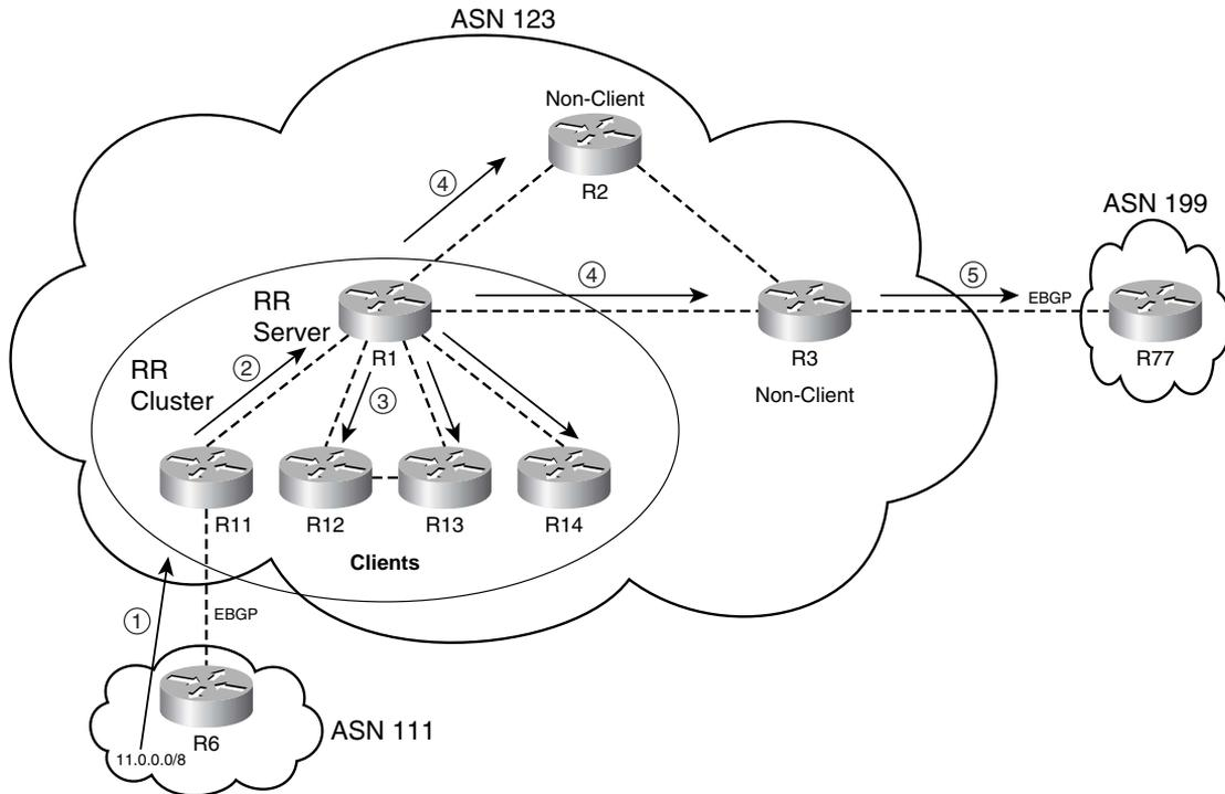
Figure 12-10 shows how prefix 11.0.0.0/8 is propagated through the AS, using the following steps:
