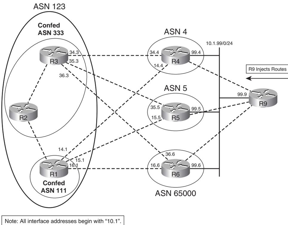
Example 13-4 shows an AS\_PATH filter in which routes are filtered going from R4 to R3. Filtering the outbound Update on R4 will be shown first, followed by filtering of inbound Updates on R3. In both cases, the goal of the filter is as follows:
