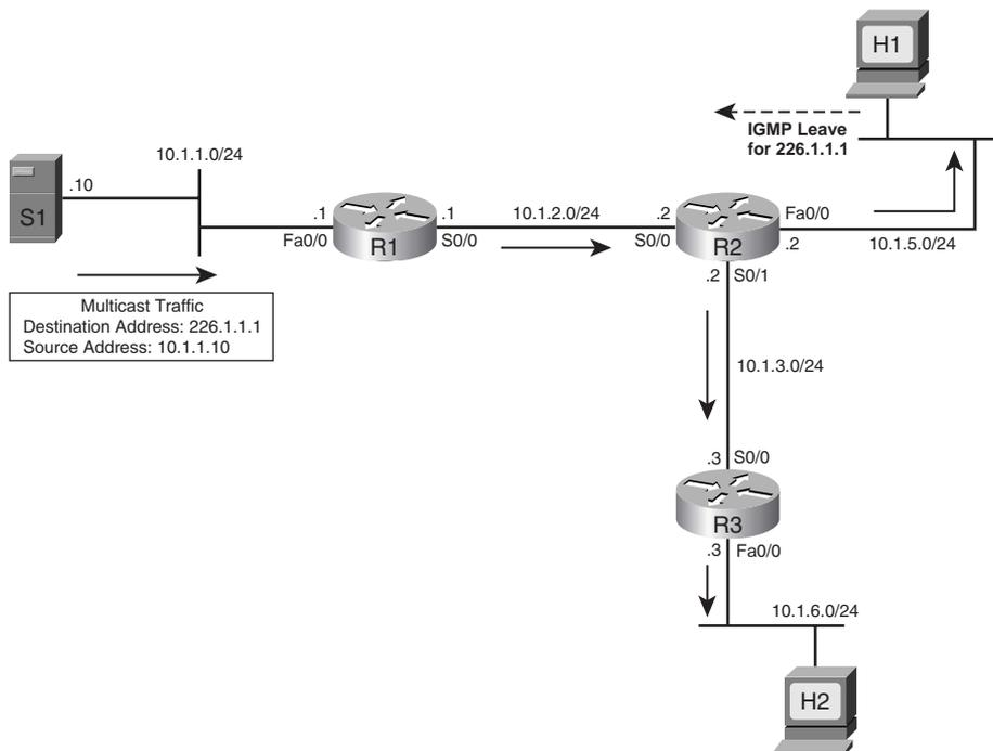
Example 20-3 shows the resulting multicast route table entry for R3 in Figure 20-7. Note that the RPF interface and neighbor IP address has changed to point to R2.
