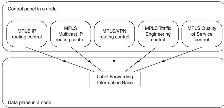
Every MPLS application has the same set of components as the IP routing application:
