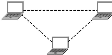
Ad hoc mode is beneficial when a user needs to send a file to another user within the same room, and no other networking is practical. Both users can enable ad hoc mode on their radio cards, and the users can communicate wirelessly. The use of an ad hoc wireless LAN is also valuable when users need to rapidly establish a wireless network when responding to emergencies in areas where no network is in place.
