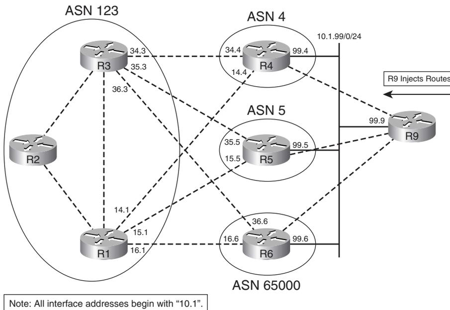
In Example 13-7, R1 sets the weight for NLRI's learned from R4, R5, and R6. The configuration shows both methods of configuring weight:
