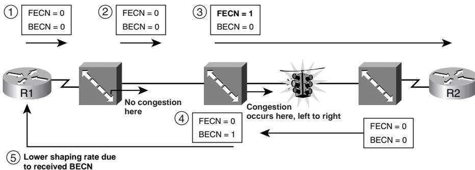
FECN can be set by the FR switches, but not by any of the routers, because the routers do not need to signal forward congestion. For example, if R1 thought congestion was occurring left to right in Figure 18-3, R1 could simply slow down its shaping rate. At the other end of the link, R2 is the destination of the frame, so it would never notice congestion for frames going left to right. So, only the switches need to set FECN.
