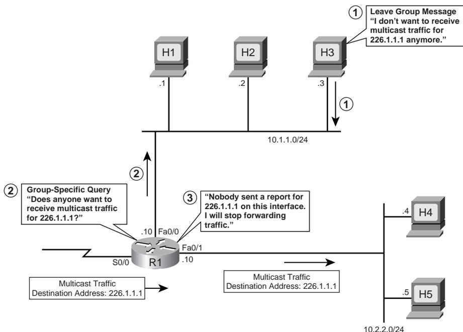
The following three steps, referenced in Figure 19-14, describe the sequence of events for the IGMPv2 Leave mechanism when H3 leaves:
