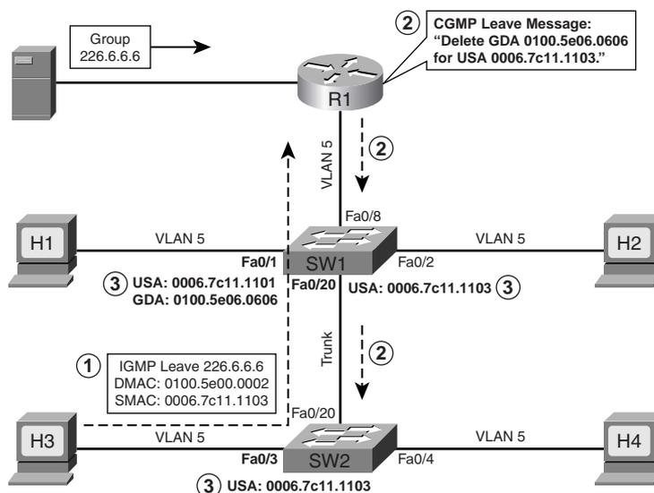
The following three steps, referenced in Figure 19-19, describe the sequence of events when H3 sends an IGMP Leave message:
