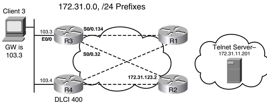
Example 7-4 shows three separate policy routing configurations on Router3. The first configuration forwards Telnet traffic over the PVC to Router2 (next hop 172.31.123.2). The next configuration does the same thing, but this time using the **set interface** command. The final option shows a nonworking case with Router3 specifying its LAN interface as an outgoing interface.
