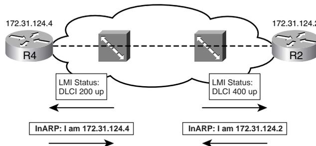
Unlike on LANs, a packet does not need to arrive at the router to trigger the InARP protocol; instead, an LMI status message triggers InARP. After receiving an LMI PVC Up message, each router announces its own IP address over the VC, using an InARP message, as defined in RFC 1293. Interestingly, if you disable LMI, then the InARP process no longer works, because nothing triggers a router to send an InARP message.
