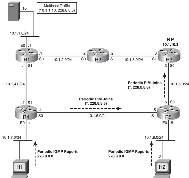
Example 20-8 shows the multicast route table entry for R5 in Figure 20-16, with these two interfaces in a forwarding state.
