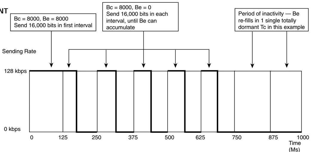
In the first interval, traffic shaping can send a total of 16,000 bits (Bc + Be bits). On a 128-kbps link, assuming a 125-ms Tc, all 125 ms is required to send 16,000 bits. In this particular case, after a period of inactivity, R1 sends continuously for the entire first interval. In the second interval, the shaper allows the usual Bc bits to be sent. In effect, with these settings, the shaper allows 192.5 ms of consecutive sending after a period of low activity.
