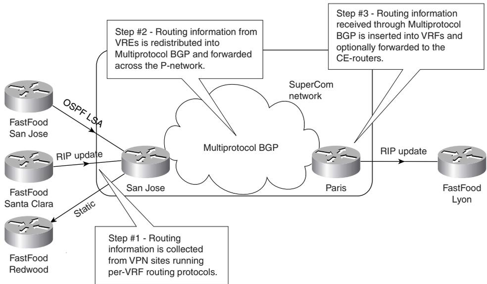
**WARNING** The redistribution of the per-VPN routing information into MP-BGP is not automatic and must be manually configured on the router for each VRF, unless this information was learned from the customer via BGP. The omission of manual redistribution into MP-BGP is one of the most common configuration errors in MPLS/VPN deployment.
