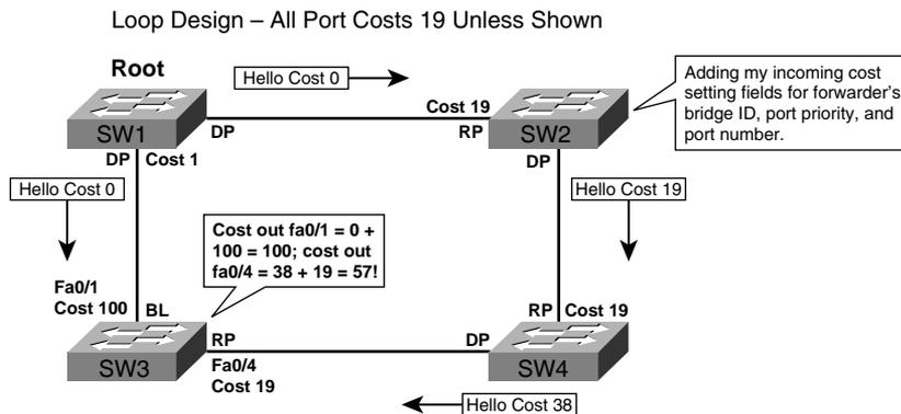
In Figure 3-2, SW1 happened to become root, and is originating Hellos of cost 0. SW3 receives two Hellos, one with cost 0 and one with cost 38. However, SW3 must then calculate its cost to reach the root, which is the advertised cost (0 and 38, respectively) plus SW3's port costs (100 and 19, respectively). As a result, although SW3 has a direct link to SW1, the calculated cost is lower
