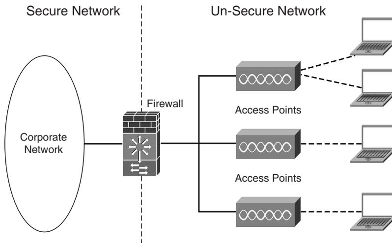
Most installations should try to limit propagation of radio signals outside the facility. As a precaution, consider designing the wireless LAN in a way that limits radio signals from being received outside the facility. This minimizes the ability for a hacker to associate with one of the wireless LAN access points. A company can reduce radio propagation outside the building by properly aligning antennas and reducing the transmit power of access points.
