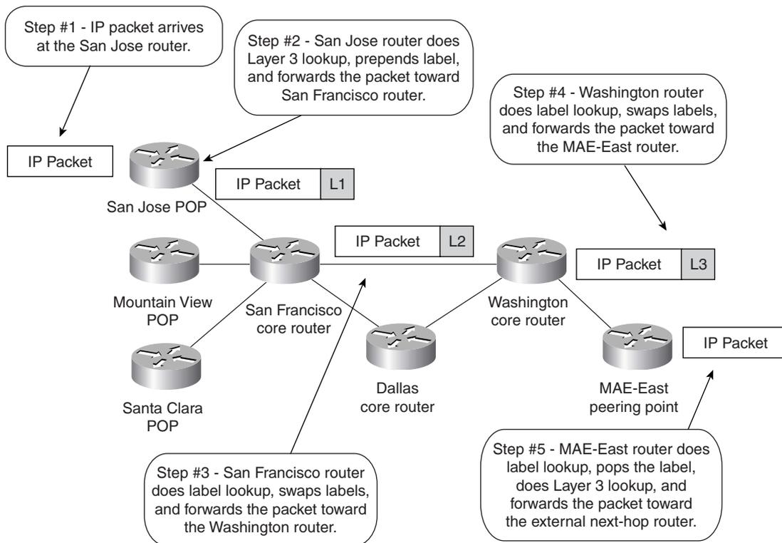
The creation of the LSP is a connection-oriented scheme because the path is set up prior to any traffic flow. However, this connection setup is based on topology information rather than a requirement for traffic flow. This means that the path is created regardless of whether any traffic actually is required to flow along the path to a particular set of FECs.
