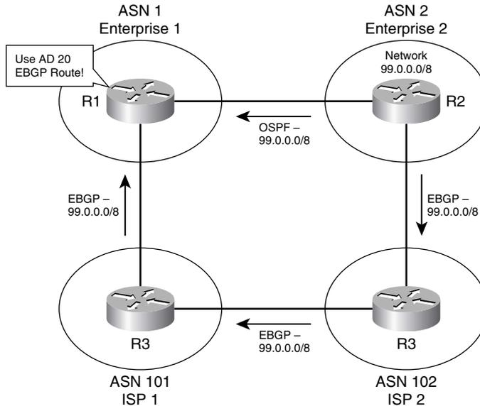
R1 uses its eBGP route to reach 99.0.0.0 because eBGP has a lower AD (20) than OSPF (110). One solution would be to configure the **distance** command to lower the AD of the OSPF-learned route. However, BGP offers an elegant solution to this particular problem through the use of the **network backdoor** command. In this case, if R1 configures the **network 99.0.0.0 backdoor** router BGP subcommand, the following would occur:
