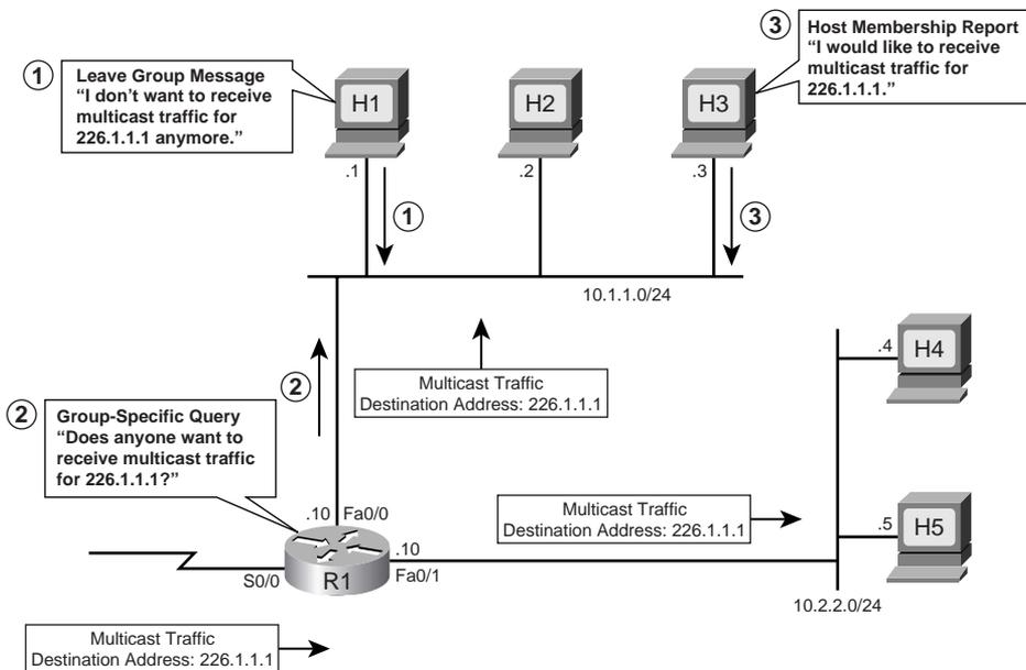
The following three steps, referenced in Figure 19-13, describe the sequence of events for the IGMPv2 Leave mechanism when H1 leaves:
