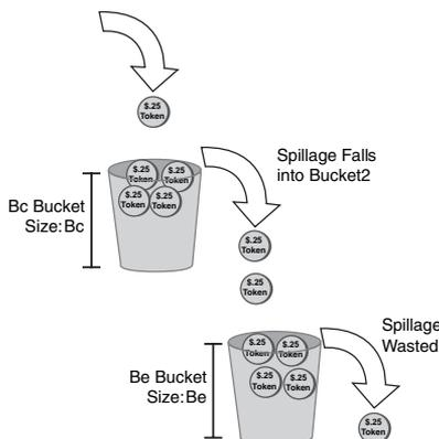
After filling the buckets, the policer then determines the category for the newly arrived packet, as shown in Table 16-6. In this case,  $X_{bc}$  is the number of tokens in the Bc bucket, and  $X_{be}$  is the number in the Be bucket.
