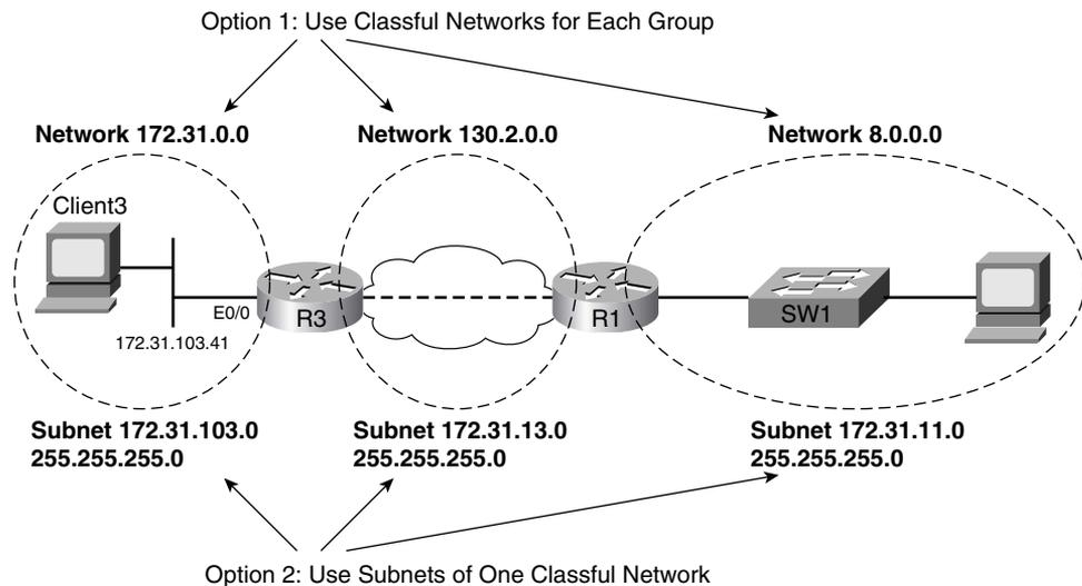
Option 1 uses three classful networks; however, it wastes a lot of IP addresses. For example, all hosts in class A network 8.0.0.0 must reside on the LAN on the right side of the figure.
