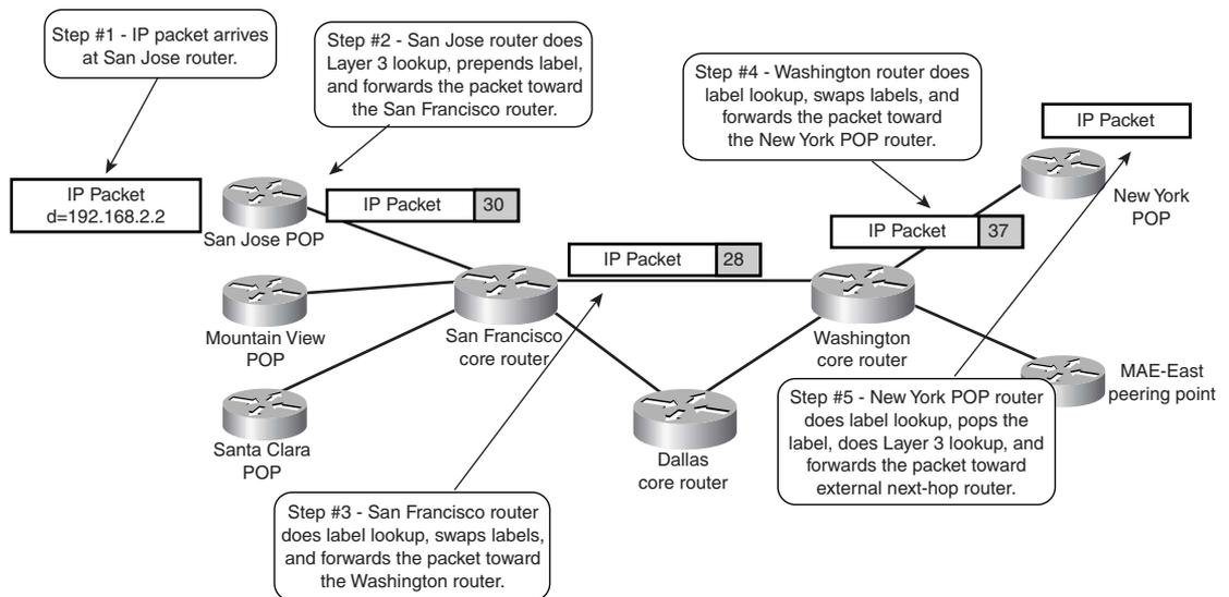
The double lookup in the New York POP router might reduce the performance of that node. Furthermore, in environments where MPLS and IP switching is realized in hardware, the fact that a double lookup might need to be performed can increase the complexity of the hardware implementation significantly. To address both issues, *penultimate hop popping (PHP)* was introduced into the MPLS architecture.
