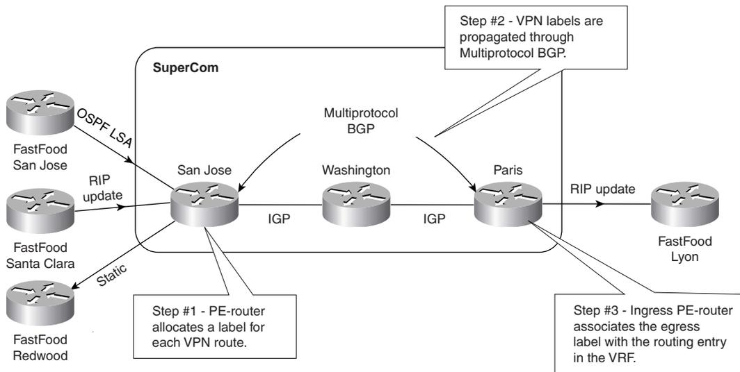
The egress PE-router receives the labeled packet, drops the first label, and performs a lookup on the second label, which uniquely identifies the target VRF and sometimes even the outgoing interface on the PE-router. A lookup is performed in the target VRF (if needed), and the packet is sent toward the proper CE-router.
