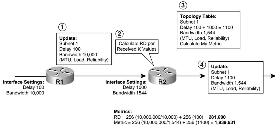
Because the received update includes the neighbor's metric components, a router can calculate the advertising neighbor's metric for a route—called the *reported distance (RD)*. A router can, of course, also calculate its own metric for a particular route, after adding its own interface delay and considering whether it should adjust the value for the constraining bandwidth. For example, consider the four steps outlined in Figure 9-3:
