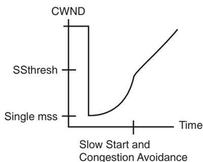
The graph shows the changes to CWND from connection establishment through multiple segment loss. Because multiple segments were lost, the TCP sender halved CWND multiple times, and in this case, CWND was lowered to its minimum value—a single MSS. Before lowering CWND, the sender calculated a variable called *Slow Start Threshold* (SStresh), which is half of the original CWND before segments were lost.
