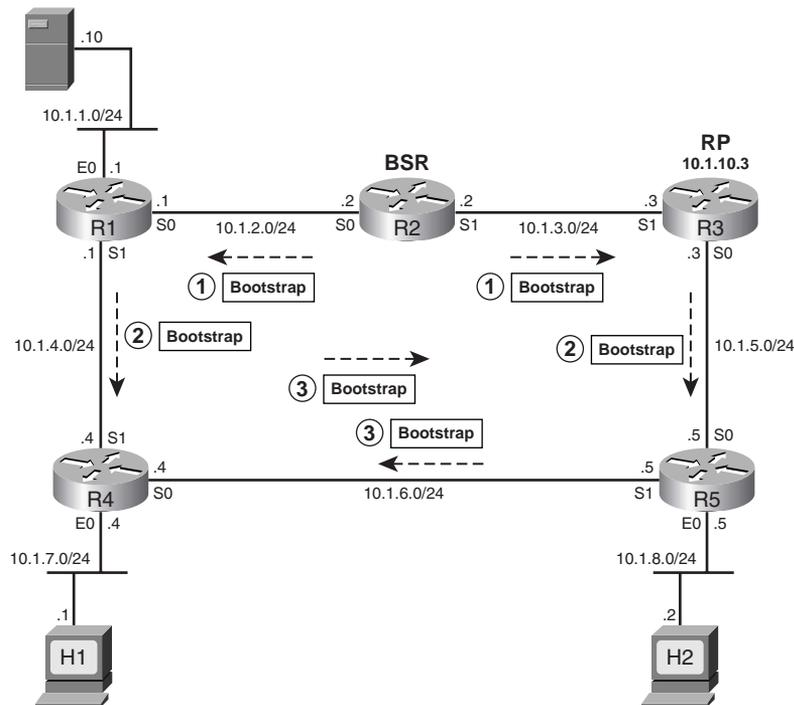
The other important part of BSR operation is for each candidate RP (c-RP) to inform the BSR router that it is an RP and to identify the multicast groups it supports. This part of the process with BSR is simple if you keep in mind the following point:
