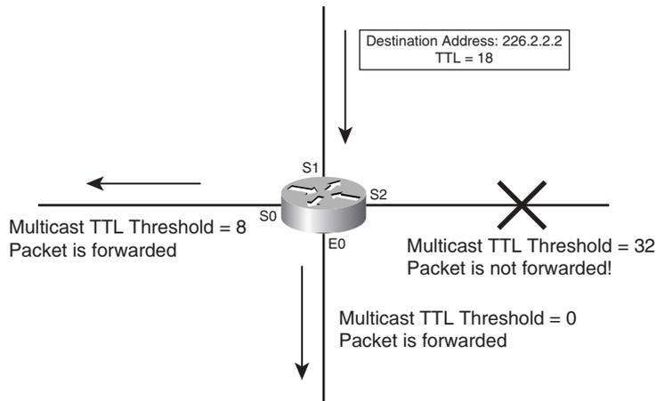
On the s0 and s2 interfaces in Figure 20-5, the network administrator has configured the TTL as 8 and 32, respectively. A copy of the packet is forwarded on the s0 and e0 interfaces because their TTL thresholds are less than 17. However, the packet is not forwarded on the s2 interface because its TTL threshold is 32, which is higher than 17.
