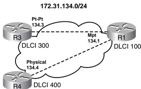
**NOTE** All figures with Frame Relay networks in this book use Global DLCI conventions unless otherwise stated. For instance, in Figure 7-3, DLCI 300 listed beside Router3 means that, due to Local DLCI assignment conventions by the service provider, all other routers (like Router4) use DLCI 300 to address their respective VCs back to Router3.
