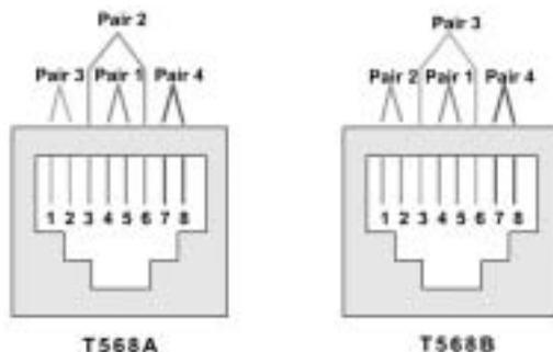
The most popular Ethernet standards (10BASE-T, 100BASE-T, and 1000BASE-T) each use two twisted pairs (specifically pairs 2 and 3 shown in Figure 1-1), with one pair used for transmission in each direction. Depending on which pair a device uses to transmit and receive, either a straight-through or cross-over cable is required. Table 1-2 summarizes how the cabling and pinouts work.
