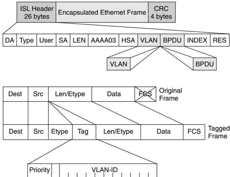
Finally, the last row from Table 2-7 refers to the *native VLAN*. 802.1Q does not tag frames sent inside the native VLAN. The native VLAN feature allows a switch to attempt to use 802.1Q trunking on an interface, but if the other device does not support trunking, the traffic for that one native VLAN can still be sent over the link. By default, the native VLAN is VLAN 1.
