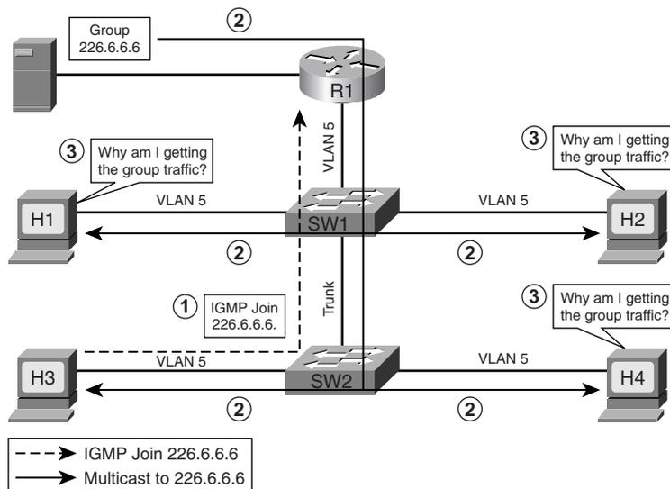
Hosts H1, H2, H3, H4, and R1 are all in the same broadcast domain of VLAN 5. The following three steps, referenced in Figure 19-16, describe the sequence of events when H3 sends an IGMP Join message:
