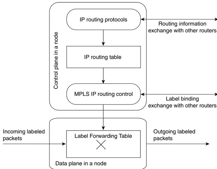
Every MPLS node must run one or more IP routing protocols (or rely on static routing) to exchange IP routing information with other MPLS nodes in the network. In this sense, every MPLS node (including ATM switches) is an IP router on the control plane.
