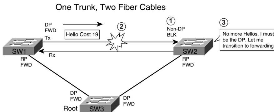
Figure 3-9 shows the fiber link between SW1 and SW2 with both cables. SW2 starts in a blocking state, but as a result of the failure on SW1's transmit path, SW2 ceases to hear Hellos from SW1. SW2 then transitions to forwarding state, and now all trunks on all switches are forwarding. Even with the failure of SW1's transmit cable, frames will now loop counter-clockwise in the network.
