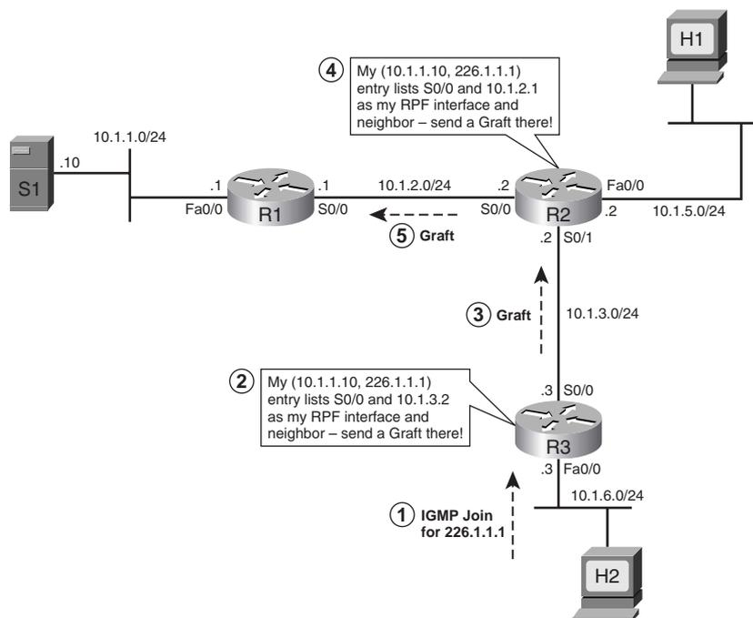
Without the Graft message, host H2 would have to wait for as much as 3 minutes before it would receive the group traffic. However, with the following steps, as listed in Figure 20-10, H2 will receive the packets in just a few seconds:
