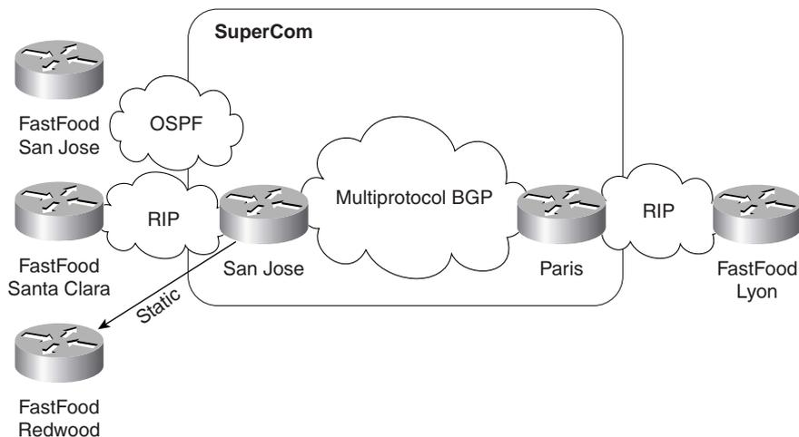
The San Jose PE-router collects routing information from the San Jose site using a per-VPN OSPF process. Similarly, the information from the Santa Clara site is collected using a per-VPN RIP process. This process is marked as Step 1 in Figure 8-7.
