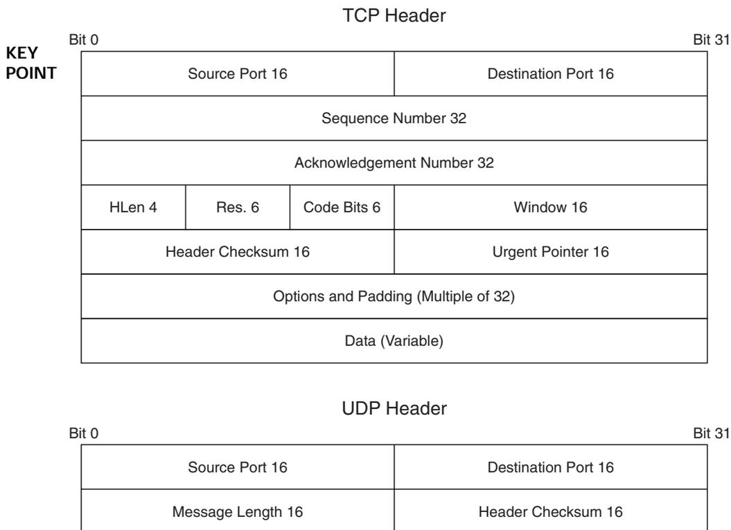
Note that UDP operates identically to TCP in regard to the Port Number fields and the Header Checksum field. The UDP Length field identifies the length of the UDP message, including the UDP header and data. The fields inside the TCP header are explained in the next few sections of this chapter.
