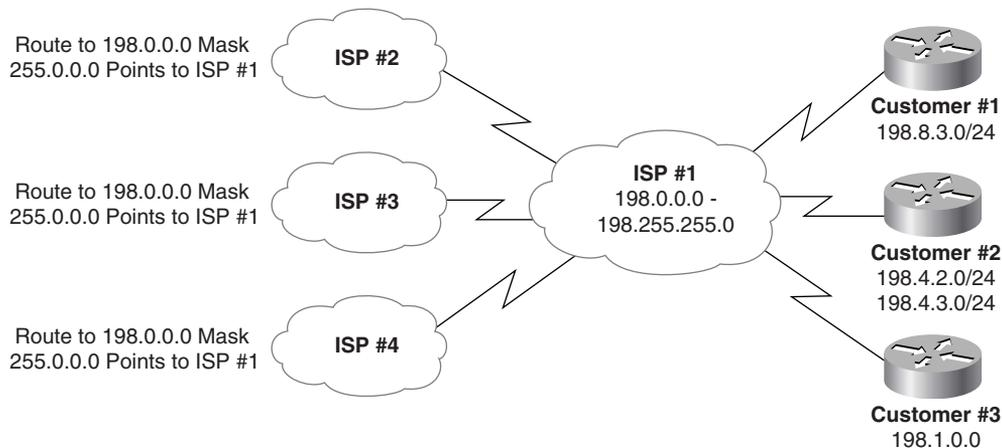
ISPs 2, 3, and 4 need only one route (198.0.0.0/8) in their routing tables to be able to forward packets to all destinations that begin with 198. Note that this summary actually summarizes multiple class C networks—a typical feature of CIDR. ISP 1's routers contain more detailed routing entries for addresses beginning with 198, based on where they allocate IP addresses for their customers. ISP 1 would reduce its routing tables similarly with large ranges used by the other ISPs.
