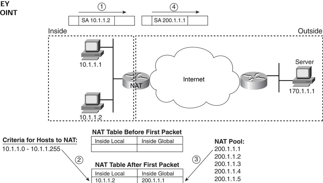
With the completion of step 3, the NAT router can actually translate the source IP address, and forward the packet. Note that as long as the dynamic NAT entry exists in the NAT table, only host 10.1.1.2 can use Inside Global IP address 200.1.1.1.
