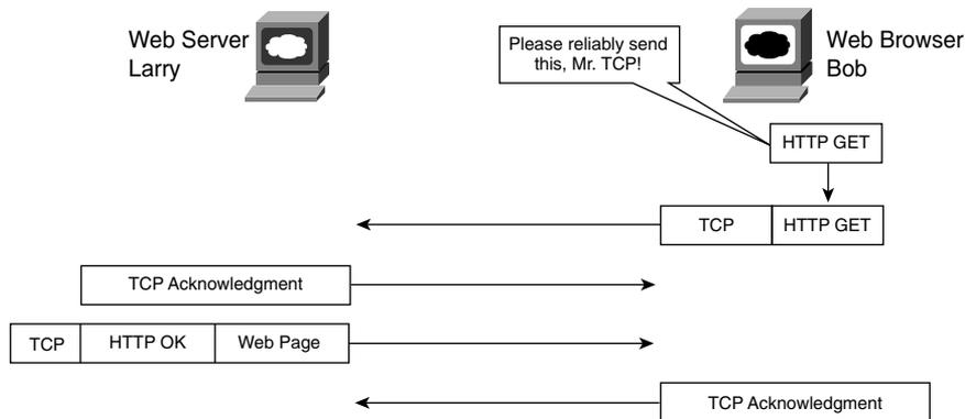
This example outlines the concepts of how protocols in adjacent layers, and on the same computer, work together. In this case, the higher-layer protocol (HTTP) needed to do something it could not do (error recovery), so it asked the next-lower-layer protocol (TCP) for help. TCP provided a guaranteed delivery service to HTTP. The interaction between these adjacent layers is aptly called *adjacent-layer interaction*.
