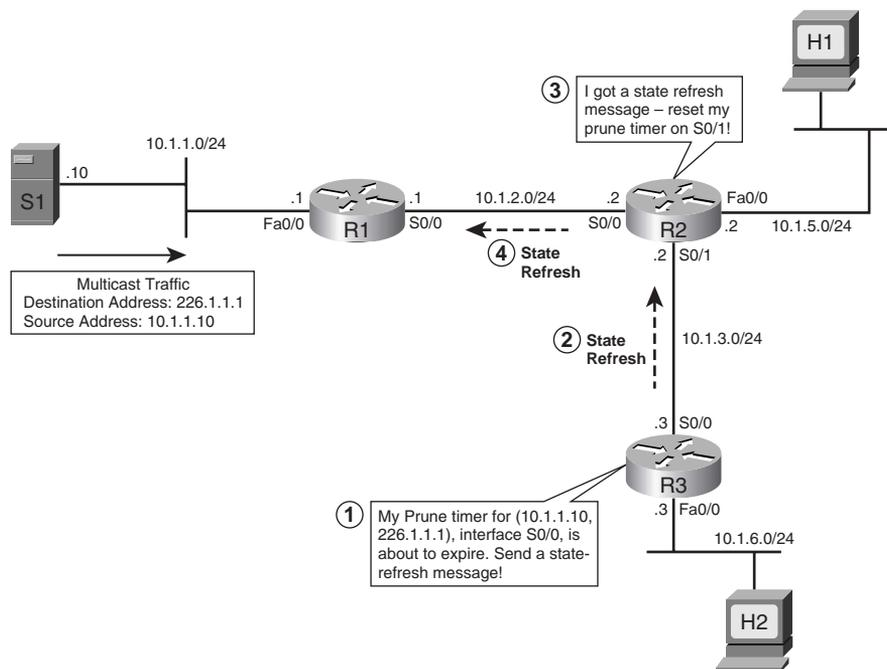
The PM State Refresh message can be sent, just before a neighbor's Prune timer expires, to keep the interface in a pruned state. In Figure 20-9, the following steps do just that:
