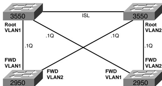
With different root switches and with default port costs, the access layer switches end up sending VLAN1 traffic over one uplink and VLAN2 traffic over another uplink.
