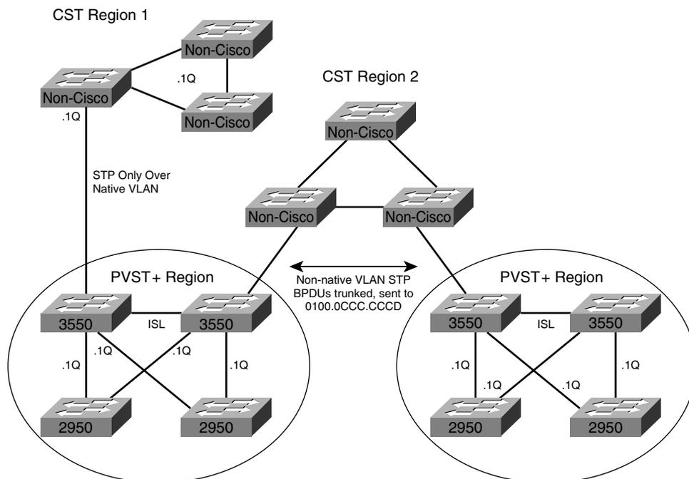
The left side of Figure 3-5 shows an example in which the CST region is not used for transit between multiple PVST+ regions. In this case, none of the PVST+ per-VLAN STP information needs to pass over the CST region. The PVST+ region maps the single CST instance to each of the PVST+ STP instances.
