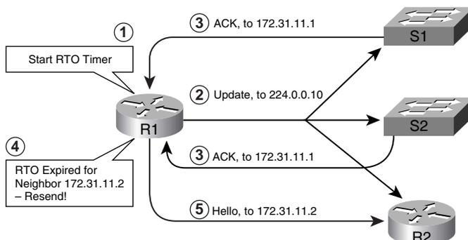
RTP allows the Updates to be sent as multicasts. If any neighbors fail to acknowledge receipt of the multicasted update, RTP resends Updates as unicasts just to those neighbors. The steps run as follows, using Figure 9-2 as an example:
