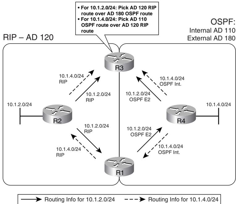
Example 11-4 shows how to configure both R1 and R3 to use a different AD for external routes by using the **distance ospf external 180** command, under the **router ospf** process.
