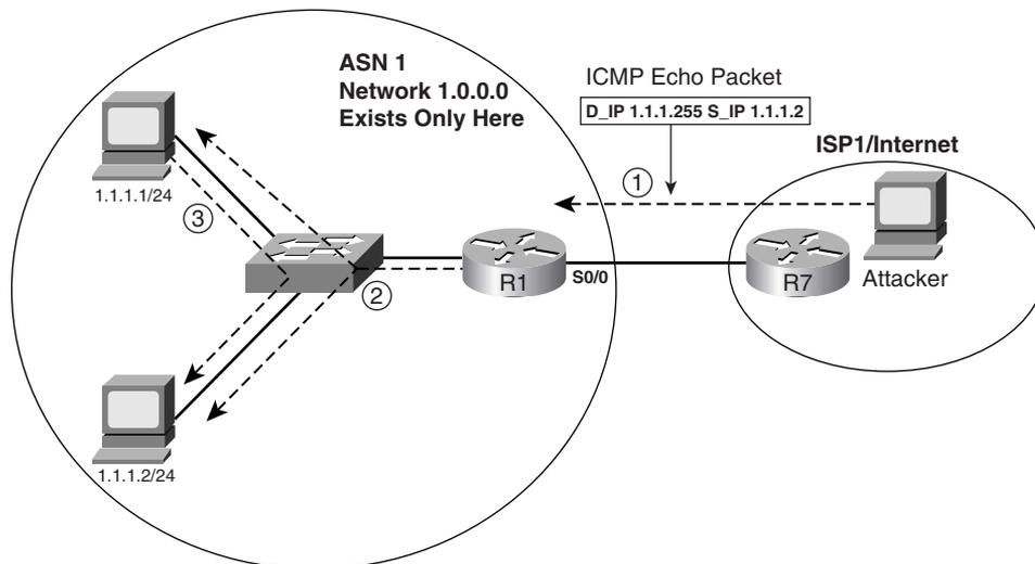
1. Attacker sends packet destined to subnet broadcast, source 1.1.1.2 (for secondary attack).
