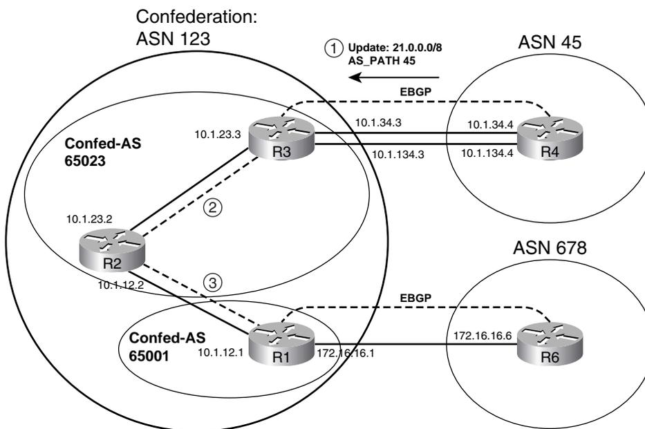
In this internetwork topology, R1 is in sub-AS 65001, with R2 and R3 in sub-AS 65023. In this case, R1 and R3 will not be neighbors. The following list outlines the sequence of events to propagate a prefix:
