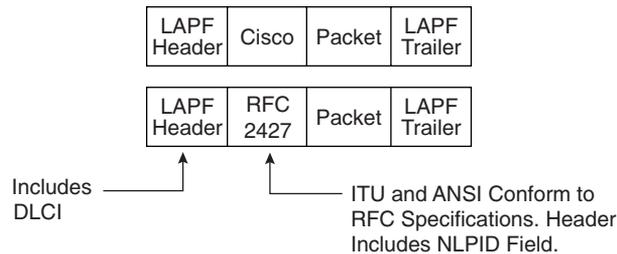
Each VC uses the Cisco encapsulation header unless configured explicitly to use the IETF header. Three methods can be used to configure a VC to use the IETF-style header:
