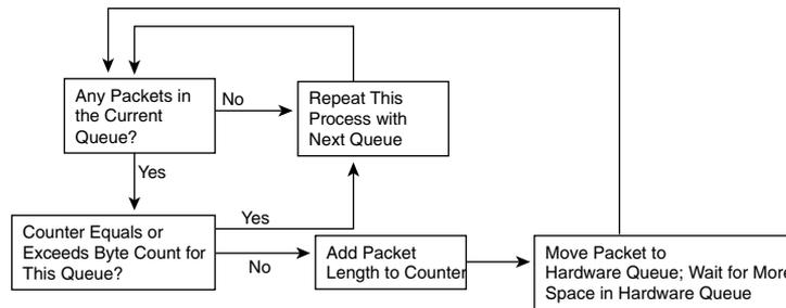
The CQ scheduler performs round-robin service on each queue, beginning with queue 1. CQ takes packets from the queue, until the total byte count specified for the queue has been met or exceeded. After the queue has been serviced for the defined byte count, or when the queue does not have any more packets, CQ moves on to the next queue and repeats the process.
