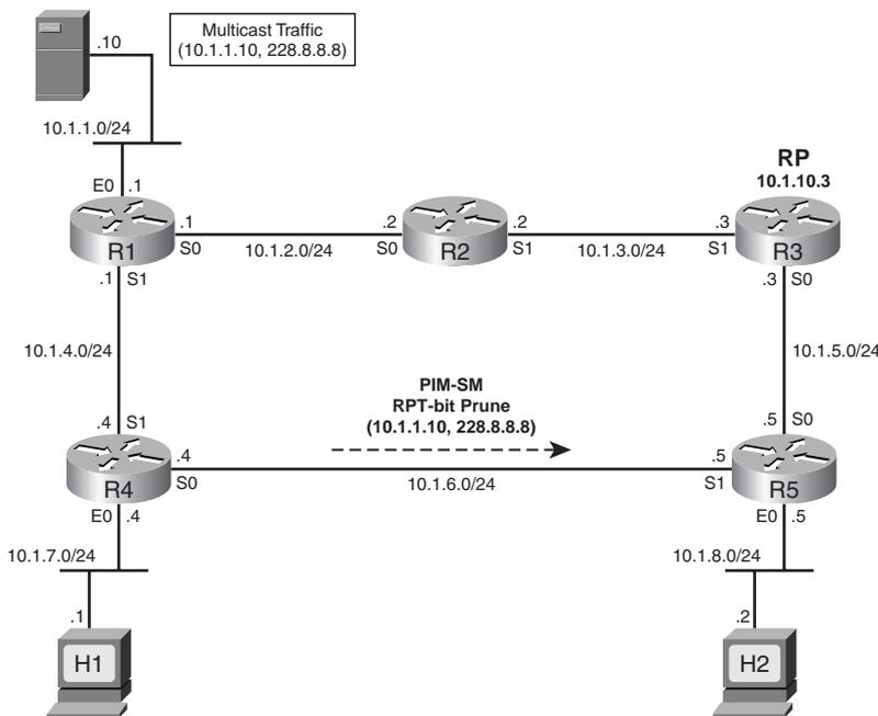
To stop the packets from being sent over the RPT to R4, R5 must prune its interface s1 in the RPT (\*, 228.8.8.8). R5 may go on to join the SPT for (10.1.1.10, 228.8.8.8) as well.
