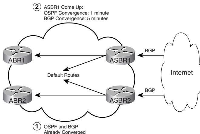
Both ASBR1 and ASBR2 advertise defaults into the network, expecting to have the capability to route to the Internet through BGP-learned routes. In this case, ASBR2 is already up, fully converged. However, if ASBR1 reloads, when it comes back up, OSPF is likely to converge faster than BGP. As a result, ASBR1 will advertise its default route, and OSPF routers may send packets to ASBR1, but ASBR1 will end up discarding the packets until BGP converges.
