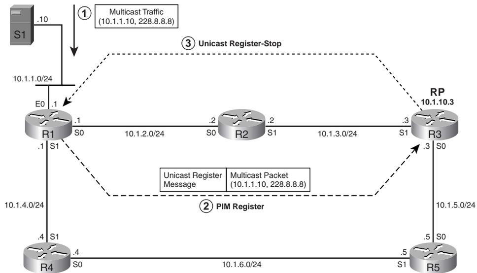
The following three steps, referenced in Figure 20-13, describe the sequence of events for the Source Registration process when the RP has not received a request for the group from any PIM-SM router because no host has yet joined the group.
