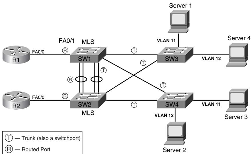
Figure 7-5 Layer 3 Topology View: Example Using MLS
