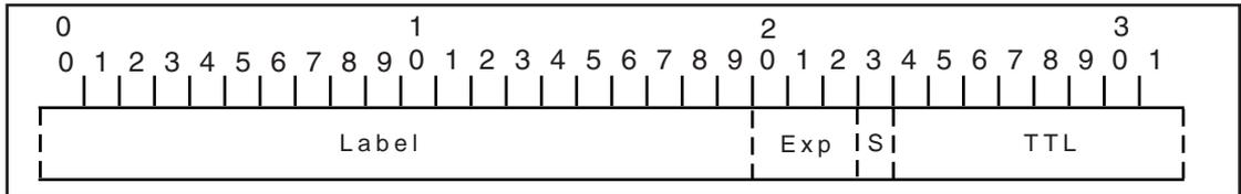
The Bottom-of-Stack bit implements an MPLS label stack, which is defined as a combination of two or more label headers attached to a single packet. Simple unicast IP routing does not use the label stack, but other MPLS applications, including MPLS-based Virtual Private Networks or MPLS Traffic Engineering, rely heavily on it.
