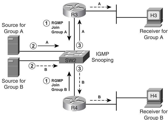
Figure 19-23 shows the following three main steps, with the first step really showing the RGMP function with the RGMP Join message. The Join message allows a router to identify the groups for which the router wants to receive traffic.
