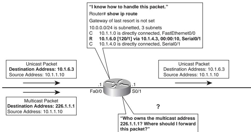
Figure 20-1 shows that the router has received a multicast packet with the destination address 226.1.1.1. The destination address represents a dynamically changing group of recipients, not any one recipient's address. How can the router find out where these users are? Where should the router forward this packet?
