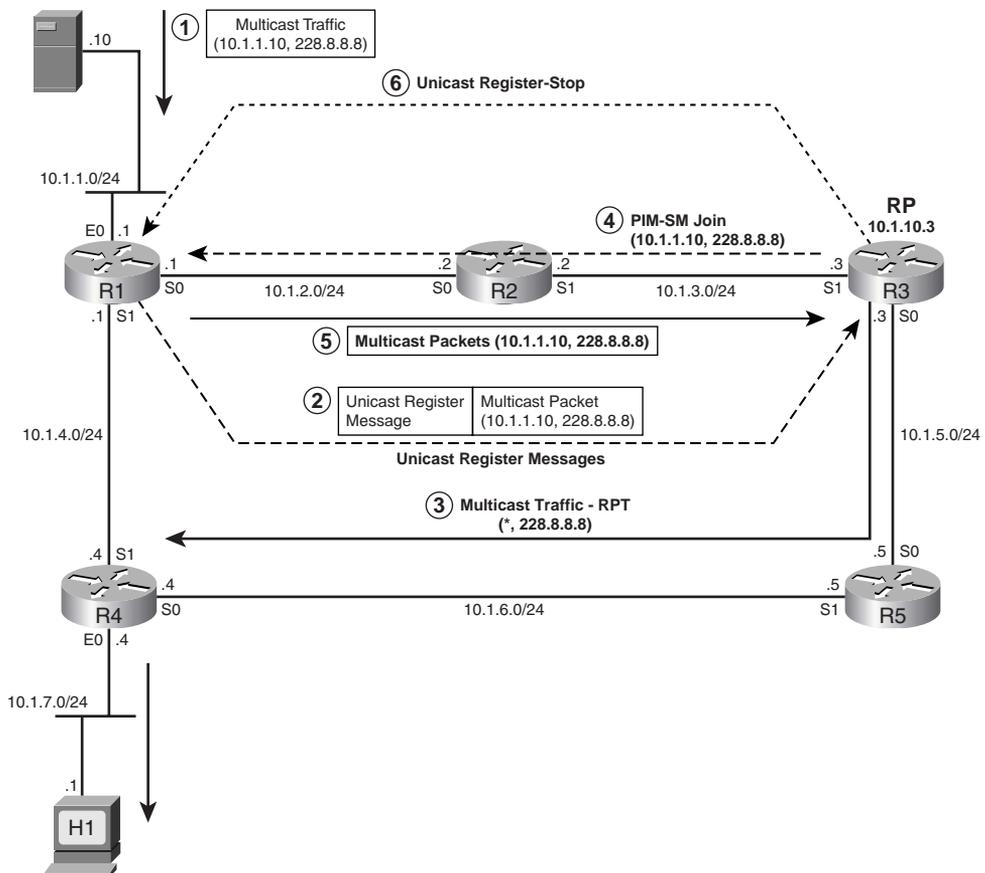
The process may seem like a lot of trouble, but at the end of the process, multicasts are delivered to the correct locations. The process uses the efficient SPT from the source to the RP, and the shared tree (\*,228.8.8.8) from the RP to the subnets that need to receive the traffic.
