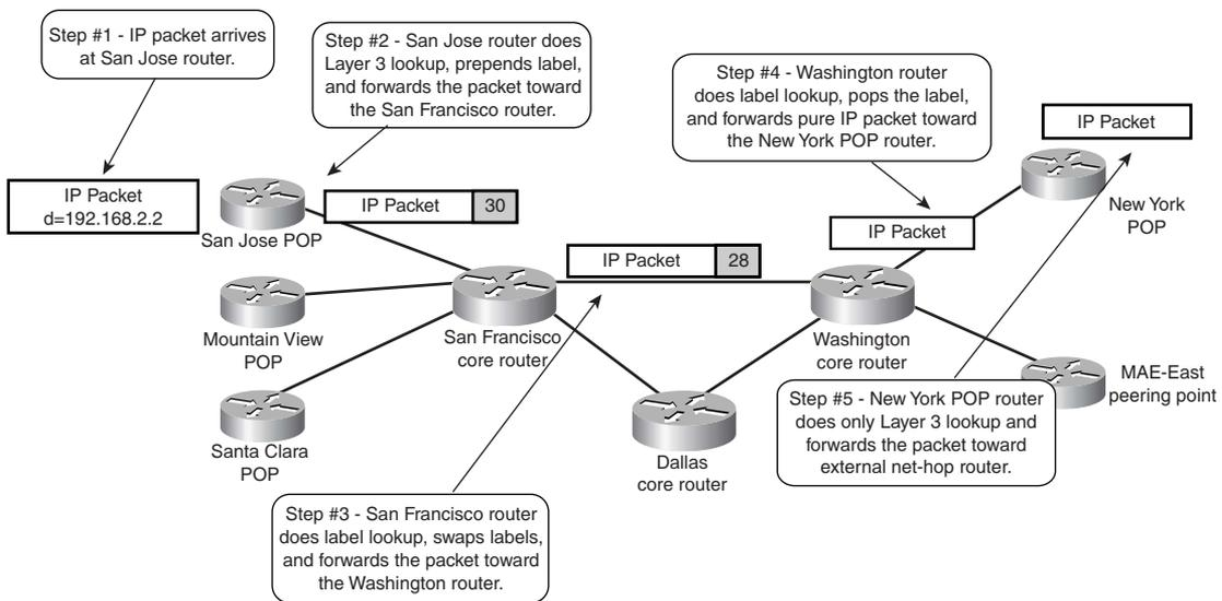
Penultimate hop popping is requested through TDP or LDP by using a special label value (1 for TDP, 3 for LDP) that also is called the *implicit-null* value.
