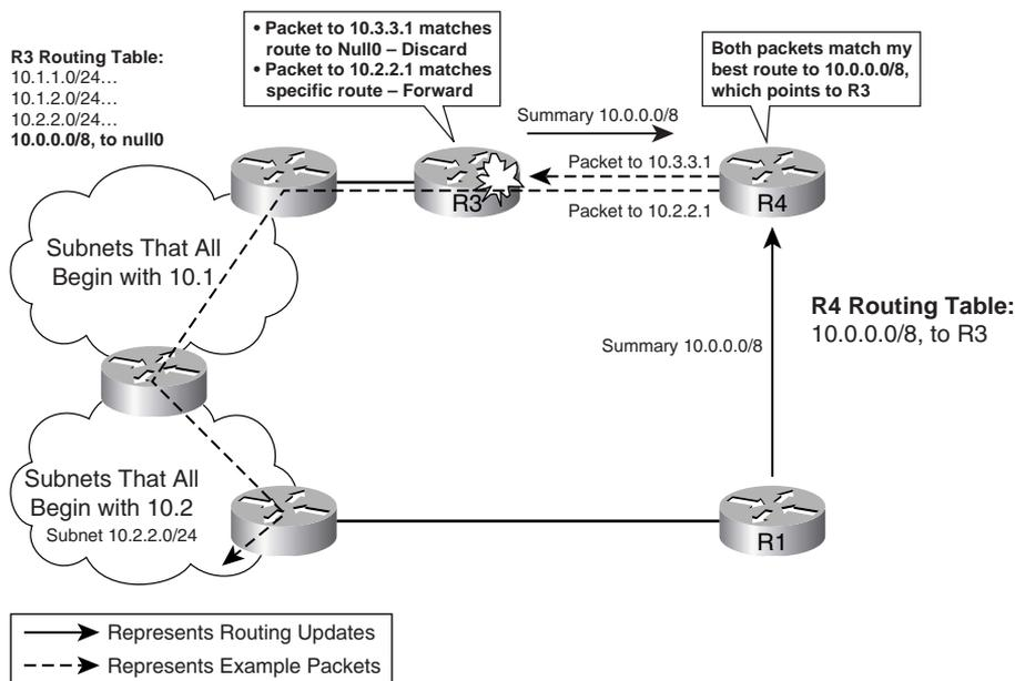
In Figure 11-7, R4 learned two paths to summary route 10.0.0.0/8, and picked the route through R3 based on the metric. Because R4 does not have a route for 10.2.2.0/24, R4 then sends any packets to that subnet based on its route to network 10.0.0.0/8, through R3. So, although subnets like 10.2.2.0/24 may be topologically closer to R4 through R1, R4 sends the packets via the scenic, suboptimal route through R3.
