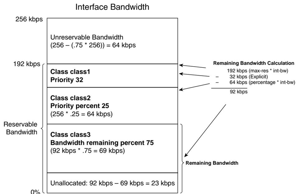
The most interesting part of Figure 15-8 is how IOS views the remaining-bandwidth concept when priority queues are configured. IOS subtracts the bandwidth reserved by the **priority** commands as well. As a result, a policy map can essentially allocate non-priority classes based on percentages of the leftover (remaining) bandwidth, with those values totaling 100 (100 percent).
