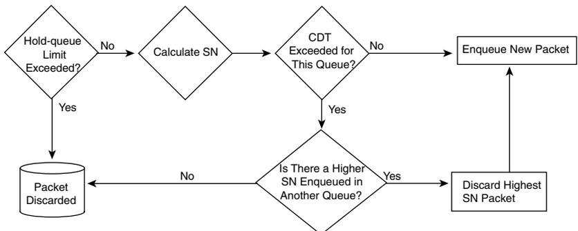
Note that each newly arriving packet goes through this process, but in one branch of the logic, the newly arrived packet is not discarded—another one is discarded. Essentially, if the new packet needs to go into a queue that has exceeded CDT, WFQ discards the highest-SN packet from any of the queues.
