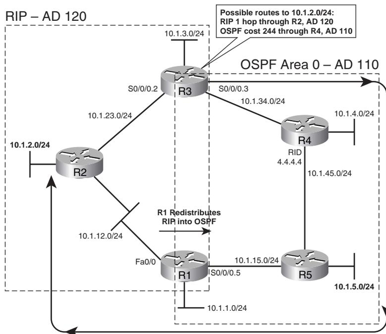
**NOTE** The OSPF configuration for this network matches only the interfaces implied by the OSPF box in Figure 11-4. RIP does not have a *wildcard-mask* option on the **network** command, so R1's and R3's **network** commands will match all of their interfaces, as all are in network 10.0.0.0.
