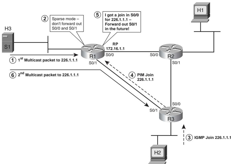
**NOTE** Throughout this chapter, the solid arrowed lines in the figures represent multicast packets, with dashed arrowed lines representing PIM and IGMP messages.
