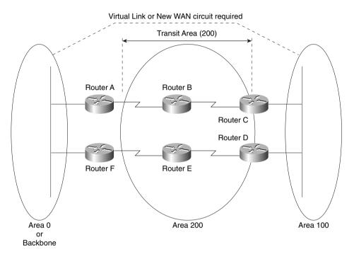
To ensure that Area 100 is reachable by the backbone, a virtual link can be configured over the transit area (200), and IP connectivity will be maintained. Virtual links are typically used in a transition phase (for example, when one company buys another and both companies use OSPF). Another solution to the problem depicted in Figure 2-16 is to install a physical link between Router C or Router D and the backbone core network.
