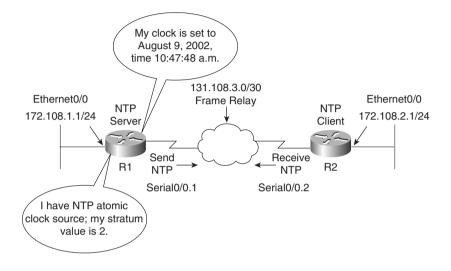
The following steps are required when enabling NTP on a Cisco router:
