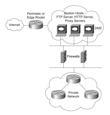
Figure 7-1 displays a typical perimeter network where the DMZ is separated by a firewall. *Firewalls* are network devices such as Private Internet Exchange (PIX), which are discussed later in this chapter. Firewalls are designed to protect the internal (or private) parts of a network from the public domain.
