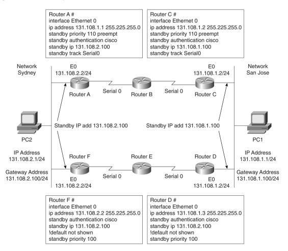
PCs are typically configured with only one gateway address. (Windows 2000/XP clients can take more than one but this still leaves a problem in that all devices must be configured for multiple gateways; the most scalable solution is to configure a single gateway on all devices and allow an intelligent network to provide redundancy where only a few devices require configuration.) Assume that PC1 is configured with a gateway address of 131.108.1.100. Two routers
