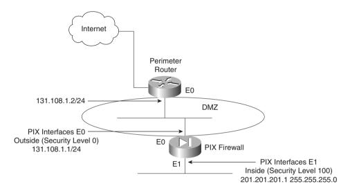
Figure 7-5 displays a typical DMZ and perimeter network between the inside (protected) and outside (public) networks.
