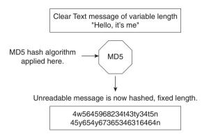
Figure 5-10 displays the simple clear text message, "Hello, it's me," which can be of any variable length. This message is sent to the MD5 process, where the clear text message is hashed and a fixed-length, unreadable message is produced. The data can include routing updates or username/password pairings, for example. MD5 produces a 128-bit hash output.
