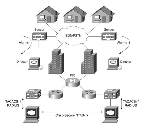
Figure 6-4 Typical NetRanger Design
