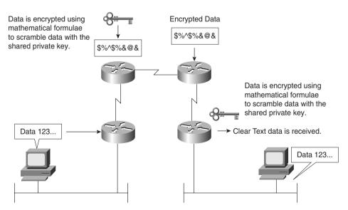
Figure 5-8 demonstrates the PC's clear text generation. The data is sent to the Cisco IOS router where it is encrypted with a shared key, sent over the IP network in unreadable format until the receiving router decrypts the message and forwards in clear text form.
