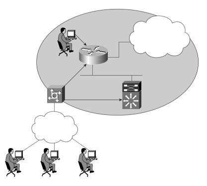
The users could be dialup users running Async (in this case PSTN) or using ISDN with Pointto-Point Protocol (PPP). The Network Access Server (NAS) ensures that only authenticated users have access to the secure network; it maintains resources and accounting information.
