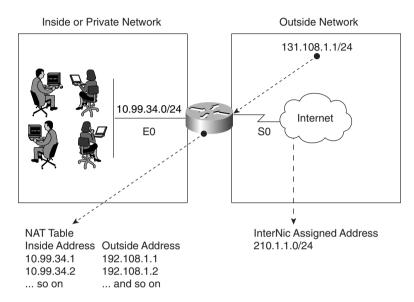
The users in Figure 7-2 are configured with the inside local addresses ranging from 10.99.34.1/24 to 10.99.34.254/24. To allow Internet access, NAT (PAT could also be configured if only one IP address was allocated by InterNIC) is configured on Router R1 to permit the inside local addresses access to the Internet. Advantages of using NAT include the following:
