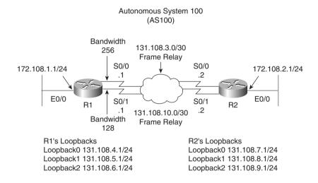
Routers R1 and R2 reside in AS 100, and to enable EIGRP on both routers, you need to start by configuring EIGRP. Example 2-15 displays the EIGRP configuration required on R1 and R2.
