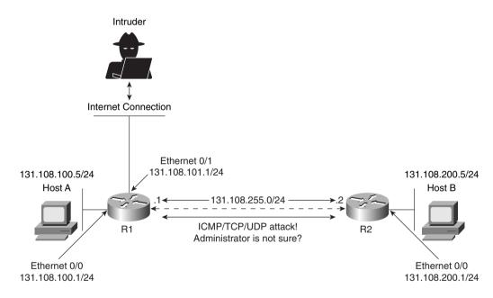
In this scenario, a Cisco IOS router is subjected to ICMP, TCP, or UDP IP packets. The network administrator is not sure of what type but notices the log file that is buffered to the Router R2 has just increased from 1 MB to 2.5 MB in less than 5 seconds. What can be done to characterize the traffic and detect the type of denial-of-service attack?
