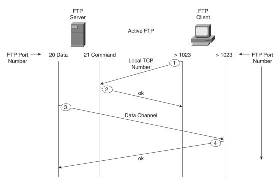
Figure 3-2 displays a typical FTP mode of operation between a client PC and FTP server in active mode. The following steps are completed before FTP data can be transferred:
