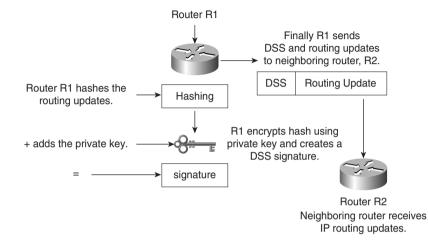
Routing updates are prone to network sniffers. By hashing the routing updates, as shown in Figure 5-9, the routing networks exchanged between Cisco IOS routers can be protected from unsecured devices.
