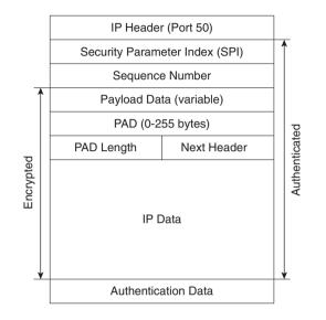
The Next Header is an 8-bit field that identifies the type of data contained in the Payload Data field. The IP data field contains the data to be sent. The Authentication Data field is a variable-length field containing an Integrity Check Value (ICV) computed over the ESP packet minus the Authentication Data.
