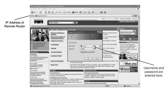
Figure 3-4 HTTP Authentication on a Cisco Router
