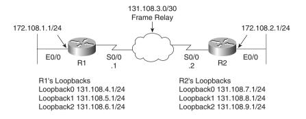
Example 2-10 displays the RIP configuration on R1. The same configuration commands are applied to R2.
