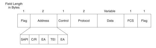
SAPI - Service Access Point Identifier C/R - Command/Response EA - Extended Address TEI - Terminal Endpoint Identifier (All 1s indicate a broadcast.)
