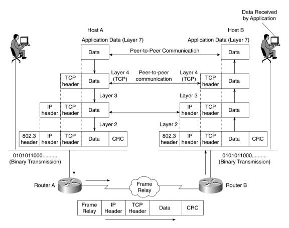
The data from one (Host A) is encapsulated inside a TCP header and passed down to Layer 3 (the IP layer) for address configuration, where an IP header is also added. Information included here is the source IP address and destination address. Layer 3 (the network layer) passes the data to the local router acting as the gateway via the Ethernet connection in raw binary.
