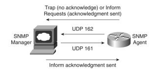
Figure 3-6 Communication Between SNMP Manager and SNMP Agent
