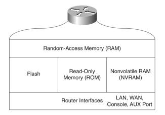
Each hardware component is vital for Cisco routers to operate properly. To help you prepare for the CCIE Security written exam, the next few sections present the main concepts you need to know about Cisco hardware components.
