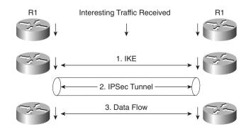
In Figure 5-19, interesting traffic (or traffic from an end user, for example) triggers the IKE phases I/II followed by the establishment of the IPSec tunnel. After the IPSec tunnel is established, the data can be transferred. After the data is transferred, the IPSec tunnel is closed. You can tunnel any form of data across the IPSec tunnel, such as IP, Novel IPX, or AppleTalk.
