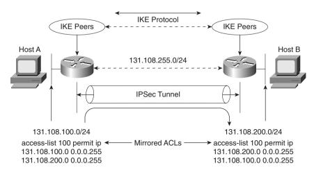
To start, configure IKE on Router R1. Example 5-15 displays the IKE configuration on R1. Remember that IKE policies define a set of parameters to be used during IKE negotiation.
