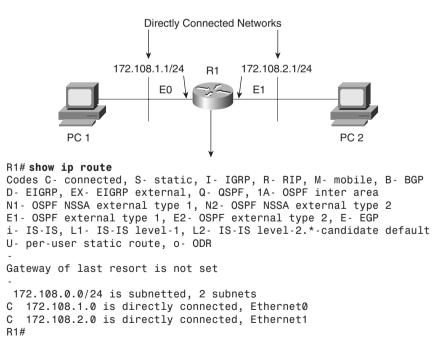
PC1 can communicate with PC2 as shown in Figure 2-13, because Cisco routers will route to directly connected interfaces.
