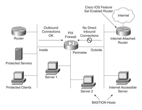
Although optional, it is recommended that you install the Cisco IOS Firewall software on the router directly connected to the Internet. The Cisco IOS Firewall feature is discussed later in this chapter.
