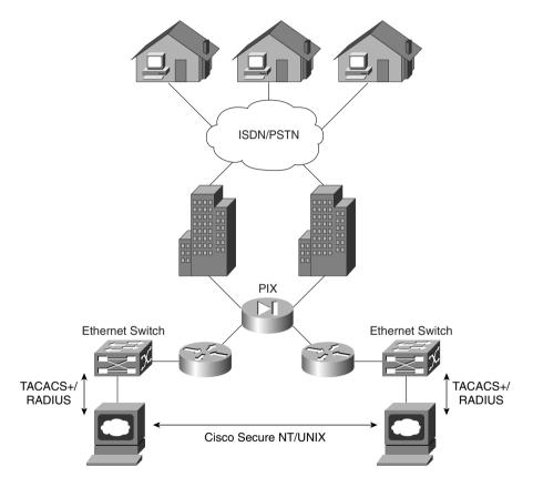
Figure 6-3 displays a typical application where ISDN/PSTN users are authenticated by RADIUS or TACACS+ via the Cisco Secure ACS server.
