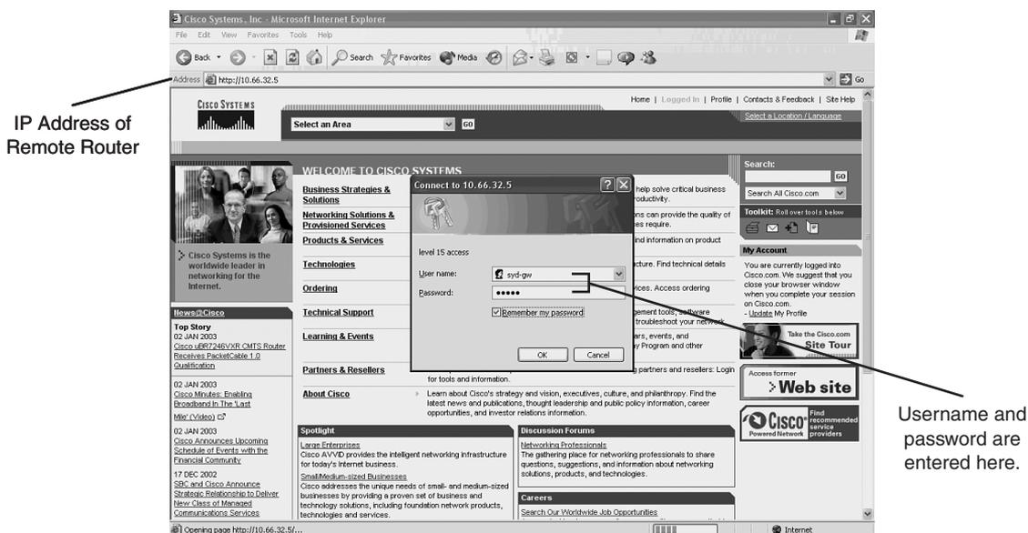
After the user is authenticated, the user enters the remote IP address or DNS name.
