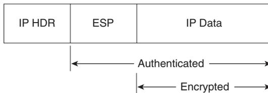
ESP does not encrypt the original IP header, and encrypts only the IP data by placing a header in between the original IP header and data. ESP provides data confidentiality, data integrity, and data origin authentication. ESP also prevents replay attacks. Replay attacks can include intruders capturing a valid packet and replaying it over the network in an attempt to get a packet conversation between an illegal and legal host.
