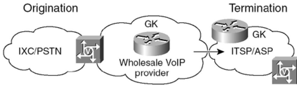
Figure 6-7. Topology 2: originating TDM/terminating IP.
