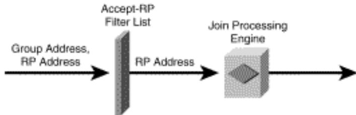
Router A has just received a (\*, G) Join from a downstream PIM neighbor. However, before processing the message, the group address G and the RP address (both of which are contained in the body of the (\*, G) Join message) are run through the **ip pim accept-rp** filter. If the filter permits this Group/RP combination, then the incoming (\*, G) Join message is processed; otherwise, it is ignored.
