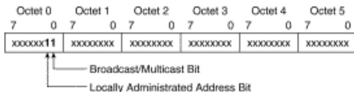
If this bit is set, then the MAC frame is destined for either an arbitrary group of hosts or all hosts on the network (if the MAC destination address is the broadcast address, 0xFFFF.FFFF.FFFF). IP multicasting at Layer 2 makes use of this capability to transmit IP multicast packets to a group of hosts on a LAN segment.
