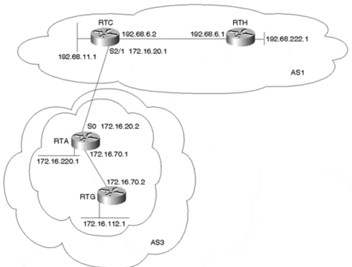
RTC has noticed lots of fluctuations in network 172.16.220.0/24 coming from AS3, causing oscillation in its BGP and consequently in OSPF. The 172.16.220.0/24 keeps showing up and disappearing from RTH's routing table. To rectify the problem, RTC will apply dampening to the BGP by using a route map to selectively dampen route 172.16.220.0/24 only. [Example 12-88](#) and [Example 12-89](#) show the configurations for RTG and RTA, respectively.
