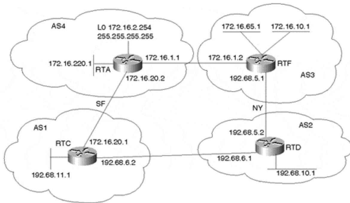
Examples 12-32 through 12-34 show the relevant configuration of RTA, RTC, and RTF, respectively. RTD should be a mirror image of RTC.
