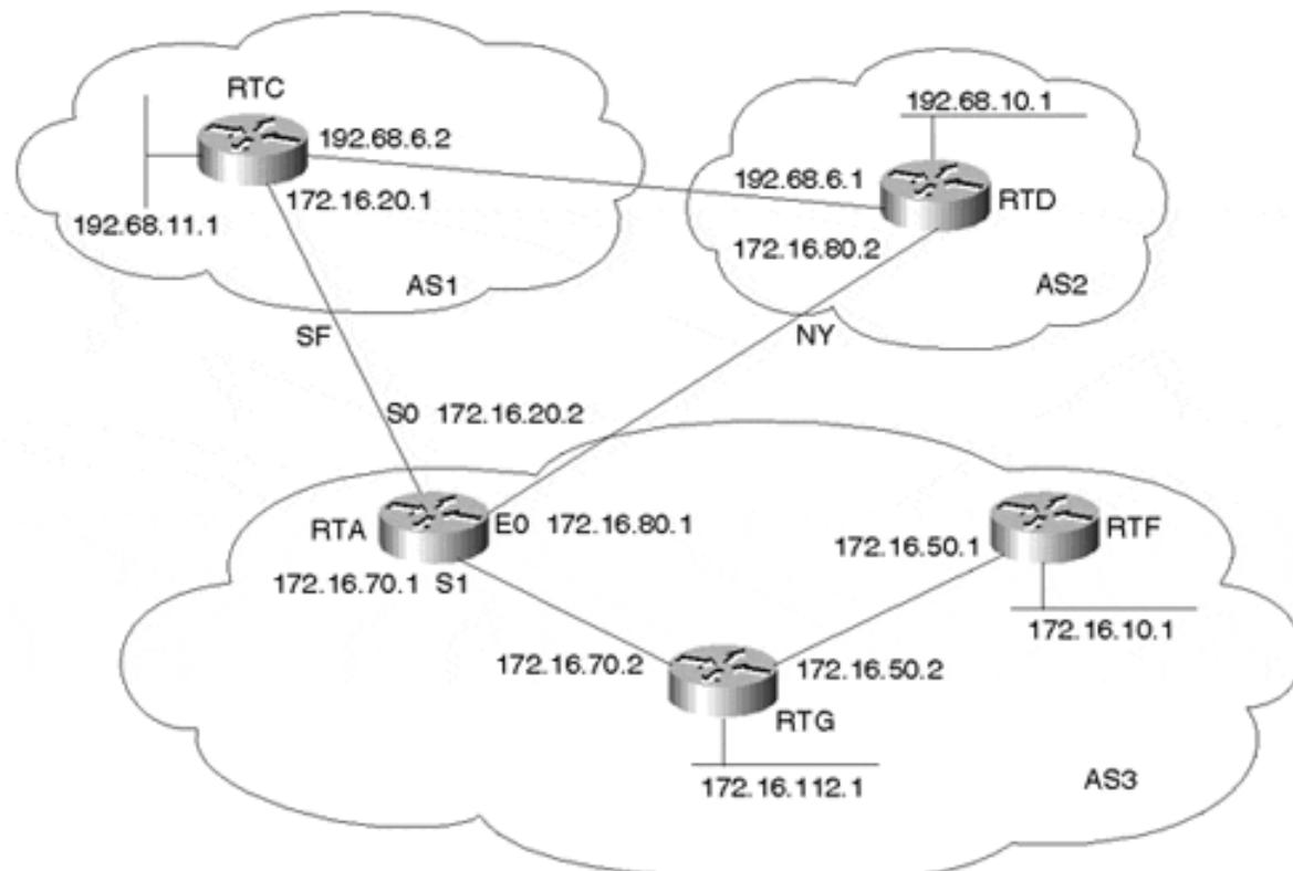
RTA wants to set policy routing in such a way that traffic coming over the serial line S1 from RTG is directed toward AS2 if the source is network 172.16.10.0/24. Traffic coming from RTG with source 172.16.112.0/24 is to be directed toward AS1; in case of a link failure to AS1, the traffic will go to AS2. For all other source IP addresses, follow normal routing.
