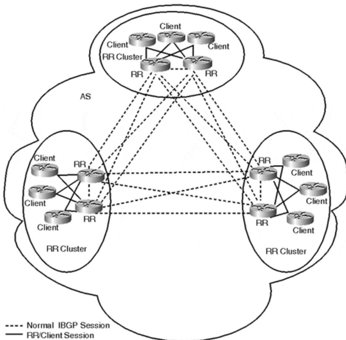
**Figure 9-8. Full-Mesh BGP Topology**
