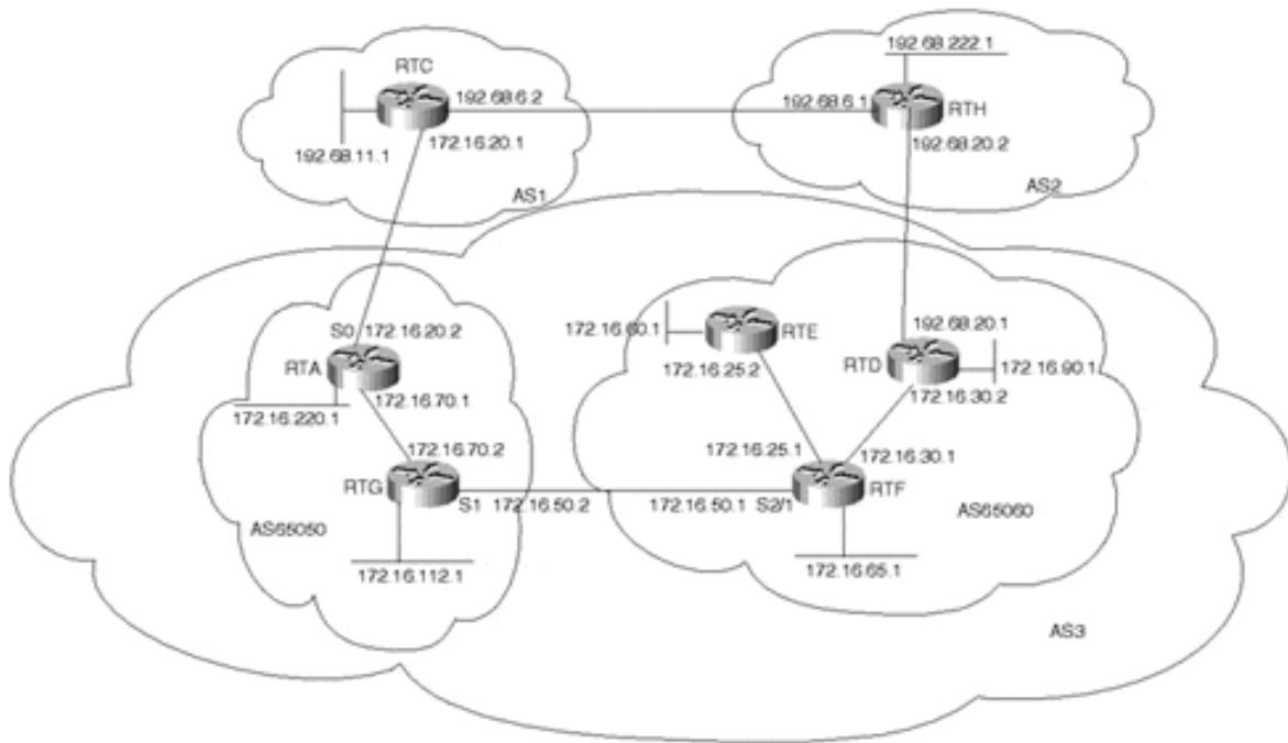
The configuration for RTA in [Example 12-73](#) shows that RTA has all its interfaces in OSPF area 5. RTA is running EBGP with RTC in AS1 and is running IBGP with RTG in AS65050. Note that RTA uses the **bgp confederation identifier 3** router subcommand to present itself to RTC as being part of confederation 3.
