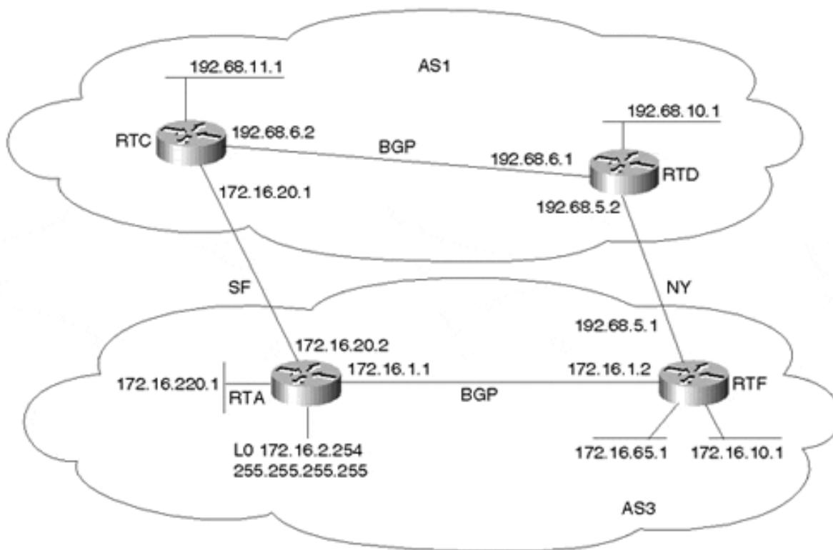
RTA will send over its direct link to AS1 the aggregate 172.16.0.0/16 plus the more-specific routes 172.16.1.0/24, 172.16.10.0/24, and 172.16.65.0/26. RTF will send over its direct link to AS3 the aggregate 172.16.0.0/16 plus the more-specific route 172.16.220.0/24 only. As a result, AS1 is forced to reach 172.16.220.0/24 via RTF and all the other routes in AS3 via RTA.
