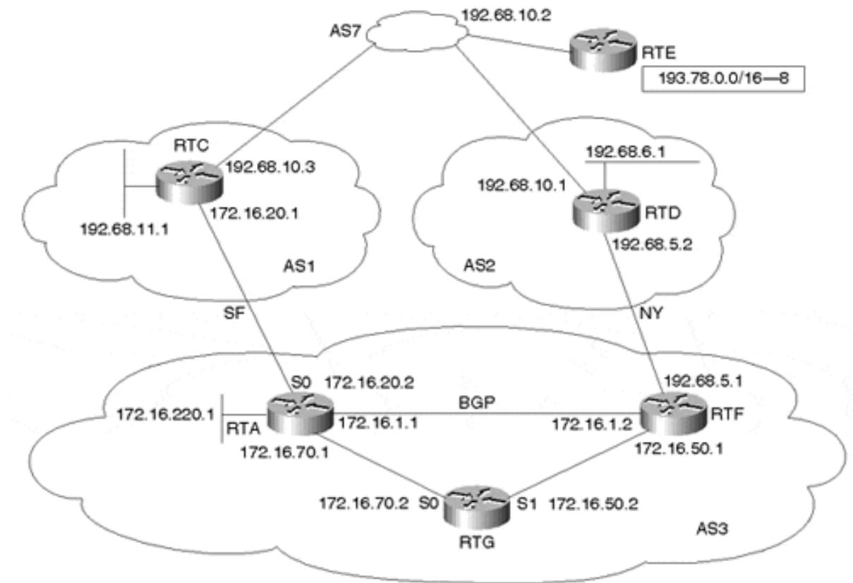
The scenario in which RTA and RTF are directly connected is easy; it is very hard for things to go wrong. As long as RTA and RTF are injecting defaults inside the IGP, traffic that reaches any of the BGP routers will find its way outside the AS. It is important that outbound traffic that reaches a BGP router does not go back to the non-BGP routers to avoid possible routing loops.
