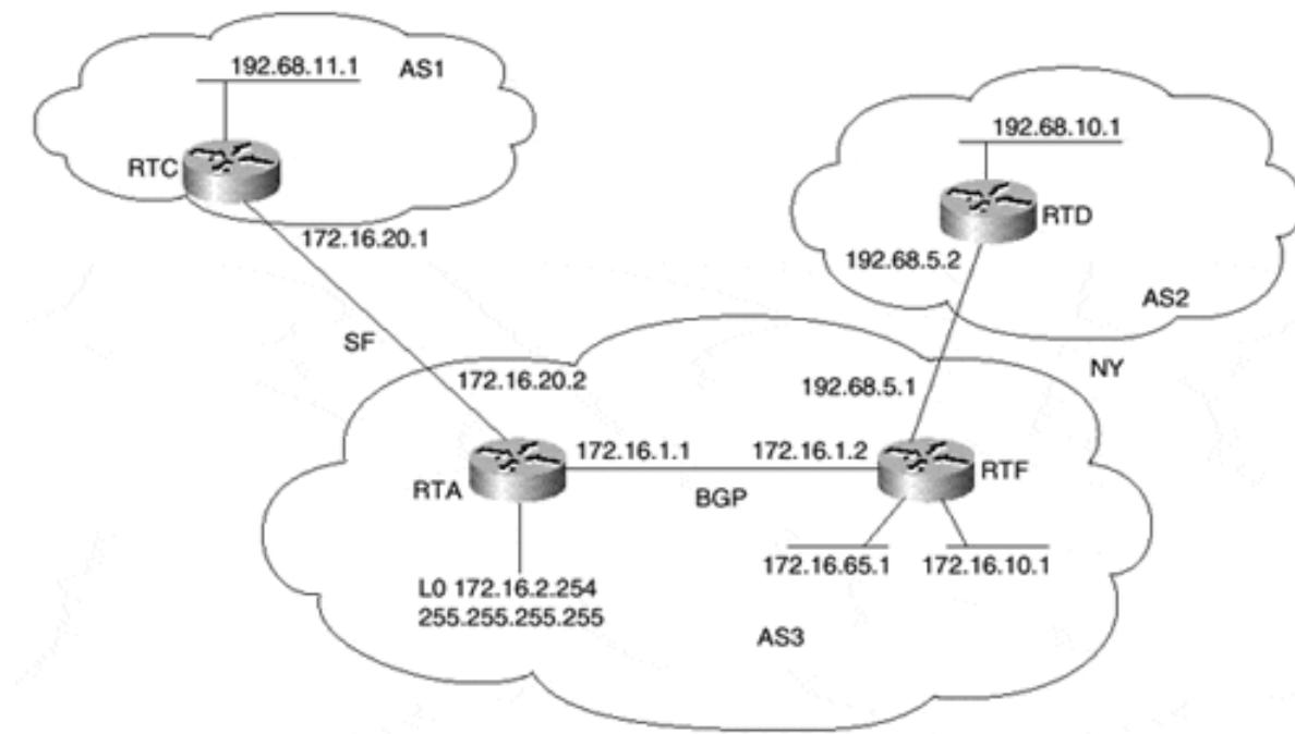
In Figure 11-14, RTA and RTF are getting routes 192.68.11.0/24 and 192.68.10.0/24 from ASes 1 and 2, respectively. If RTA and RTF are to aggregate these routes into 192.68.0.0/16 using the **as-set** option, the aggregate cannot be sent back to either AS1 or AS2, because it contains {1 2} in the AS path. This is due to the normal BGP behavior in detecting loops.
