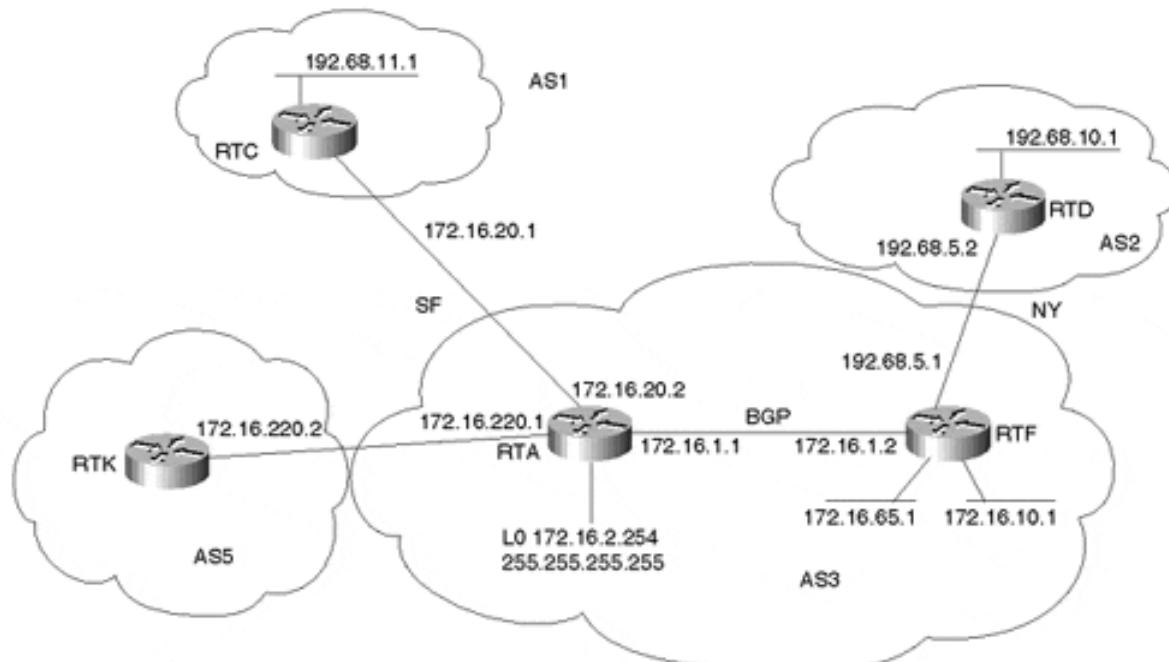
In [Figure 11-13](#), RTA is aggregating prefixes 192.68.10.0/24 and 192.68.11.0/24 coming from AS2 and AS1, respectively. Without AS\_SET, the aggregate 192.68.0.0/16 will be
