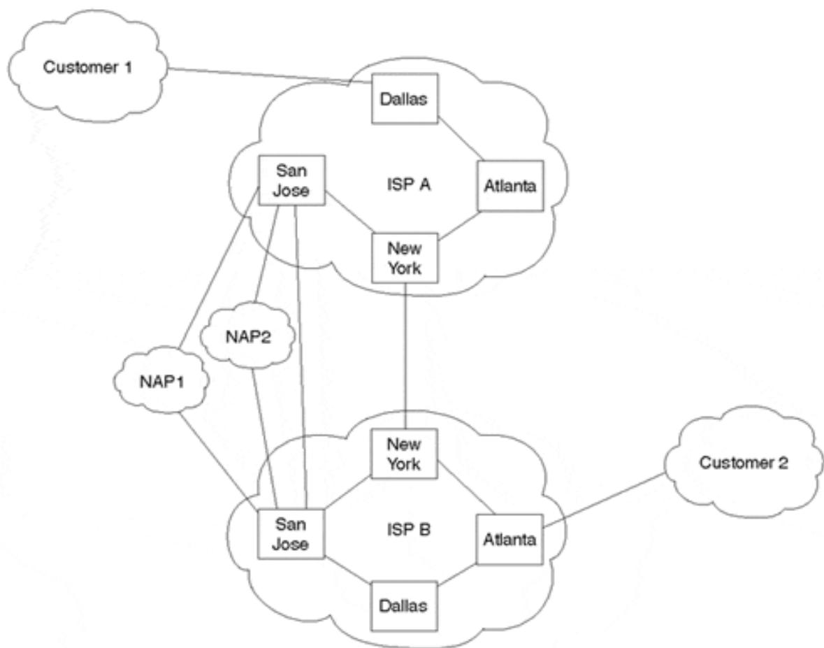
**Figure 2-7. Redundant Interconnection Model**
