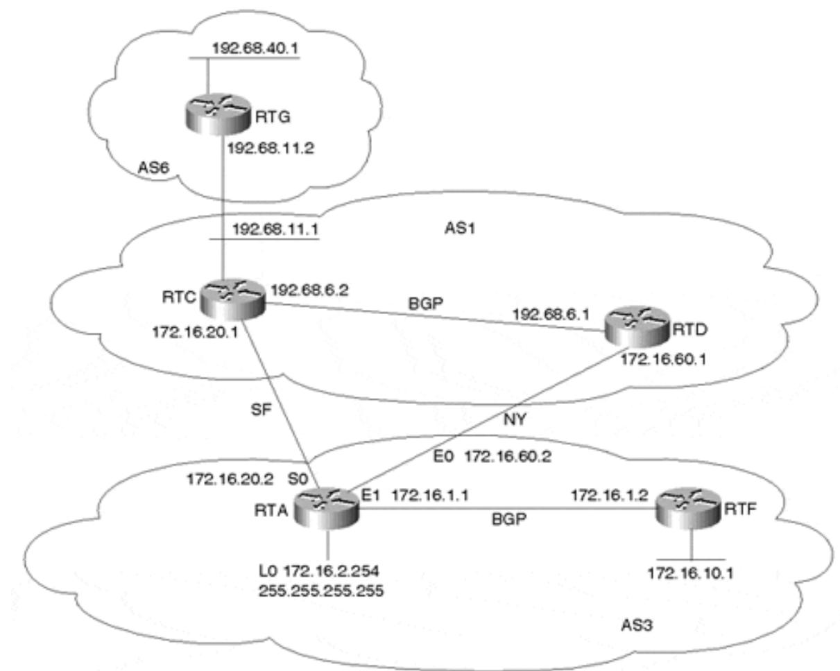
RTA is EBGP peering with routers RTC and RTD in AS1. RTA is receiving identical updates about prefixes 192.68.11.0/24 and 192.68.40.0/24 from two links. You can configure RTA with the **maximum-paths** BGP router subcommand to enable IP routing to load balance among up to six paths. In [Example 12-18](#), the **maximum-paths** number is set to 2.
