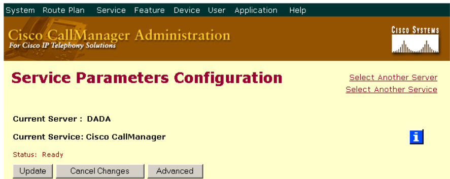
Figure 30-1 Service Parameter Configuration Pane
