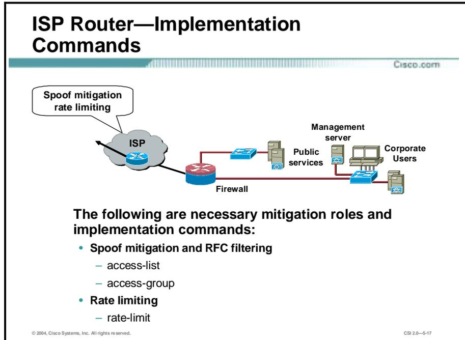
The primary function of the customer-edge router in the ISP is to provide connectivity to the Internet or ISP network. The egress of the ISP router rate-limits nonessential traffic that exceeds pre-specified thresholds in order to mitigate distributed denial of service (DDoS) attacks. At the egress of the ISP router, RFC 1918 and RFC 2827 filtering is configured to mitigate source-address spoofing of local networks and private address ranges.
