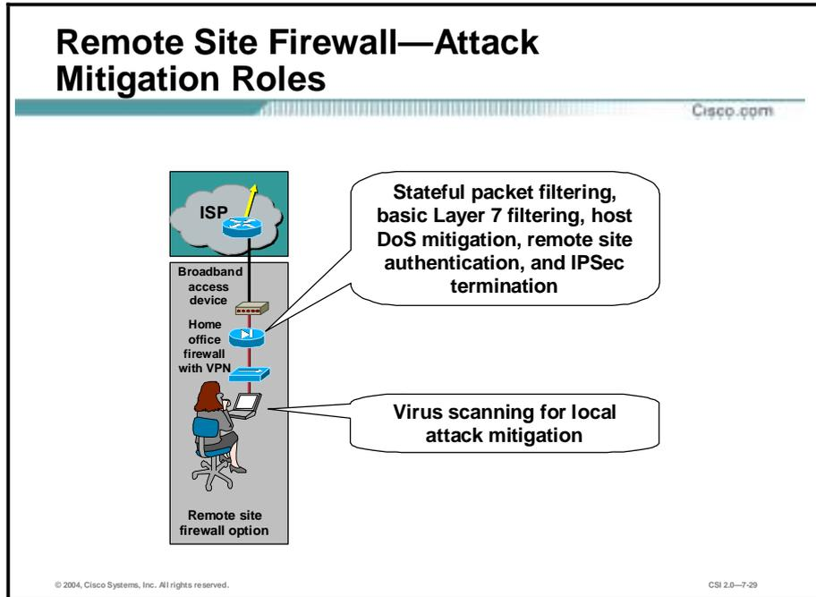
This figure provides attack mitigation roles for the remote site firewall option:
