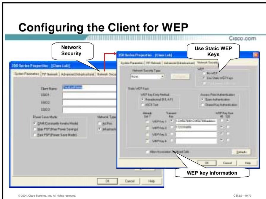
Static WEP keys are set on the client using the ACU. From the Aironet Client Utility screen, click **Profile Manager**. This will launch the Profile Manager screen. From the Profile Manager, choose the desired profile from the drop down box and click the **Edit** button.
