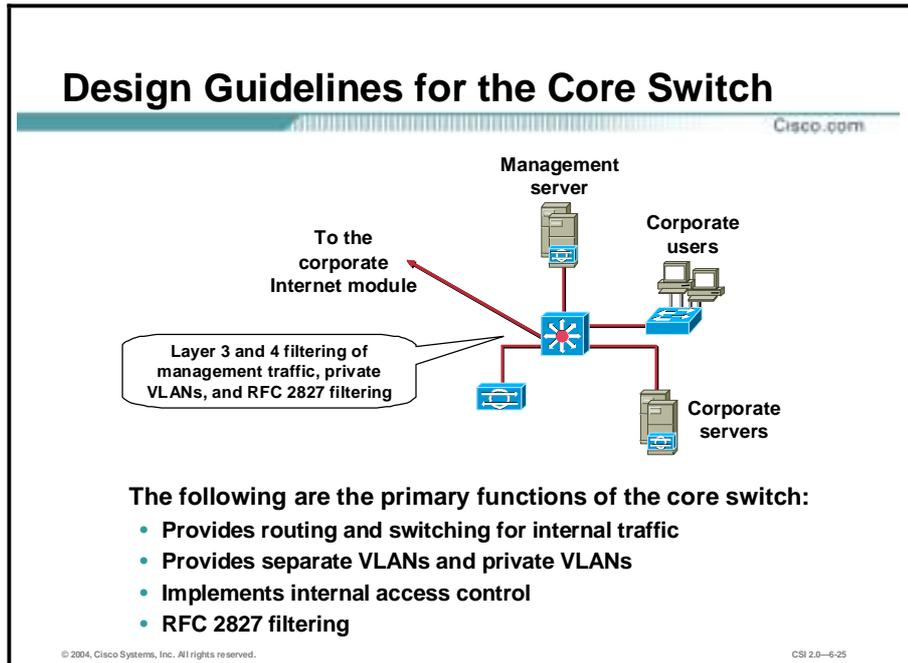
The primary function of the core switch is to provide routing and switching for production and management traffic, distribution layer services (routing, quality of service [QoS], and access control) for the distribution and access switches, connectivity for the corporate and management servers, and advanced services such as traffic filtering between the subnets.
