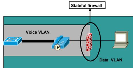
**For PC-based IP phones, SAFE recommends deploying a stateful firewall to broker data-voice interaction.**
