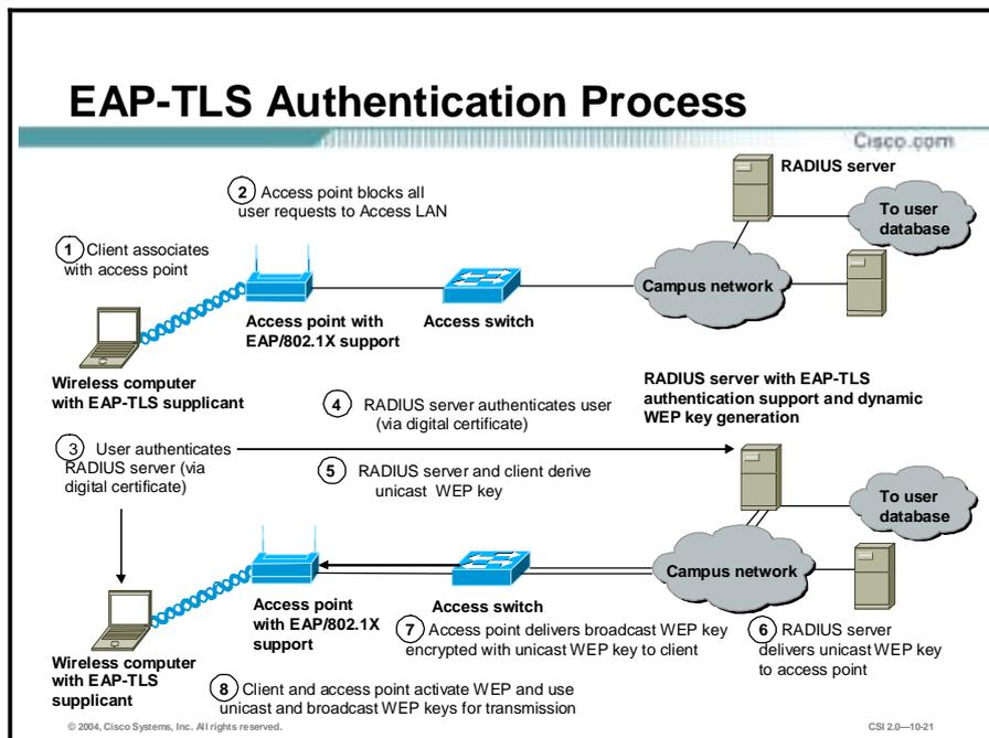
EAP-TLS is an Internet Engineering Task Force (IETF) standard (RFC 2716) that is based on the TLS protocol (RFC 2246). EAP-TLS uses digital certificates for both user and server authentication and supports the three key elements of 802.1x/EAP mentioned previously.
