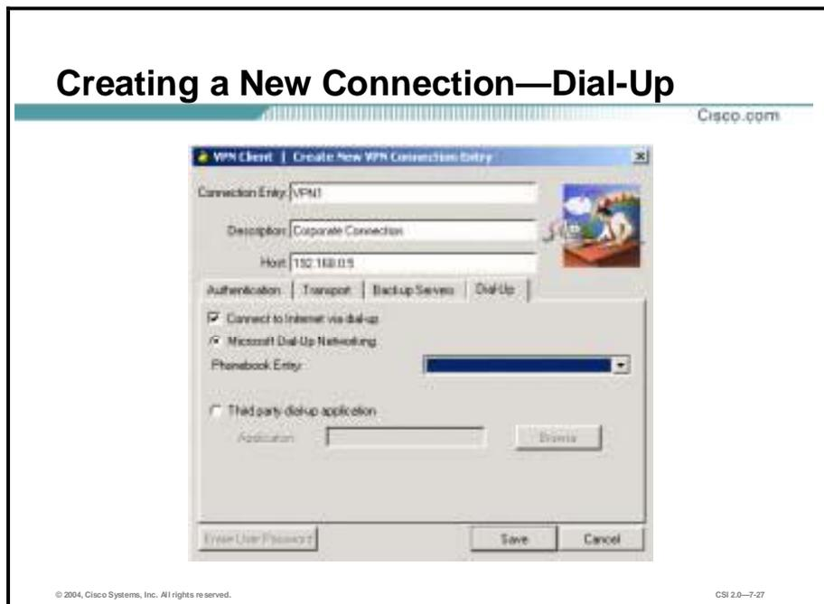
To enable and configure a connection to the Internet through dial-up networking, select the **Connect to Internet via dial-up** check box. This feature is not selected by default.
