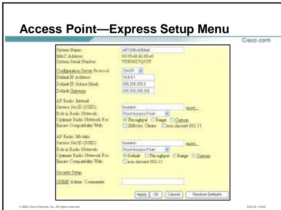
The first time the access point is turned on, this is the default web page for the access point. It will remain the default page until a configuration is successfully applied or you click **OK**. The Express Setup page contains the following settings:
