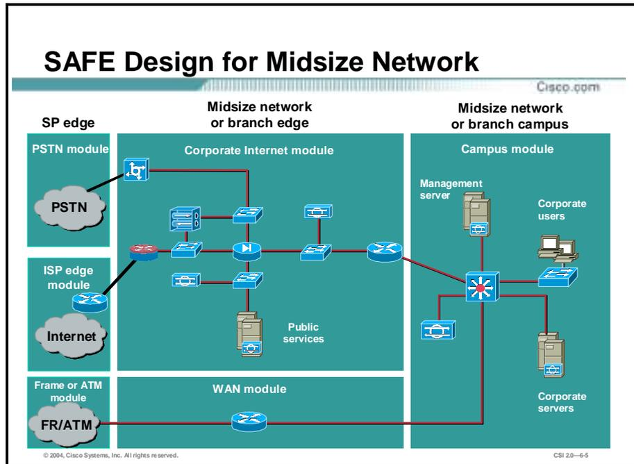
As in the small network design, the corporate Internet module has the connection to the Internet, and terminates VPN traffic and public-services traffic (Domain Name System [DNS], HTTP, FTP, and Simple Mail Transfer Protocol [SMTP]). Dial-in traffic also terminates at the corporate Internet module. The campus module contains the Layer 2 and Layer 3 switching infrastructure along with all the corporate users, management servers, and intranet servers.
