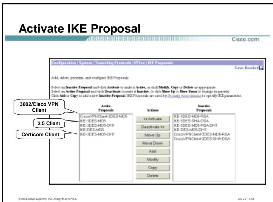
The VPN 3000 Concentrator can handle three types of remote clients: Cisco VPN client, Altiga client, and Certicom client. Before the VPN 3000 Concentrator can interface with these clients, you must make sure that the appropriate IKE proposal is configured, activated, and prioritized.
