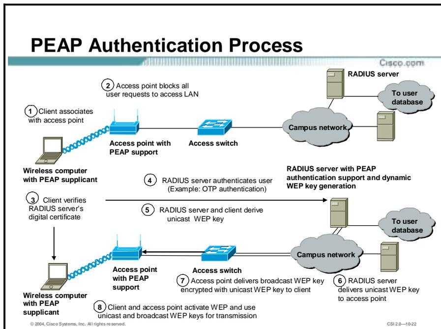
PEAP is an IETF draft RFC authored by Cisco Systems, Microsoft, and RSA Security. PEAP uses a digital certificate for server authentication. For user authentication, PEAP supports various EAP-encapsulated methods within a protected TLS tunnel. PEAP supports the three main elements of 802.1x/EAP, as mentioned previously.
