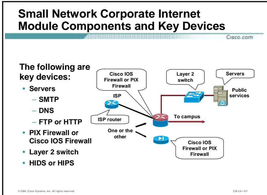
The corporate Internet module provides internal users with connectivity to Internet services and Internet users access to information on public servers. VPN access is also provided to remote locations and telecommuters. This module is not designed to serve e-commerce type applications.
