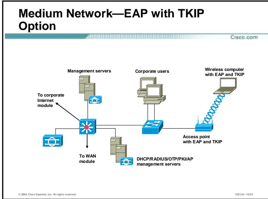
The medium network WLAN overlays wireless on top of the campus portion of the SAFE medium network design. All the components for implementing the mitigation techniques are contained within the medium-campus module. These components are intended to allow WLAN access for end users within the medium-network campus.
