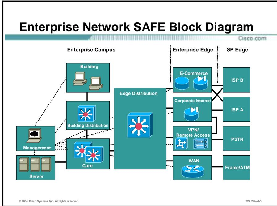
The enterprise comprises two functional areas: the Enterprise Network Campus and the Enterprise Network Edge. These two areas are further divided into modules that define the various functions of each area in detail.
