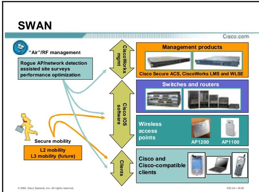
The Cisco Structured Wireless-Aware Network (SWAN) combines the Cisco switch and router infrastructure with the Cisco wireless network, making one integrated "wireless-aware" network. This secure, integrated wired and wireless network extends Cisco's proven LAN infrastructure capabilities to the WLAN, providing the security, management, ease-of-deployment, scalability, and reliability that our enterprise customers depend on for their core business applications.
