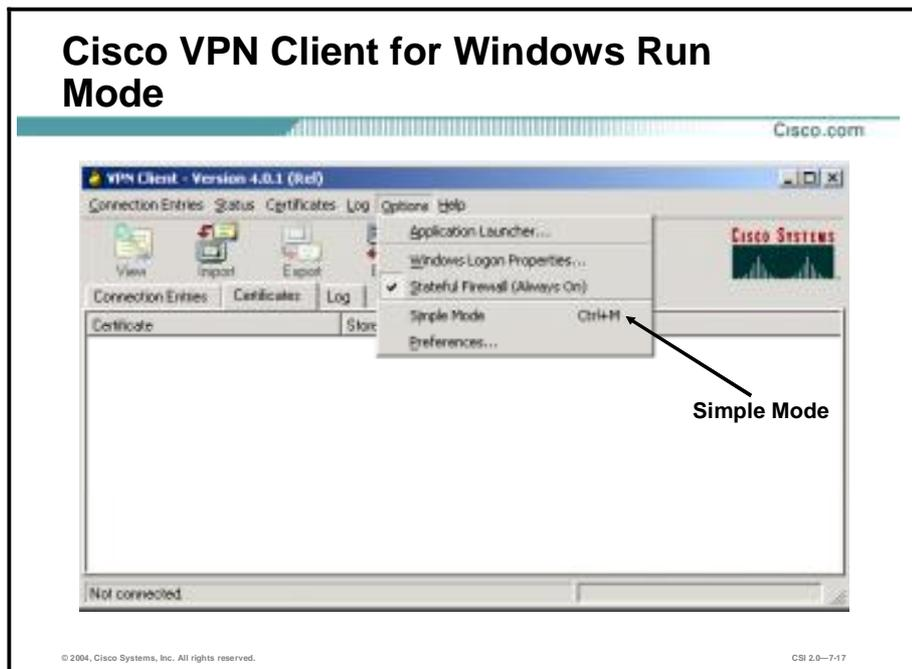
You can run the Software Client in simple mode or in advanced mode. The default is advanced mode, although your network administrator might have configured simple mode as the default.
