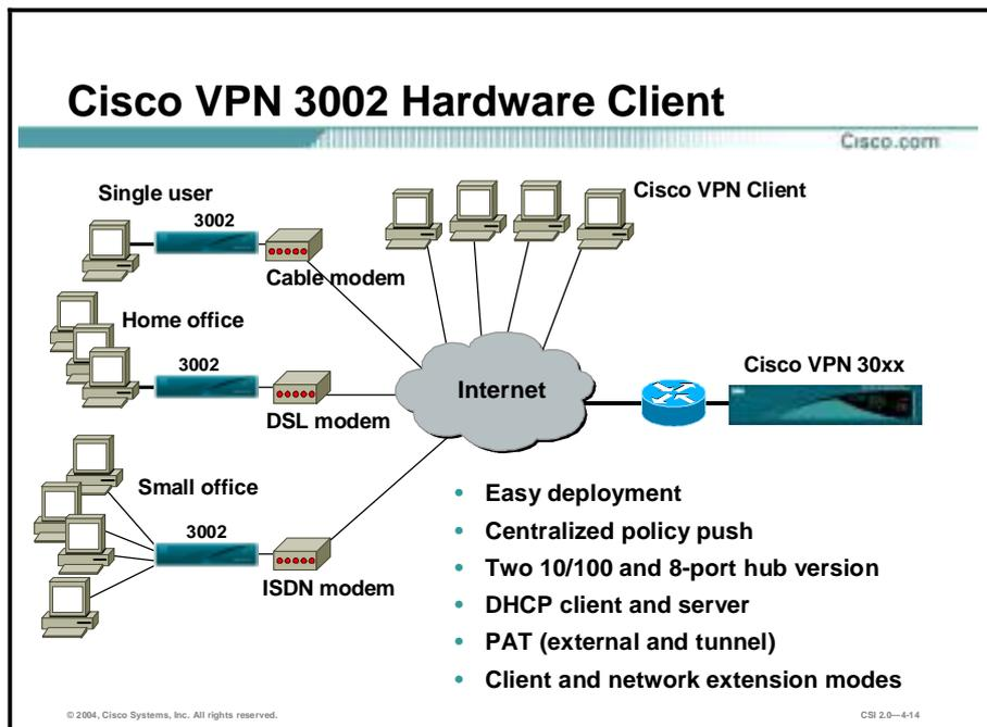
Based on the unified VPN Client framework, the Cisco VPN 3002 Hardware Client combines the best features of a software client, including scalability and ease-of-deployment, with the stability and independence of a hardware platform. The Cisco VPN 3002 Hardware Client works with all operating systems and does not interfere with the operation of the PC because it is a separate hardware appliance.
