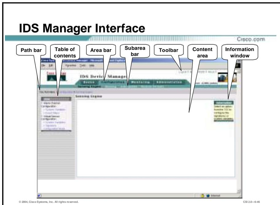
The IDM GUI provides the network security administrator with an intuitive approach to configuring Sensors. The GUI has the following sections:
