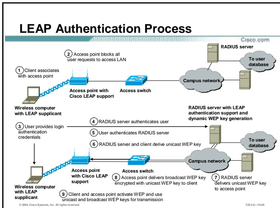
Cisco LEAP is the widely deployed EAP type in use today in WLANs. LEAP supports all three of the 802.1x and EAP elements mentioned previously. With LEAP, mutual authentication relies on a shared secret, the user's logon password, which is known by the client and the network.
