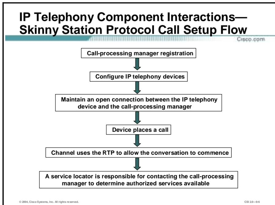
These IP telephony component interactions model that of the Skinny Station Protocol and are provided as a reference call setup flow:
