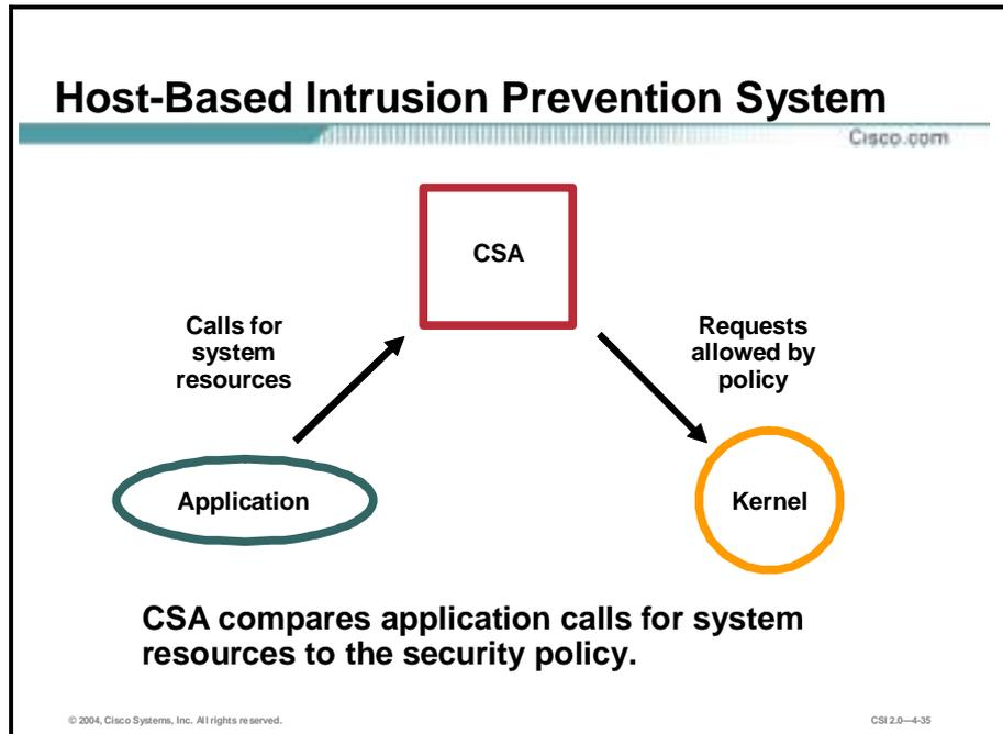
CSA is a HIPS that provides a third layer of depth to the network defense by applying security policy to system behavior at the host level. With this different approach to security, CSA can stop attacks missed at other levels of network security for the following reasons:
