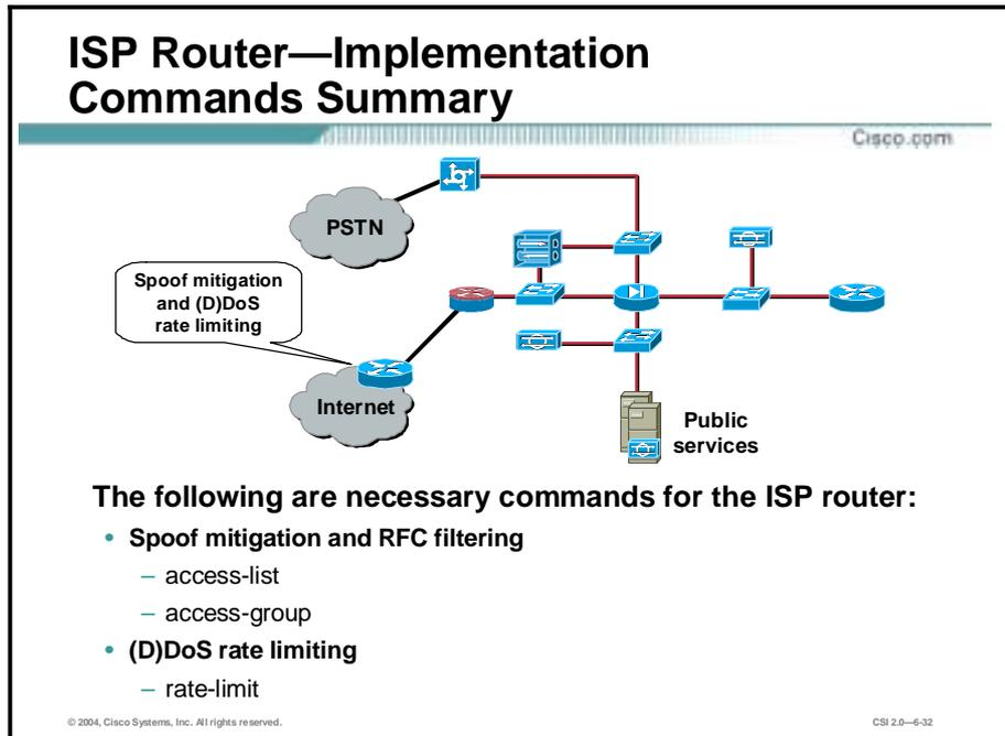
Starting at the customer edge router in the ISP, the egress of the ISP rate limits nonessential traffic that exceeds pre-specified thresholds in order to mitigate DDoS attacks. Also at the egress of the ISP router, RFC 1918 and RFC 2827 filtering mitigates source-address spoofing of local networks and private address ranges.
