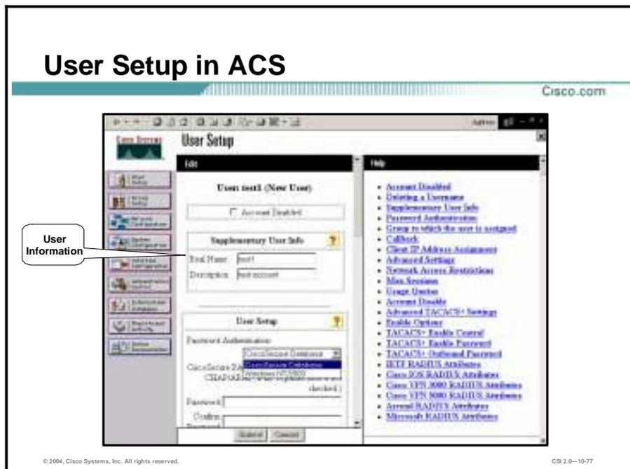
To configure accounts on Cisco ACS, click the **User Setup** button from the main screen. This will launch the User Setup screen. Enter information about the user.
