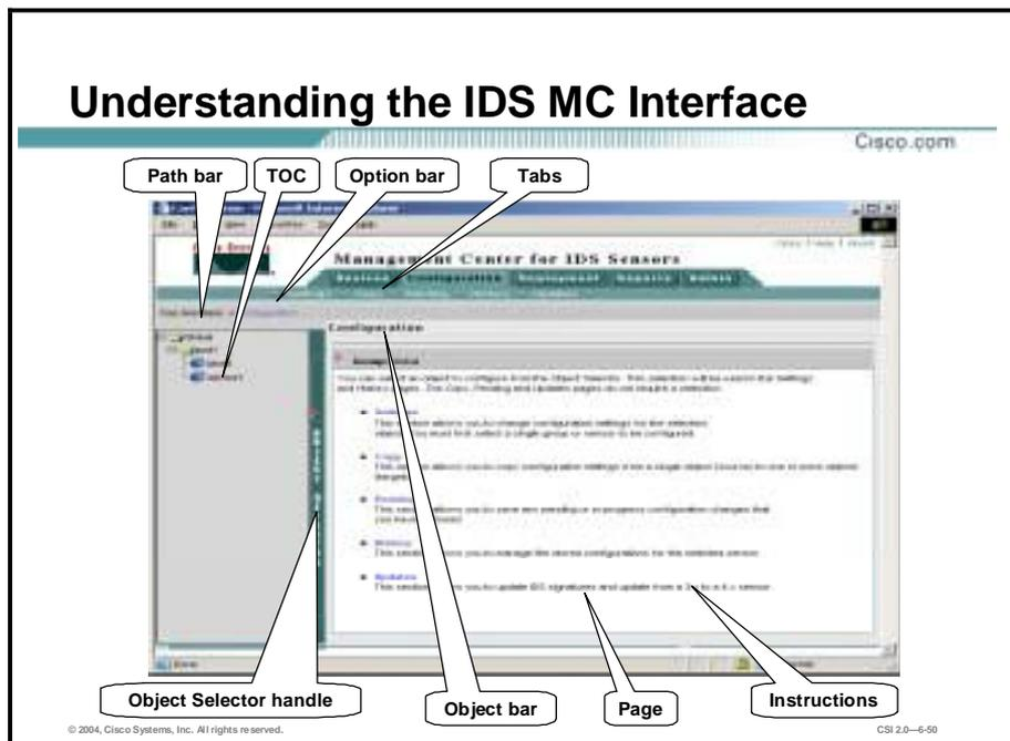
The figure illustrates elements of the IDS MC GUI. The elements are described as follows:
