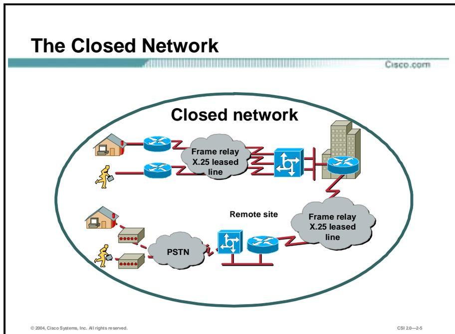
The closed network typically consists of a network designed and implemented in a corporate environment, and it provides connectivity only to known parties and sites without connecting to public networks. Networks were designed this way in the past and thought to be reasonably secure because there was no outside connectivity.
