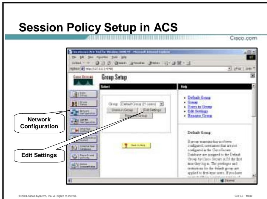
To adjust the timeout value for the client session (requiring re-authentication and new WEP key derivation as in LEAP), click the **Group Setup** button from the ACS main screen. This will launch the Group Setup screen.
