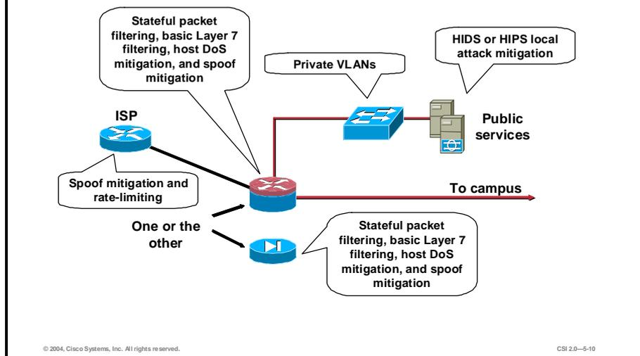
The attack mitigation roles for each device in the SAFE SMR small network corporate Internet module are as follows:
