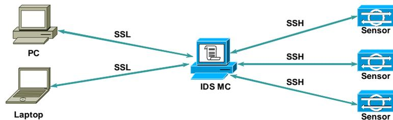
**The IDS MC is a web-based application that centralizes and accelerates the deployment and management of multiple IDS Sensors or IDS Ms.**
