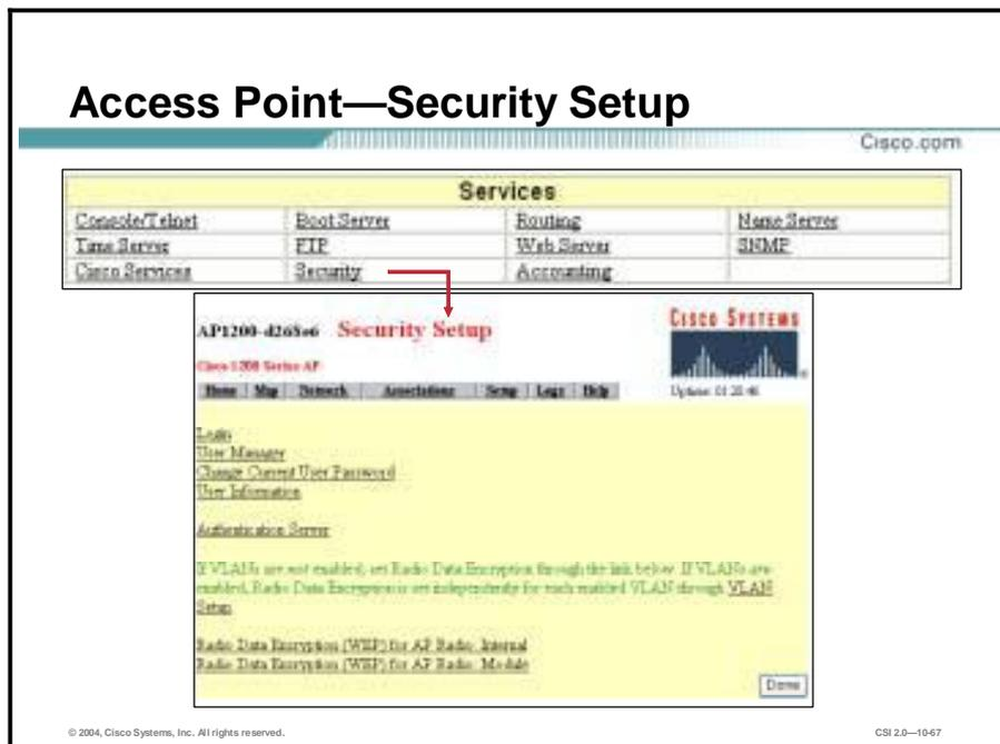
The Services menu has the option to configure access point security. The security features protect wireless communication between the access point and other wireless devices, control access to your network, and prevent unauthorized entry to the access point management system. In order to maximize security on the WLAN, a number of features need to be enabled and configured. These features are as follows:
