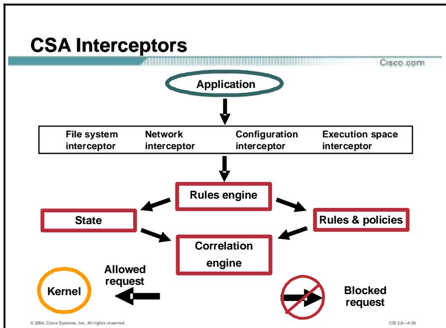
When an application needs access to system resources, it makes an operating system call to the kernel. CSA intercepts these operating system calls and compares them to the cached security policy. If the request does not violate policy, it is passed to the kernel for execution.
