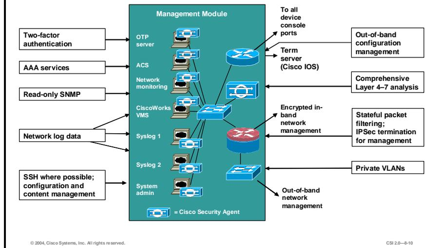
The attack mitigation roles for each device in the SAFE Enterprise Network Campus Management module are as follows:
