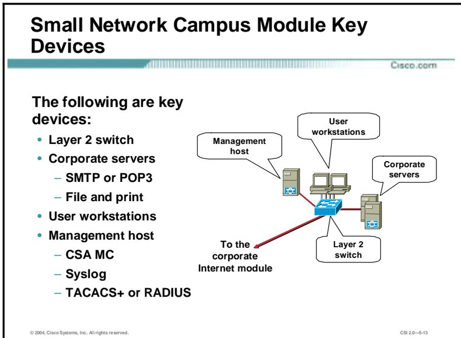
The campus module contains end-user workstations, corporate intranet servers, management servers, and the associated Layer 2 infrastructure required to support the devices. Within the small network design, this Layer 2 functionality has been combined into a single switch.
