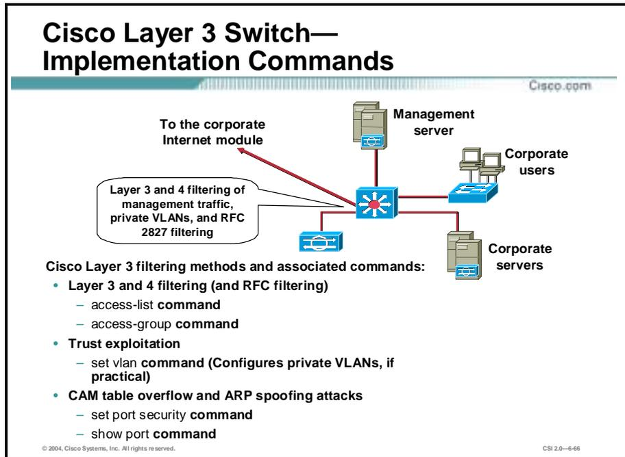
The following commands and features are used to implement SAFE SMR on a Layer 3 switch:
