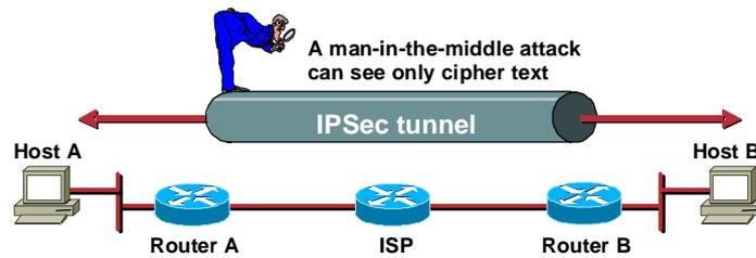
**Man-in-the-middle attacks can be effectively mitigated only through the use of cryptography (encryption).**
