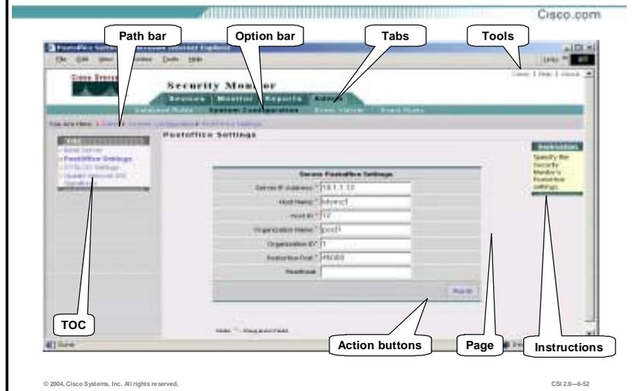
The figure illustrates elements of the Security Monitor GUI. The elements are described as follows:
