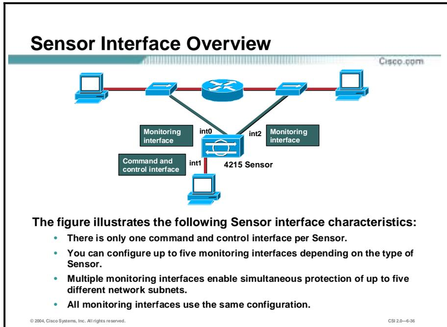
Each Sensor has only one command and control interface, but you can configure up to five monitoring interfaces depending on the type of Sensor you have. Multiple interfaces enable simultaneous protection of up to five different network subnets, which is like having five Sensors in a single appliance.
