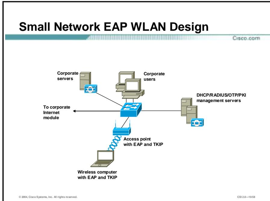
The small WLAN network design overlays WLAN on top of the SAFE small network design. The small WLAN design is contained within the campus module. This topic discusses one option, EAP with TKIP, for providing WLAN users connectivity to the wired campus. IPSec is not presented as an option because of the financial burden of implementing a dedicated WLAN VPN in a network of this size.
