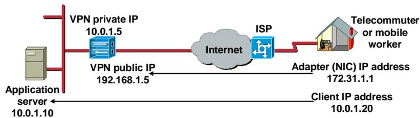
**The result of implementing IPSec remote-user-to-LAN tunneling is that the security perimeter of your organization is extended to include remote sites.**
