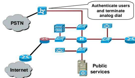
**Traditional dial-in users are terminated on an access router with built-in modems. CHAP is used to authenticate the user along with the AAA server.**
