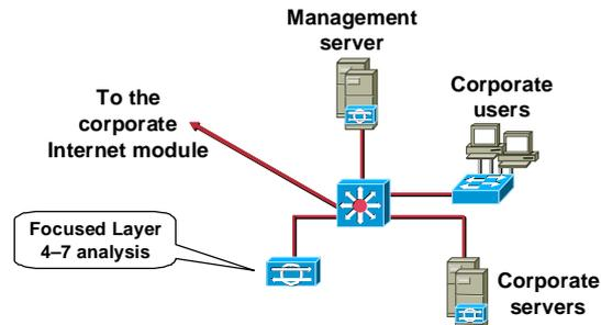
**Intrusion detection should monitor internal traffic for suspicious activity. Very few attacks should be detected.**
