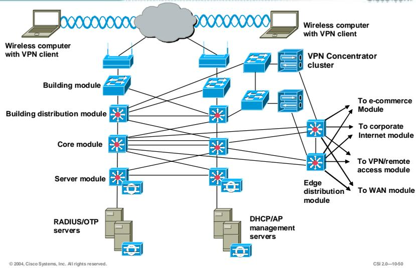
IPsec VPN access via the wireless network uses several modules from the SAFE enterprise architecture, as follows:
