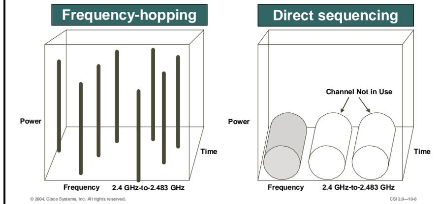
The 802.11 standard specifies two different types of Layer 1 physical interfaces for radio-based devices. One uses a frequency-hopping architecture, whereas the other uses a more straightforward single-frequency approach, known as direct sequencing.
