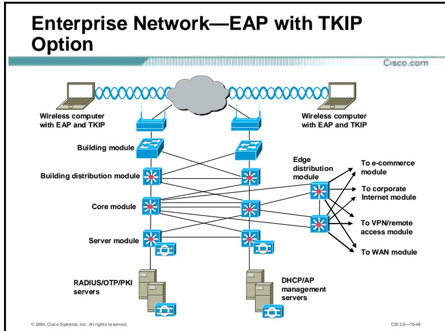
The large-enterprise WLAN network design overlays WLANs on top of the campus portion of the SAFE enterprise blueprint. All of the components for implementing the mitigation techniques are contained within the large-enterprise building, distribution, and server modules. These components are intended to allow WLAN access for enterprise end users within the enterprise campus.
