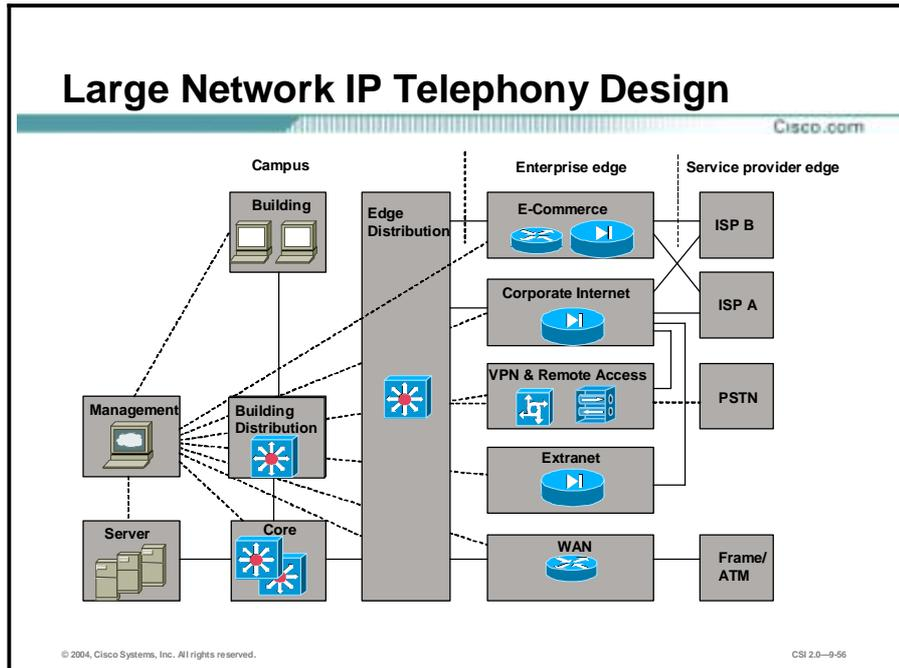
The large network IP telephony design uses the large network design from the SAFE: A security Blueprint for Enterprise Networks white paper. IP telephony is covered in the initial release of the paper but not discussed in depth. Some changes have been made to the design, including:
