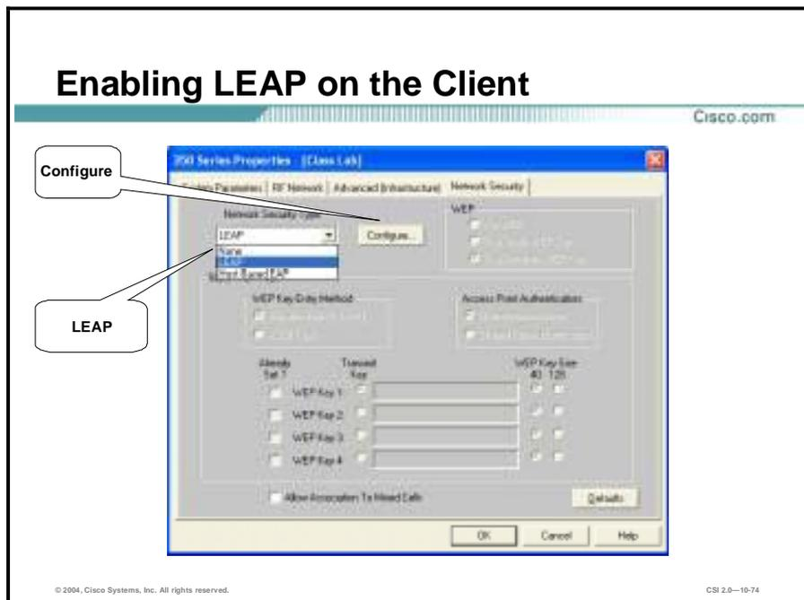
From the Profile Manager on ACU, choose the profile you wish to configure for Server Based Authentication, and click the **Edit** button. This will launch the Properties screens for the profile. Click the **Network Security** tab.
