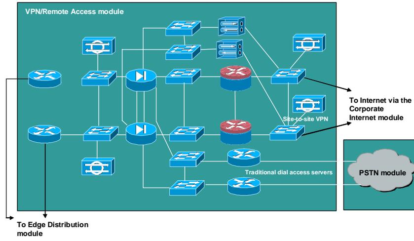
The primary objective of the VPN and Remote Access module is threefold: terminate the VPN traffic from remote users, provide a hub for terminating VPN traffic from remote sites, and terminate traditional dial-in users. All the traffic forwarded to the Edge Distribution module is from remote corporate users that are authenticated in some fashion before being allowed through the firewall.
