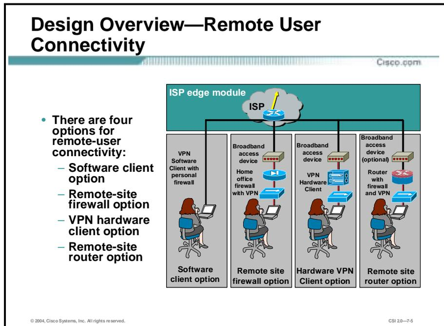
Remote connectivity applies to both mobile workers and home-office workers. The primary purpose of these designs is to provide connectivity from the remote site to the corporate headquarters and the Internet. The following four options include software-only, software-with-hardware, and hardware-only solutions:
