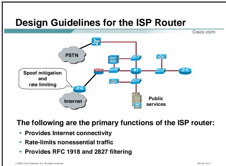
The primary function of the customer-edge router in the ISP (ISP router) is to provide connectivity to the Internet or ISP network. The egress of the ISP router rate-limits nonessential traffic that exceeds pre-specified thresholds in order to mitigate against distributed denial of service (DDoS) attacks. In addition, at the egress of the ISP router, RFC 1918 and RFC 2827 filtering is configured to mitigate against source-address spoofing of local networks and private address ranges.
