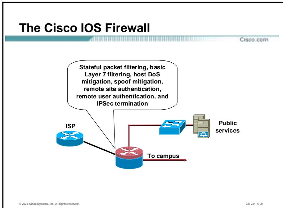
The primary function of the Cisco IOS Firewall is to provide connection-state enforcement and detailed filtering for sessions initiated through the Cisco IOS Firewall. The Cisco IOS Firewall also acts as a termination point for site-to-site IPSec VPN tunnels for both remote site production and remote site management traffic.
