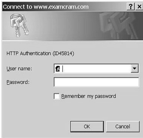
Figure 10.4 The cut-through proxy HTTP dialog box.
