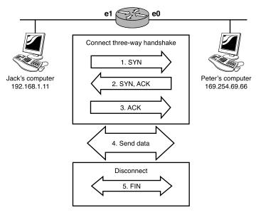
Figure 5.1 A three-way handshake.
