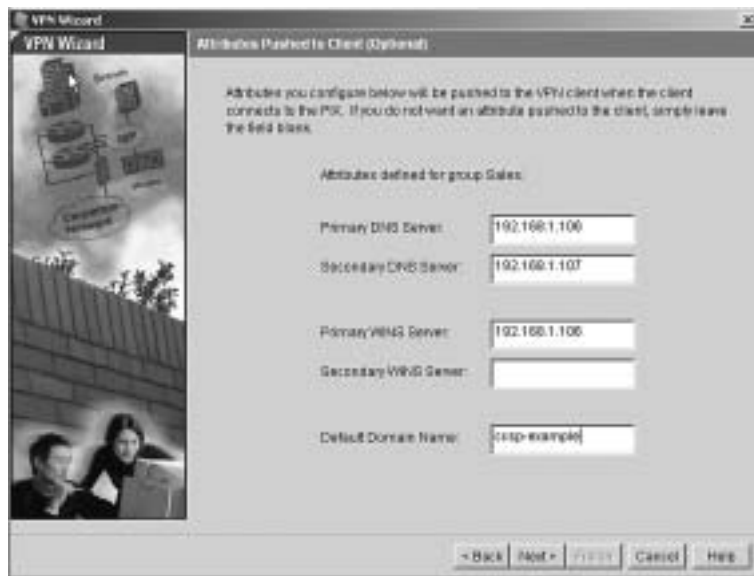
Figure 13-23 Attributes Pushed to Client Window
