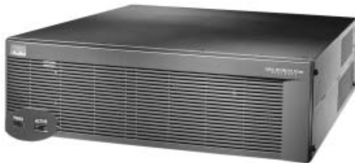
Figure 3-13 PIX 535 Front Panel
