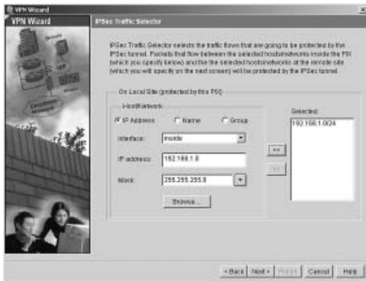
Figure 13-15 IPSec Traffic Selector Window: On Local Site
