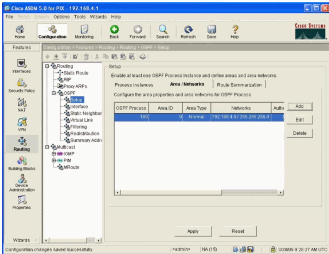
40. Enter the IP Address and Netmask of the second network in the OSPF process field and click **OK**.
