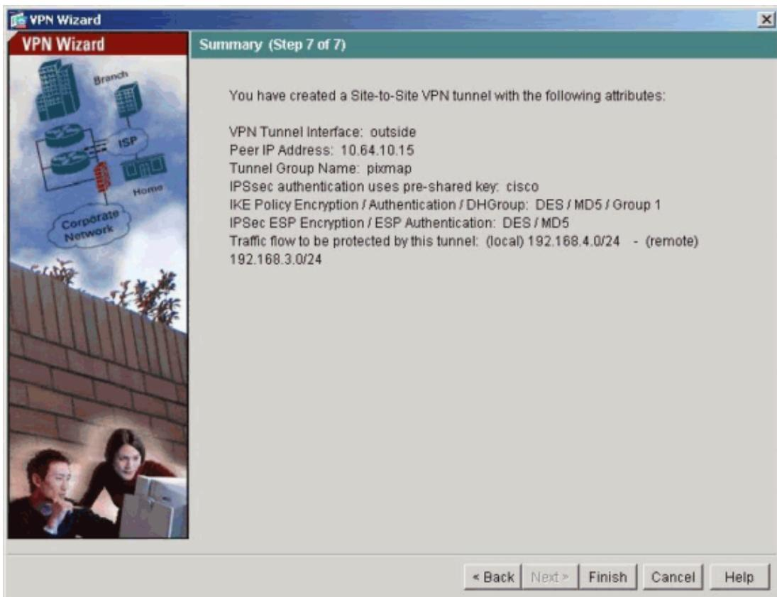
22. In order to verify the LAN-to-LAN tunnel configurations that the VPN Wizard created, choose **Configuration > VPN**.
