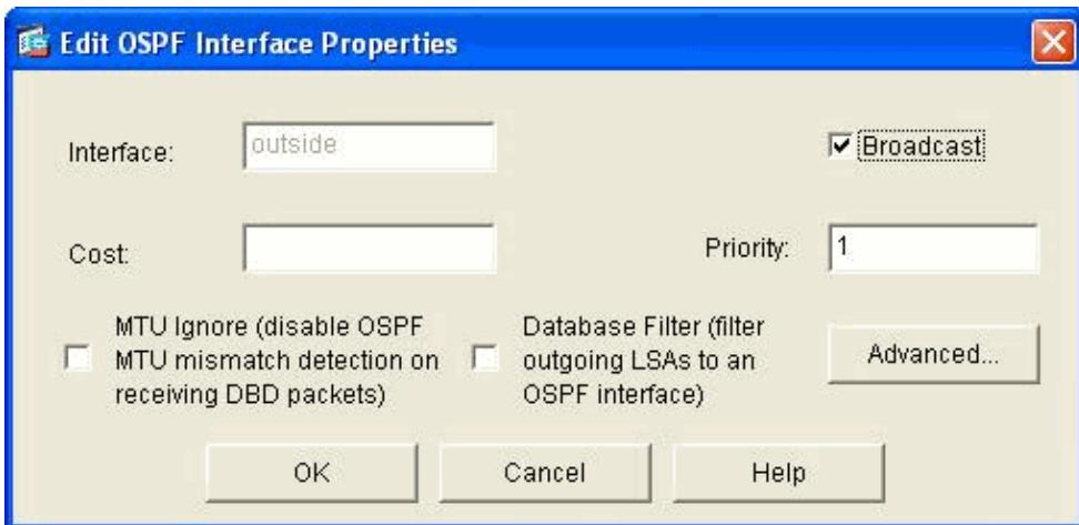
44. Check the Broadcast column for the outside interface in order to verify that the selection is **no**, then click **Apply**.
