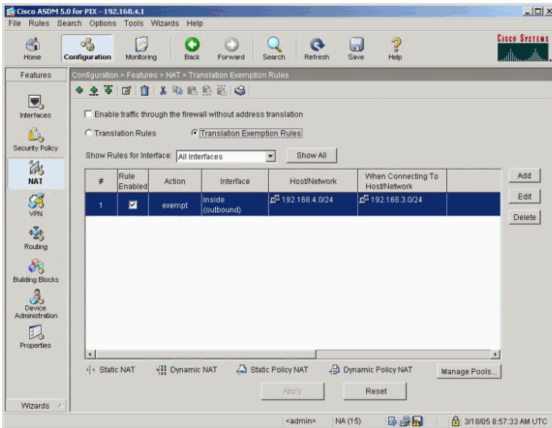
28. Because this example uses NAT, uncheck the check box for **Enable traffic through the firewall**
