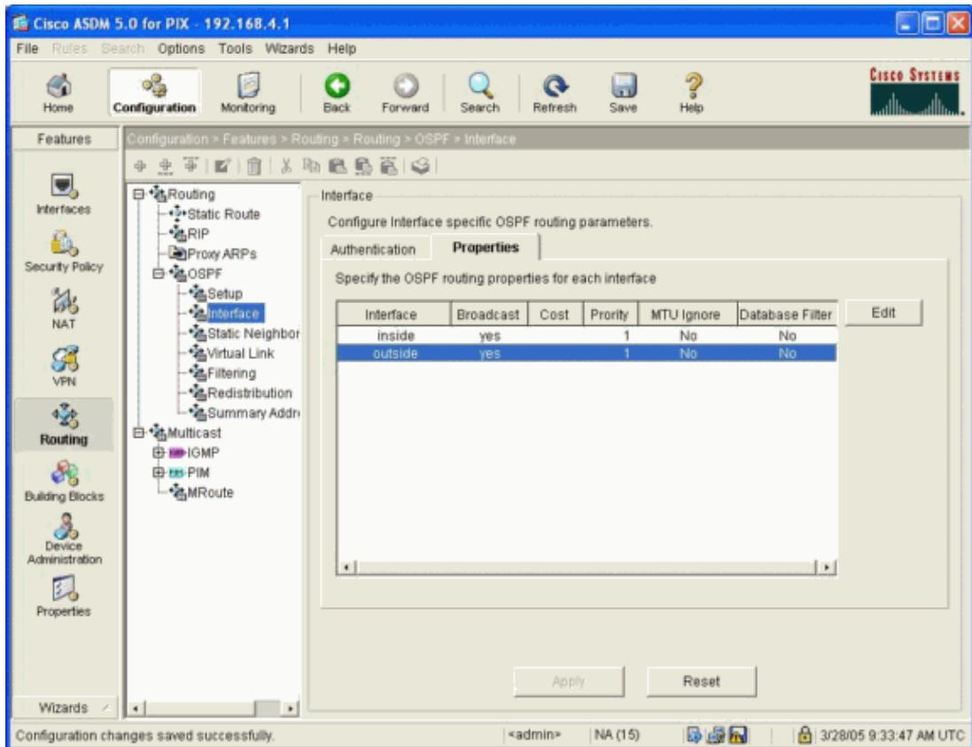
43. Uncheck the **Broadcast** check box on the outside interface.
