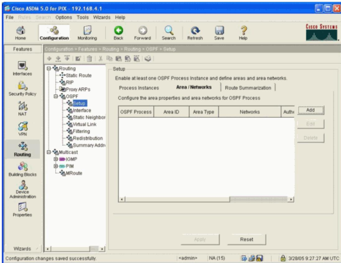
38. Enter the IP Address and Netmask of one network in the OSPF process field and click **OK**.
