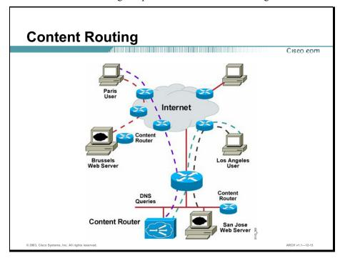
Cisco routers and switches incorporate Web Cache Communication Protocol (WCCP) software to enable content routing capabilities. Additionally, Cisco offers content routers specifically designed to support large-scale mirrored web sites.
