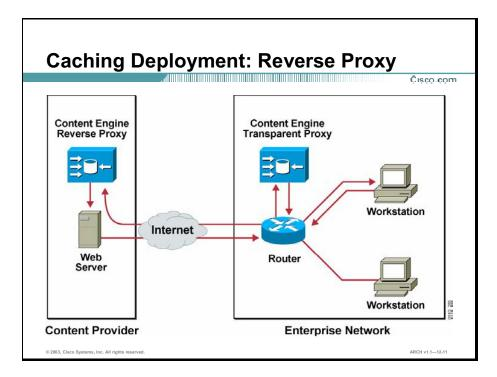
With reverse proxy caching, static content from a server is offloaded onto a CE. Requests destined for the server are directed to the CE, which serves the content locally, freeing the server from processing multiple requests for static content. CEs in reverse proxy mode are placed close to the servers being offloaded, typically in an internal server farm or an edge server farm providing outbound web or e-commerce services.
