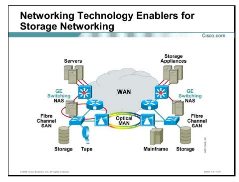
The iSCSI protocol enables access to storage over TCP/IP, while Fibre Channel over IP (FCIP) links Fibre Channel SANs over IP.
