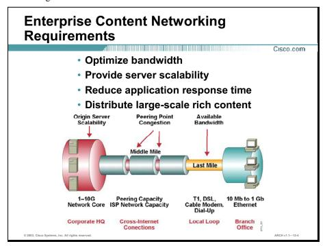
Users are accessing web content more and more frequently. In addition, the content being delivered continues to increase in size and complexity. With the increase in activity and content size, enterprises can experience bandwidth bottlenecks, overloaded servers, and degraded response times. New applications such as broadcast video and media-on-demand can place an untenable strain on network resources.
