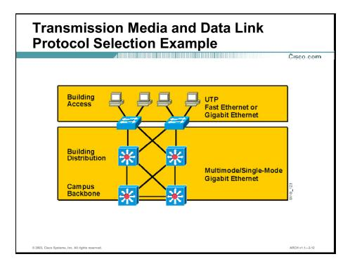
The figure shows the transmission media for a typical campus network structure. Building Access submodule devices that are no more than 100 meters away from the LAN switch use UTP. The UTP wiring can easily handle the required distance and speed and is easy to install.
