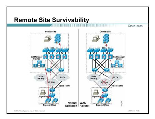
When deploying IP telephony across a WAN with the centralized call processing model, you should take additional steps to ensure that data and voice services at the remote sites are highly available. SRST provides high availability for voice services only, by providing a subset of the call processing capabilities within the remote office router and enhancing the IP Phones with the ability to "re-home" to the call processing functions in the local router if a WAN failure is detected.
