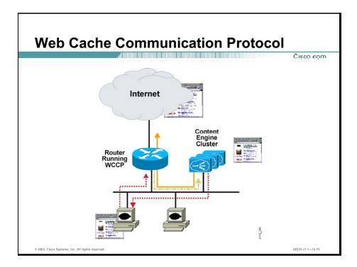
WCCP provides the mechanism for content routers and other WCCP-enabled routers and switches to redirect user requests to the appropriate destination. WCCP includes load balancing, scaling, fault tolerance, and service-assurance (failsafe) mechanisms, and includes these steps:
