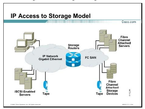
Cisco extends storage consolidation beyond the data center by enabling block-oriented storage I/O over an IP network. This allows servers that may not have otherwise been eligible to connect to shared storage resources. This could include Microsoft Windows server farms, remote servers, and small server clusters in remote offices.
