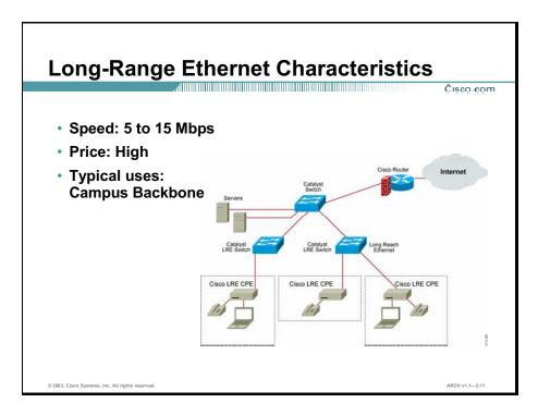
For buildings with existing Category 1/2/3 wiring, Long-Range Ethernet (LRE) technology provides connectivity at speeds from 5 to 15 Mbps (full duplex) and distances up to 5000 feet. LRE technology delivers broadband service on the same lines as plain old telephone service (POTS), digital telephone, and ISDN traffic. LRE also supports modes compatible with asymmetric digital subscriber lines (ADSLs), allowing enterprises to implement LRE to buildings where broadband services currently exist.
