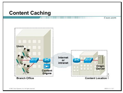
Caching is a demand-based replication and storage of cacheable content for the purpose of serving that same content to users making subsequent requests for it. Cacheable content is typically static application data associated with a file type and file extension, such as:
