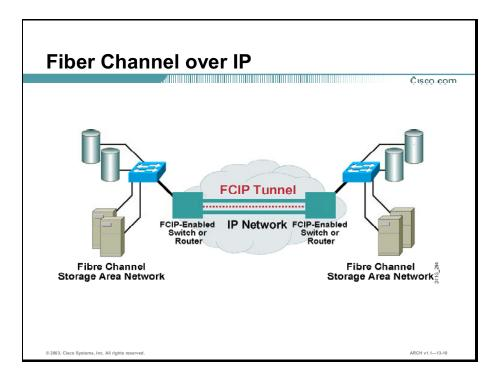
An important technology for linking Fibre Channel SANs is FCIP. FCIP and iSCSI are complementary solutions for enabling company-wide access to storage. FCIP transparently interconnects Fibre Channel SAN islands over IP networks through FCIP tunnels, while iSCSI allows IP-connected hosts to access iSCSI or FC-connected storage.
