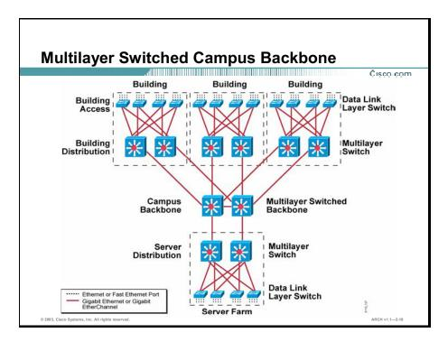
The most flexible and scalable campus backbone consists of multilayer switches, as shown in the figure. The backbone switches are connected by routed Gigabit Ethernet or Gigabit EtherChannel links. Multilayer-switched backbones have several advantages:
