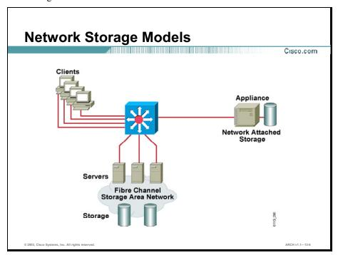
A SAN describes a dedicated, high-performance network infrastructure deployed between servers and storage resources. The storage area infrastructure is a separate, dedicated network entity optimized for the efficient movement of a large amount of raw block data to the application servers, which coordinate client access to data. In effect, SAN is an extended link between server and storage. SANs enable the extension of the storage access protocol over longer distances.
