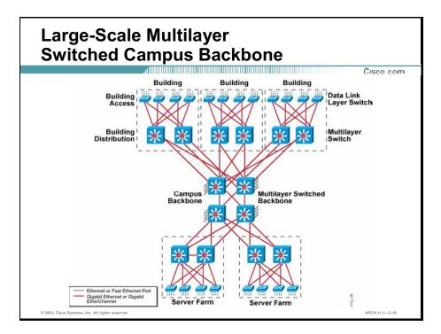
The figure shows the multilayer-switched campus backbone on a large scale. The multilayer-switched backbone has the advantage that arbitrary topologies are supported because a sophisticated routing protocol such as EIGRP or OSPF is used pervasively.
