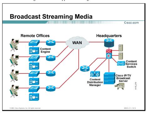
Applications such as e-learning and corporate communications frequently involve broadcasting media streams that are to be accessed simultaneously by multiple users throughout the network. The content networking solution shown in the figure includes these components:
