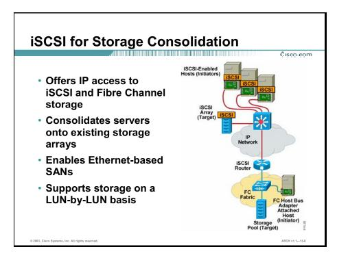
The iSCSI protocol encapsulates a SCSI request in an IP packet. iSCSI is a SCSI transport protocol for mapping block-oriented storage requests over TCP/IP networks. Making direct access to storage over IP possible, the iSCSI protocol allows IP-connected hosts to access iSCSI or Fibre Channel-connected storage.
