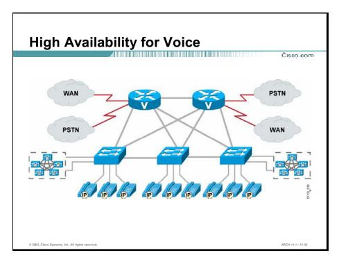
Cisco AVVID IP telephony is based on a distributed model for high availability. CallManager clusters support CallManager redundancy. The gateways must support the ability to "re-home" to a secondary CallManager in the event that a primary CallManager fails, providing CallManager redundancy. This differs from call survivability in the event of a CallManager or network failure, where the call is routed to an alternate gateway, such as an MGCP gateway.
