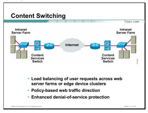
Content switching intelligently load balances traffic across servers or CEs based on the availability of the content and the load on the server. Content Services Switches (CSSs) provide these services:
