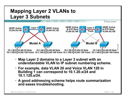
In a structured design, one IP subnet maps to a single VLAN, which is carried to the wiring-closet switch. A good IP addressing scheme can take advantage of multilayer switching features to exchange summarized routing information, rather than learning the path to every host in the whole network. Summarization is important to routing protocol scalability for OSPF and EIGRP.
