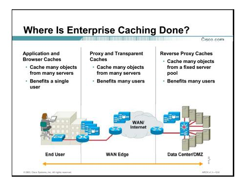
Enterprise caching can be accomplished between a central site and any remote site. At the central site, caching is deployed at the data center or within a perimeter LAN. Typically, caching takes place at the remote site, close to users.
