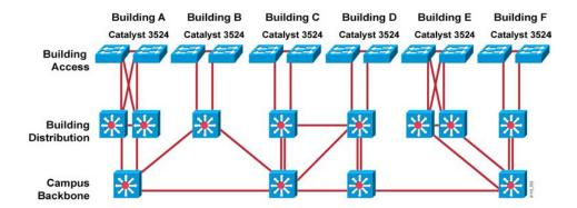
The figure shows a network diagram for the wide area network with redundant links for load sharing and high availability.
