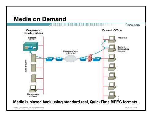
A media-on-demand solution typically involves the distribution of large video and/or audio files. The content networking solution shown in the figure includes these components:
