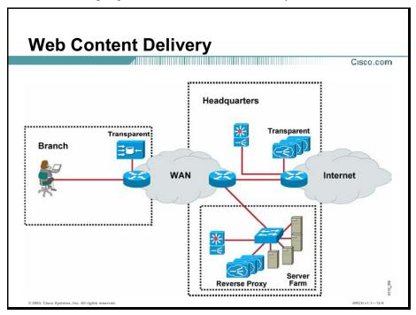
A content networking implementation for web delivery should take into account access to both internal and external web servers from throughout the enterprise. The example implementation shown in the figure includes these elements:
