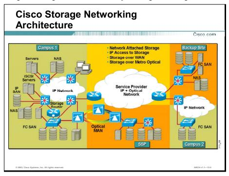
Key components of the Cisco storage networking solution are:
