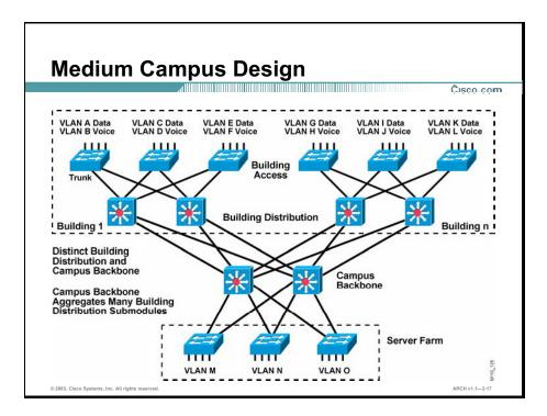
A medium campus design with higher availability and higher capacity is shown in the figure. The most flexible and scalable campus backbone consists of multilayer switches, as shown in the figure. The backbone switches are connected by routed Gigabit Ethernet or Gigabit EtherChannel links. Multilayer-switched backbones offer these advantages:
