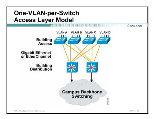
The Building Access submodule is the first point of entry into the network and essentially links end users to the remainder of the network. The figure shows a one-VLAN-per-switch Building Access submodule model.
