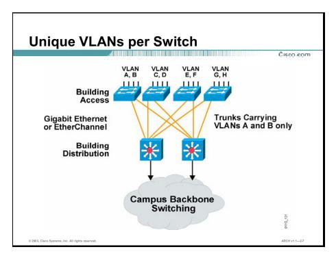
The figure represents a set of unique VLANs per switch. Because more than one VLAN exists per wiring-closet switch, trunks are defined and unnecessary VLANs are removed. This design still requires a multilayer device to transport traffic between VLANs.
