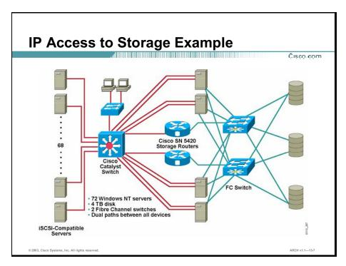
A major medical research facility's database was growing quickly, and users needed access. Hundreds of users in five separate buildings were networked into a powerful server farm made up of application servers that shared a very large, 4-terabyte Oracle database. The organization wanted to install a storage network to support the storage access requirements at the remote locations that would support their performance and cost needs, as well as grow with them in the future.
