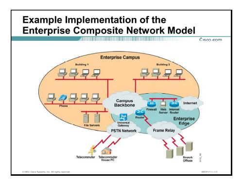
The figure shows an enterprise network with the major components of the Enterprise Composite Network Model. The network is divided into the Enterprise Campus and Enterprise Edge functional areas, connected by the Campus Backbone submodule.
