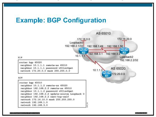
The figure above shows another BGP example, which will take into account several BGP features and conclude the topic of configuring basic BGP configuration steps. Router R1 has one EBGP neighbor, router R2 has one EBGP and one IBGP neighbor, and router R3 has one IBGP neighbor. Showing the configuration of routers R1 and R2 will explain the basic configuration needed to create an EBGP and IBGP neighbor relationship.
