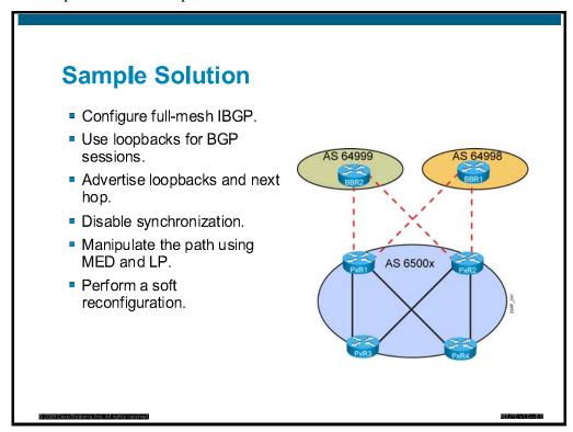
This sample solution includes the configuration steps necessary for each of the tasks. Different solutions are possible. However, this figure points out the important tasks required for successful configuration.
