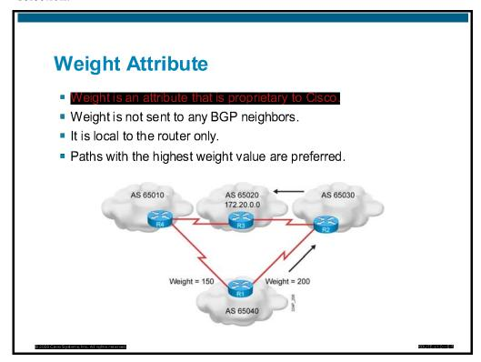
The weight attribute is an attribute that Cisco defines for the path selection process. The weight is configured locally on a router and is not propagated to any other routers. This attribute applies when one router is used with multiple exit points out of an autonomous system, as opposed to the local preference attribute, which is used when two or more routers provide multiple exit points.
