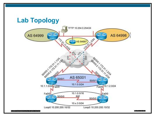
This figure presents the lab topology used for the configuration of BGP path manipulation lab. The topology uses four pod routers, which are members of a full Internal BGP (IBGP) relationship and two backbone routers, which are members of an External BGP (EBGP) relationship. The lab is preconfigured with addressing including loopbacks and an IGP routing protocol.
