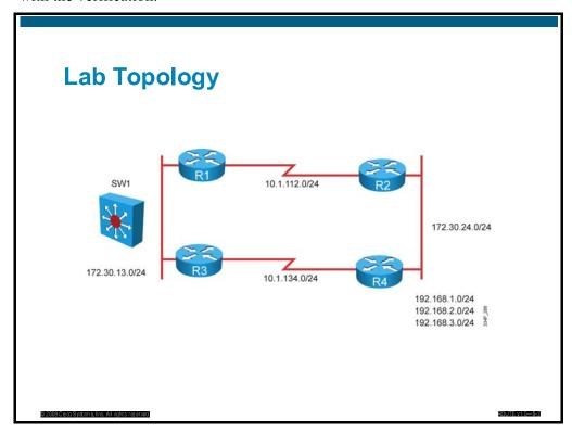
This figure shows the physical lab topology used for Lab 5-1: Configure and verify Path Control between multiple IP routing protocols. The topology uses four pod routers and one switch. Routers R1 to R4 build the network where path manipulation is required, and switch SW1 is one source of packets. The other source is locally-originated traffic on router R1.
