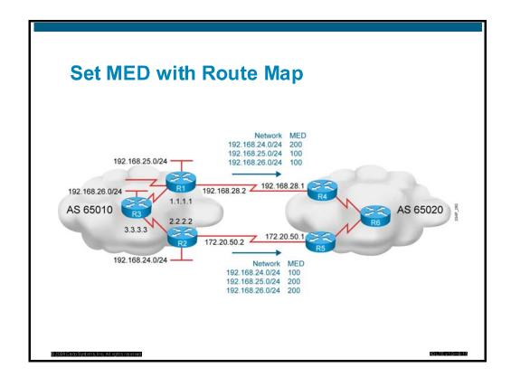
This figure is used in the following configurations to demonstrate how to manipulate inbound traffic using route maps to change the BGP MED attribute. The intention of these route maps is to designate router R1 as the preferred path to reach networks 192.168.25.0/24 and 192.168.26.0/24 and to designate router R2 as the preferred path to reach network 192.168.24.0/24. The other networks should still be reachable through each router in case of a link or router failure.
