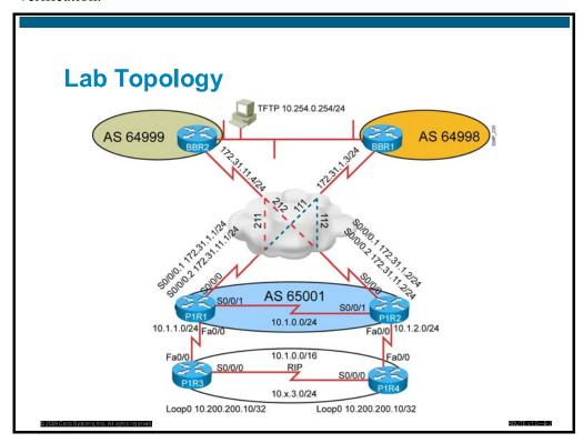
The figure above presents a logical lab topology used for configuration of a BGP operations lab. The topology uses four pod routers, which are members of an Internal BGP (IBGP) relationship, and two backbone routers, which are members of an EBGP relationship. The lab is preconfigured with addressing, including loopbacks and an IGP routing protocol.
