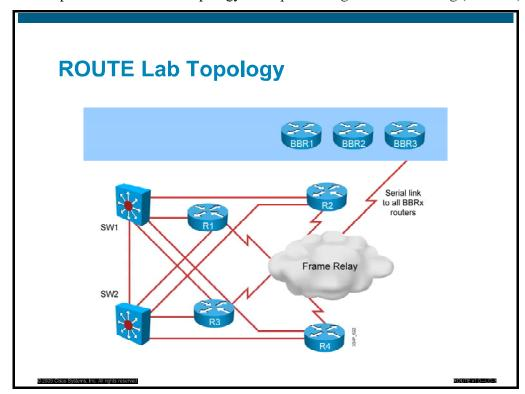
The ROUTE v1.0 lab topology consists of a student pod that represents an enterprise network. The student pod is connected to a backbone managed by the instructor, which represents the Internet. The student pod consists of four routers and two multilayer switches. The instructor-managed backbone consists of three routers, a Layer 2 LAN switch, and a Frame Relay switch. All student pods are independent and use exactly the same IP address scheme and configurations.
